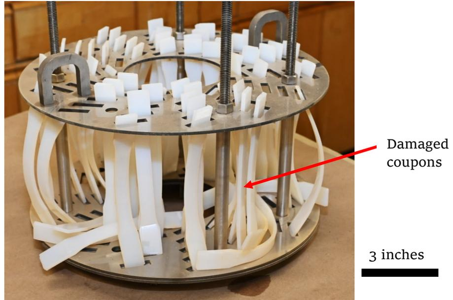
Figure 35: Carousel of damaged tensile test coupons
