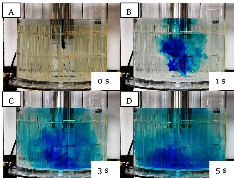
Figure 57: Dye test on skeletonized middle plate with sous vide heater only: (A) time at 0s, (B) time at 1s, (C) time at 3s, and (D) time at 5s
