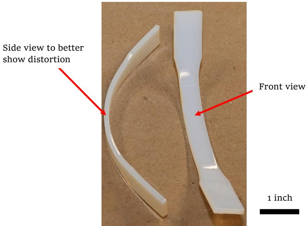
Figure 36: Close up view of damaged tensile test coupons showing the deformation
