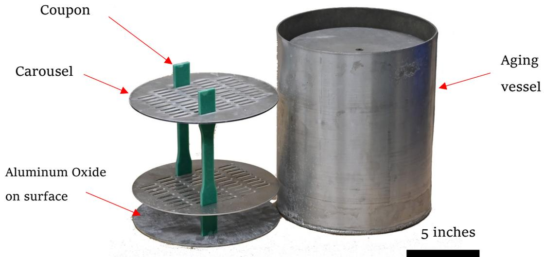
Figure 2: Previous tensile test coupon aging setup A
