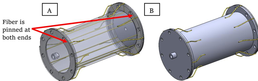
Figure 10: Design B concept of a fiber aging fixture: (A) transparent pipe spool to show fibers, (B) opaque pipe spool
