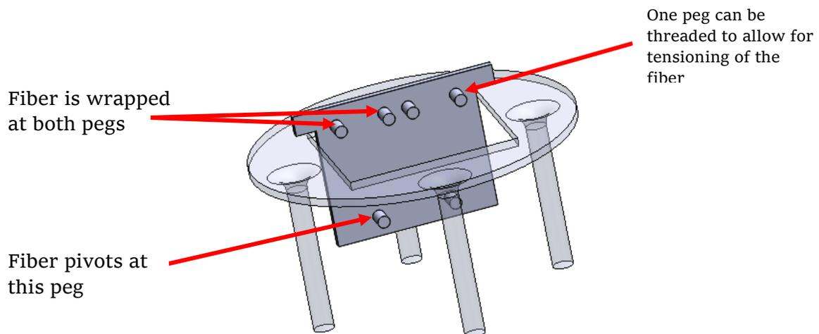
Figure 12: Design D concept of a fiber aging fixture with stand
