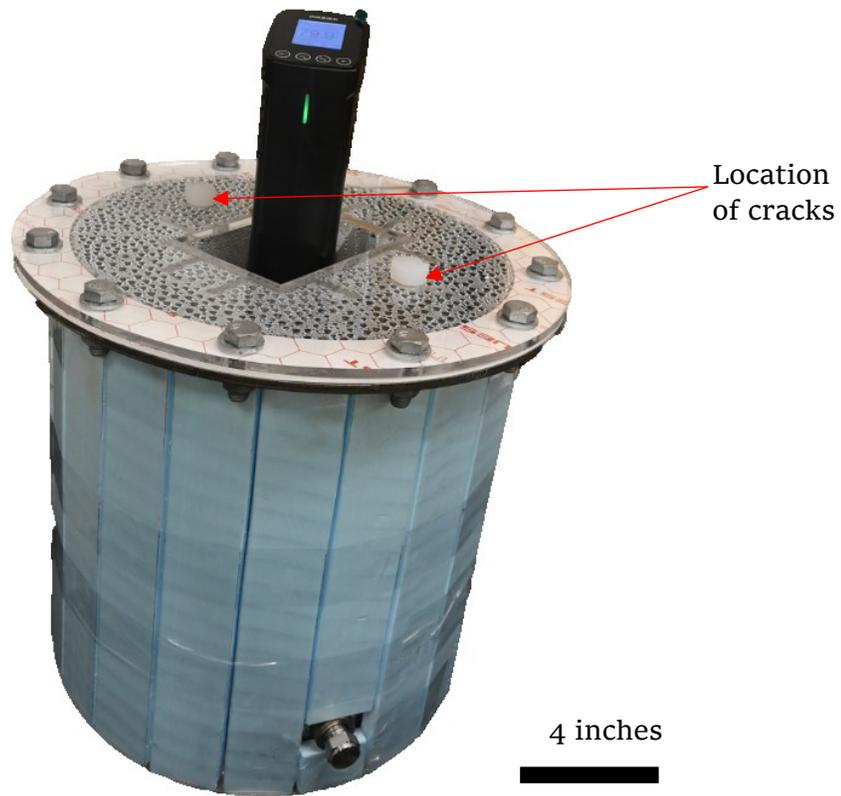
Figure 8: Location of cracks on aging cell from initial testing
