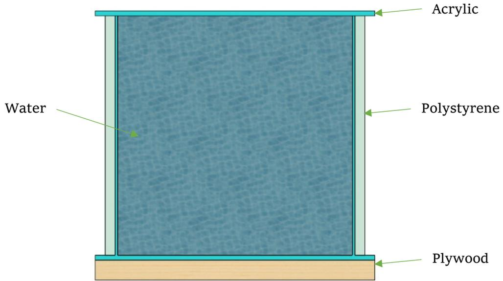
Figure 45: Cross section of aging cell for heat loss calculation
