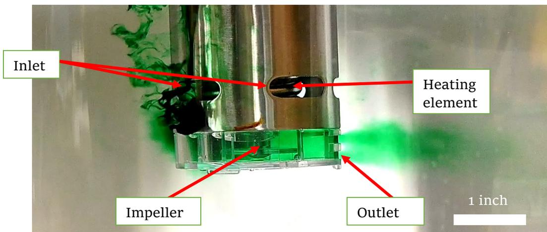
Figure 30: Sous vide heater with dye showing the flow path
