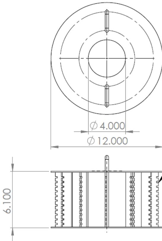
fibers are wound around the carousel with each fiber within a set of these slits
