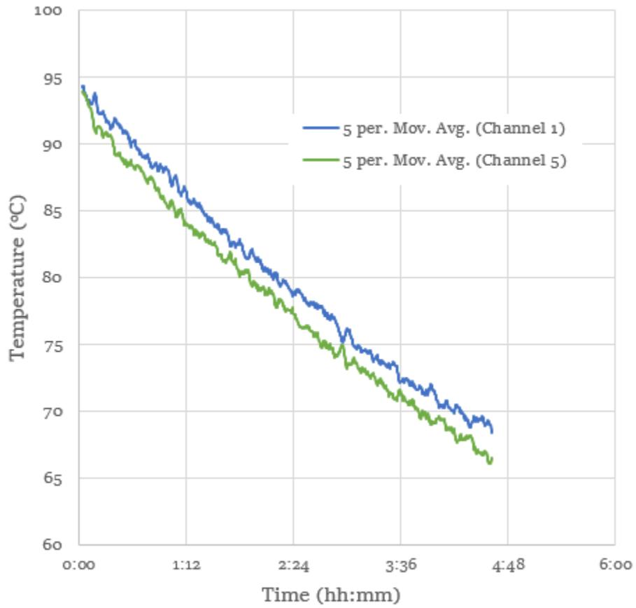
Figure 50: Stainless steel aging cell cool down curve at 95°C
