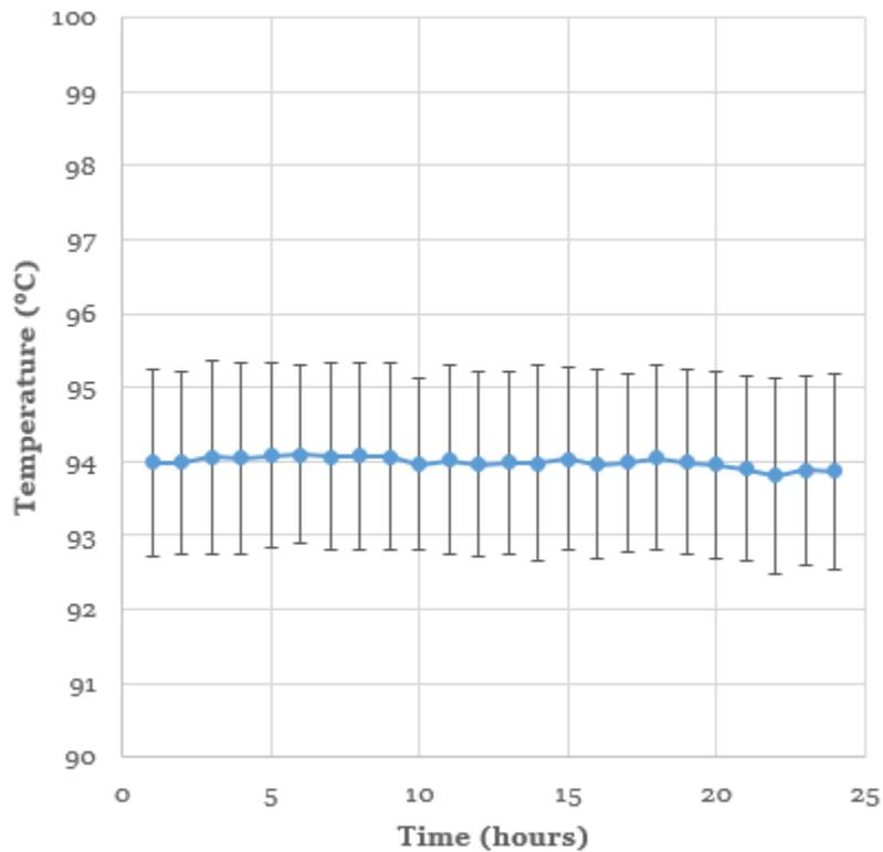
Figure 81: Stainless steel aging cell measured thermal gradients over 24 hours at 95.0°C
