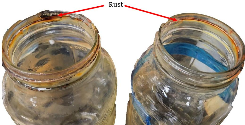
Figure 40: Rust on mason jars after 2 weeks of aging
