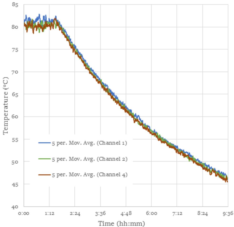
Figure 49: Stainless steel aging cell cool down curve at 82°C
