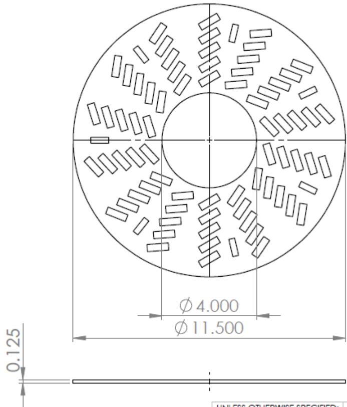
Made of 316SS perforated plate
