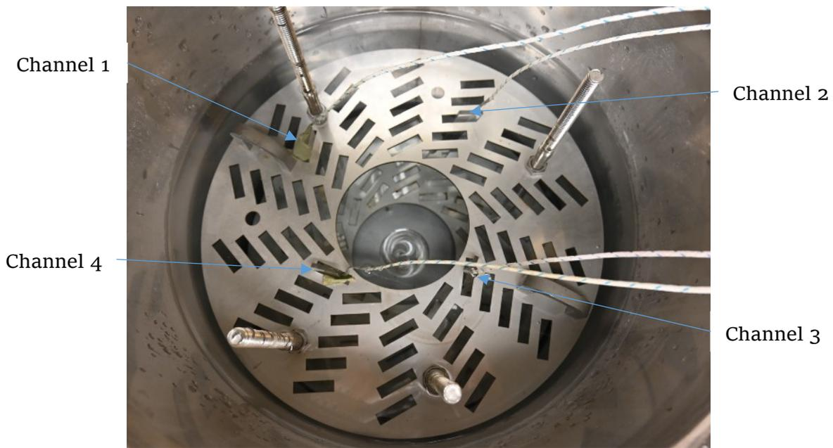
Figure 48: Thermocouple placement in the 82°C test
