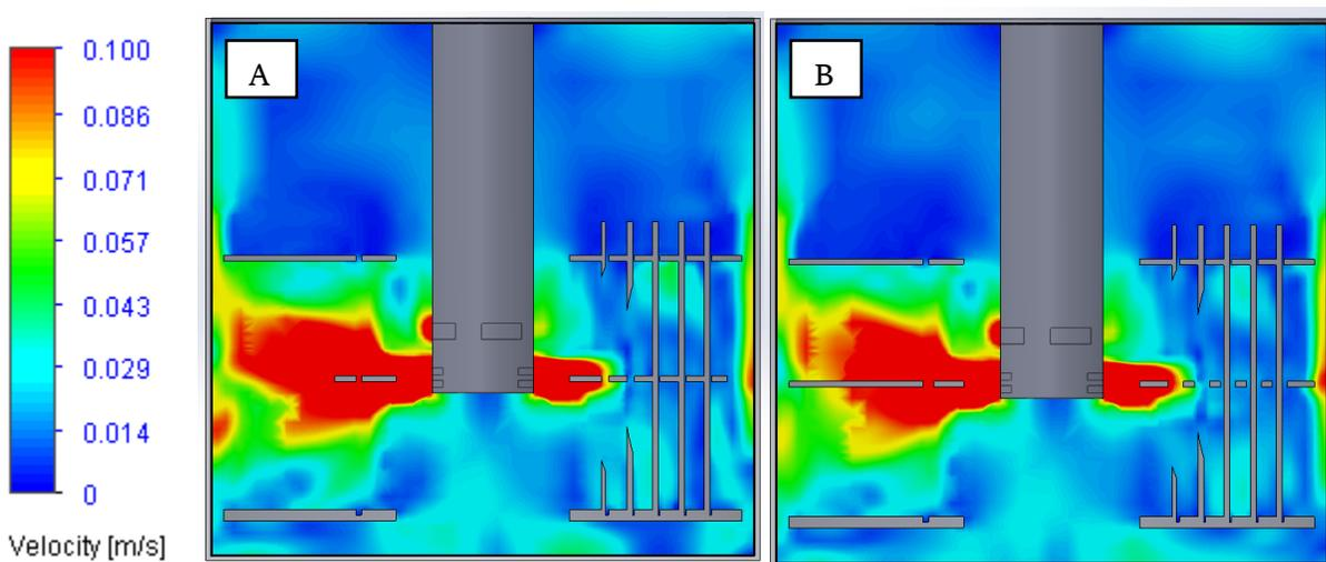
Figure 71: Vertical cross section of velocity profile with: (A) skeletonized middle plate, (B) full middle plate
