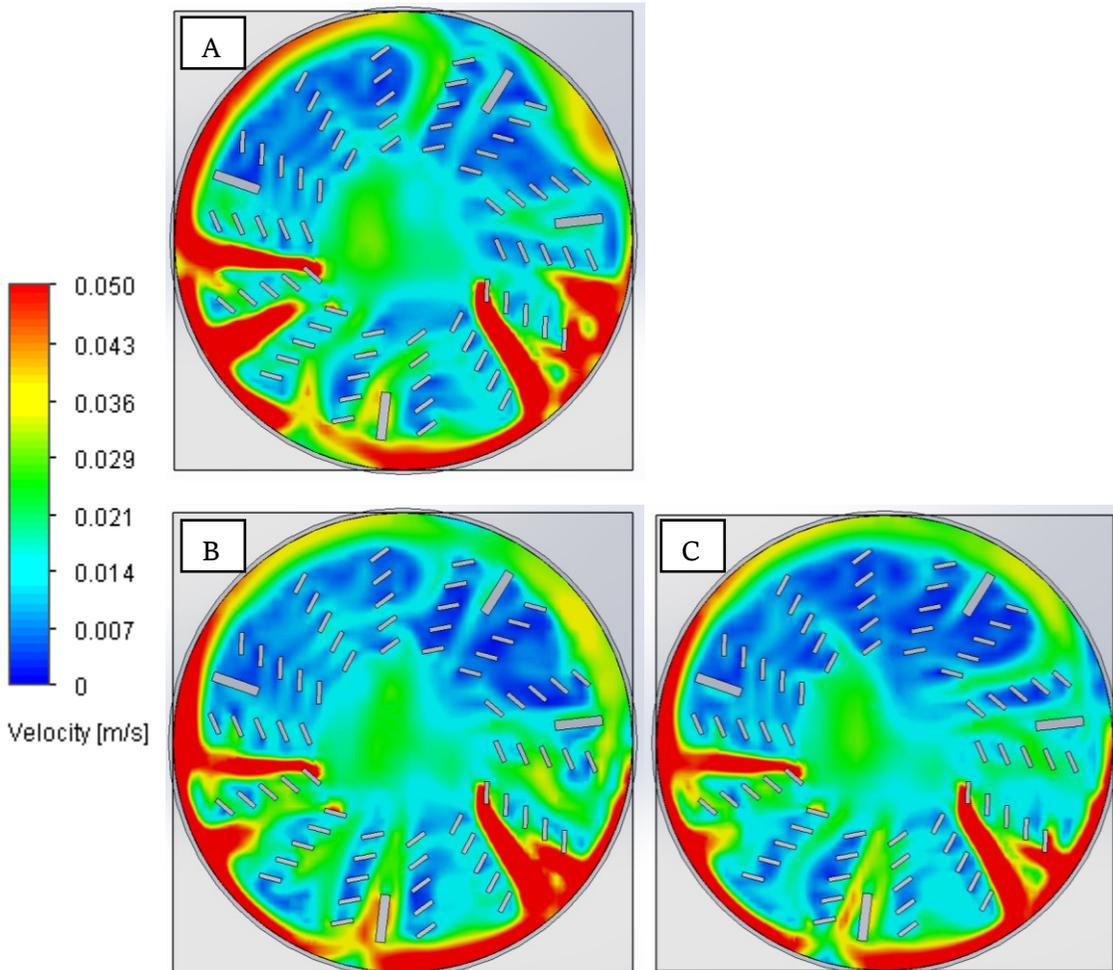
Figure 72: Horizontal cross section of velocity profile for: (A) perforated middle plate, (B) skeletonized middle plate, (C) full middle plate
