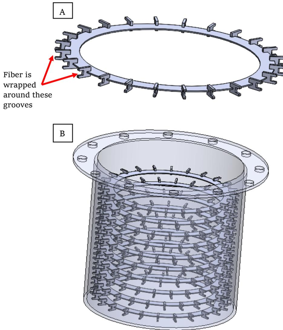
Figure 17: (A) Design I concept of a fiber aging fixture, (B) Design I fiber aging fixtures stacked inside of aging cell
