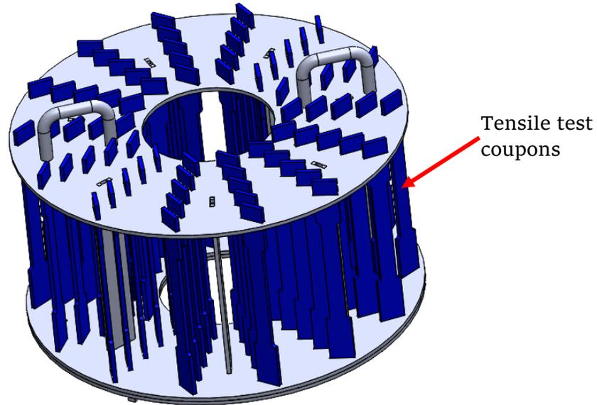
Figure 20: Carousel with tensile test coupons
