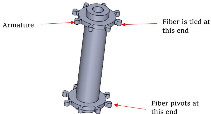
Figure 9: Design A concept of a fiber aging fixture
