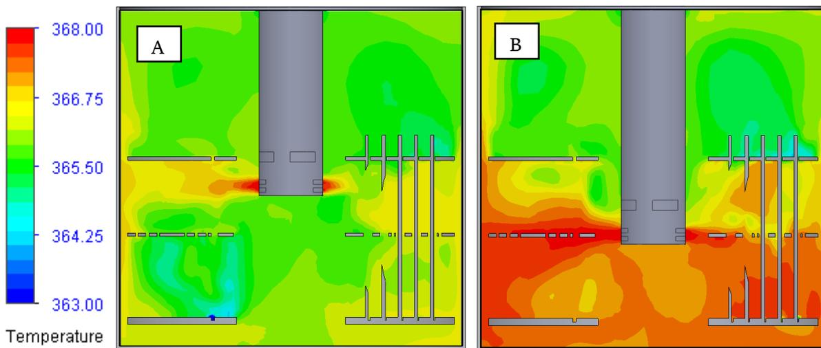
Figure 70: Vertical cross section of temperature profile with the perforated middle plate: (A) raised case, (B) centered case
