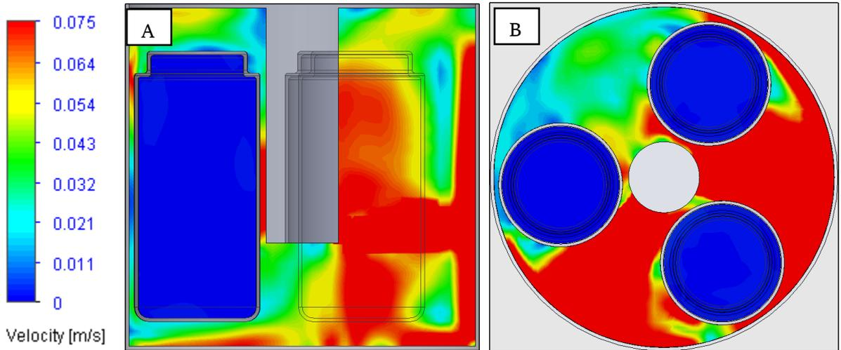
Figure 74: Cross section of velocity profile for the three jar case: (A) Front cross section, (B) horizontal cross section at the sous vide outlet
