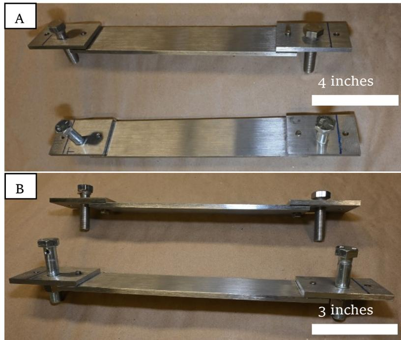
Figure 42: Design G fiber aging fixtures: (A) top view of fixtures, (B) side view of fixtures
