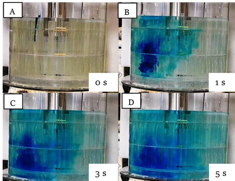
Figure 58: Dye test on perforated middle plate with sous vide heater only:
