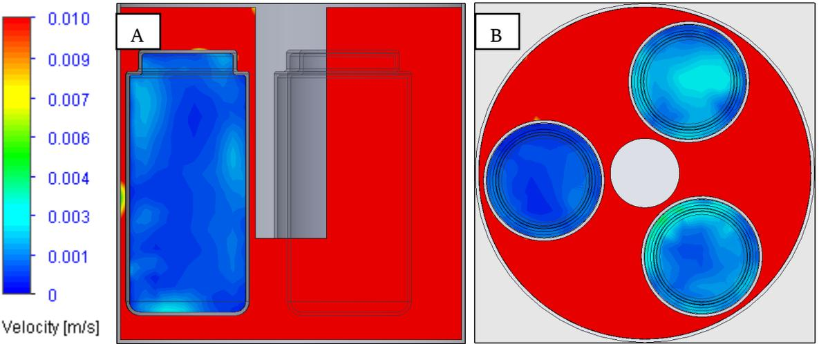
Figure 75: Cross section of velocity profile for the three jar case: (A) Front cross section, (B) horizontal cross section at the sous vide outlet
