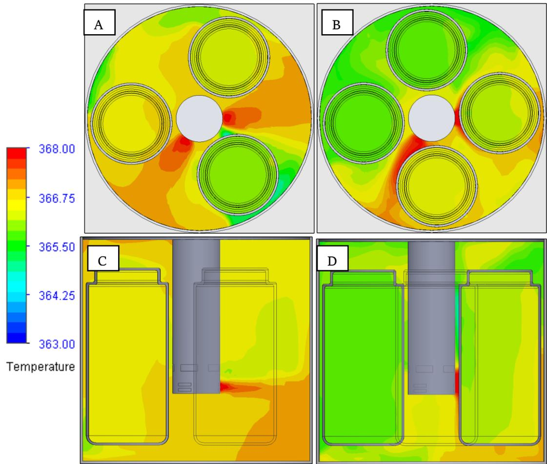
Figure 78: Cross section of temperature profile for the: (A) horizontal for the three jar case, (B) horizontal for the four jar case, (C) vertical for the three jar case, (D) vertical for the four jar case
