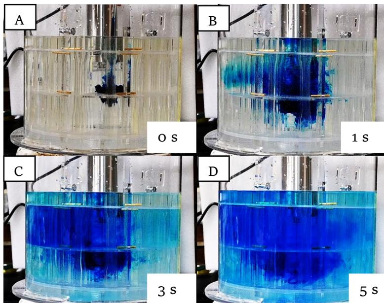
Figure 54: Dye test on modified carousel design with both magnetic stirring and sous vide heater on: (A) time at 0s, (B) time at 1s, (C) time at 3s, and (D) time at 5s
