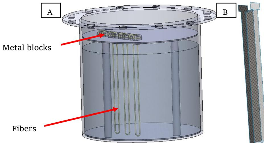
Figure 16: (A) Design H concept of a fiber aging fixture inside of aging cell, (B) mesh divider concept
