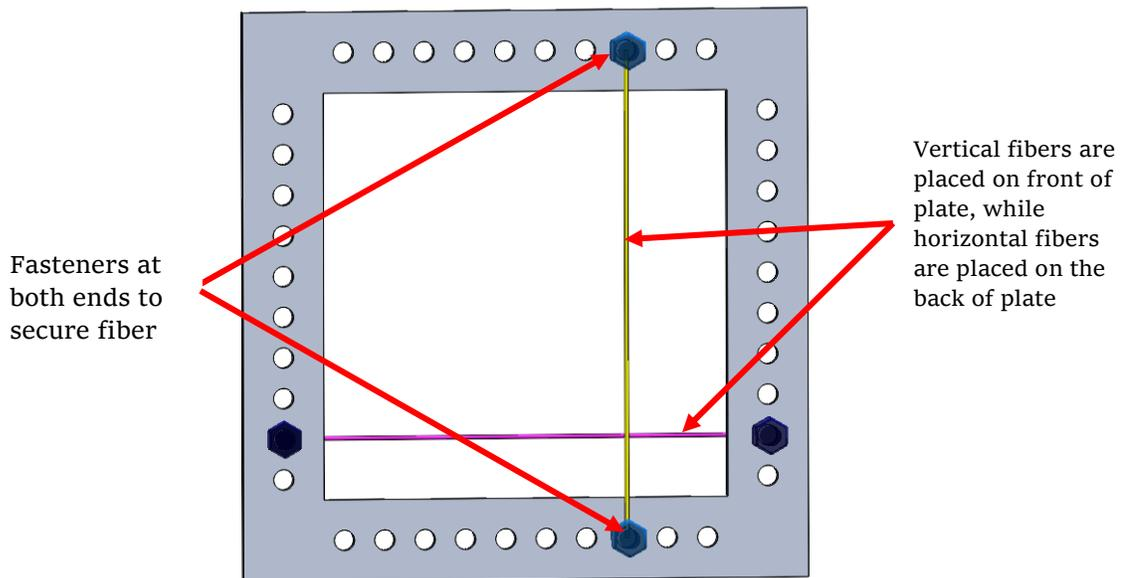
Figure 13: Design E concept of a fiber aging fixture
