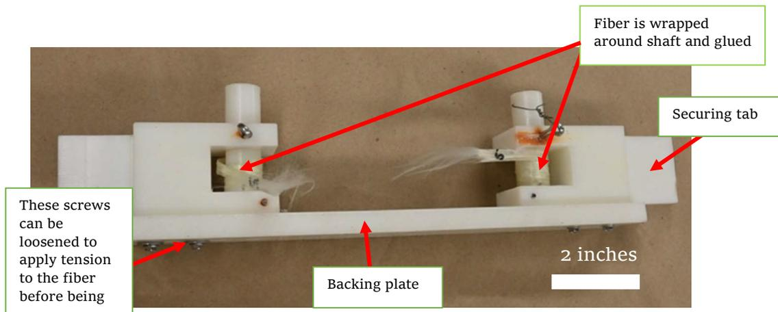
Figure 5: Fiber aging fixture (setup C) from another research group
