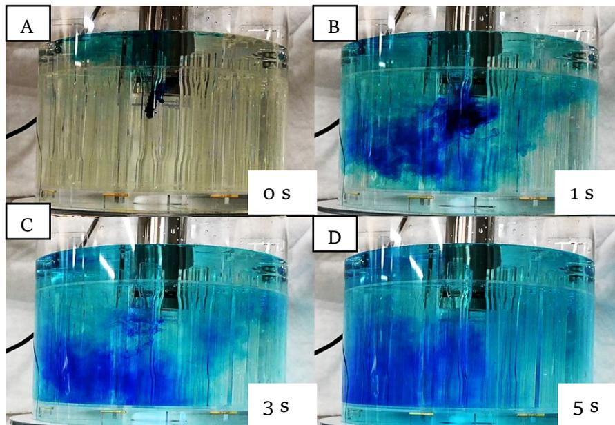
Figure 51: Dye test on initial carousel design with both magnetic stirring and sous vide heater on: (A) time at 0s, (B) time at 1s, (C) time at 3s, and (D) time at 5s
