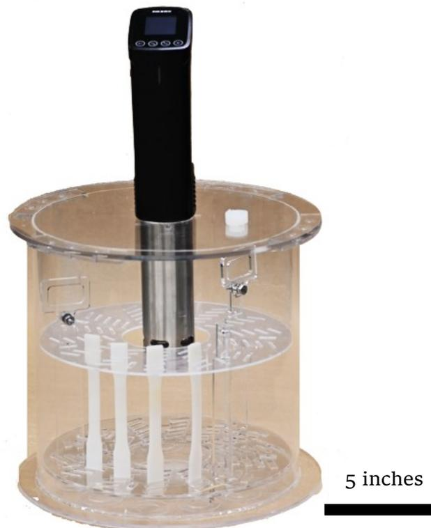
Figure 26: Acrylic aging cell and carousel with sous vide heater
