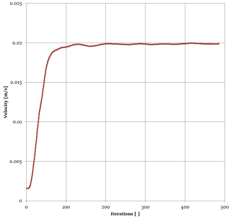
Figure 64: Velocity convergence plot for the lowered sous vide heater case
