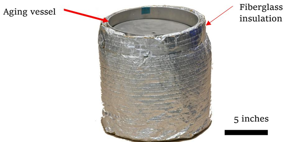
Figure 3: Previous tensile test coupon aging vessel (setup A) with insulation
