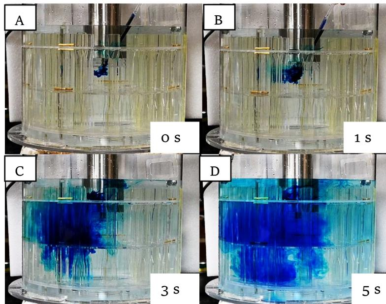
Figure 56: Dye test on modified carousel design with sous vide heater only: (A) time at 0s, (B) time at 1s, (C) time at 3s, and (D) time at 5s
