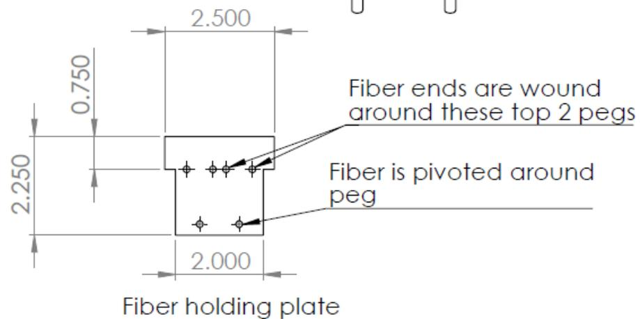
Note: model was scaled for 3D printing as a small palm sized concept model
