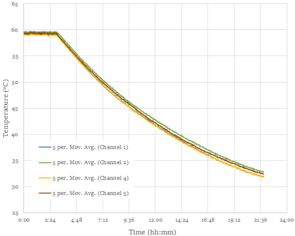
Figure 47: Acrylic aging cell cool down curve at 60°C
