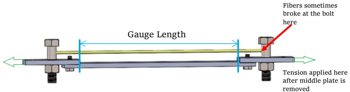
Figure 41: Design G fiber aging fixture location of breakage during initial testing
