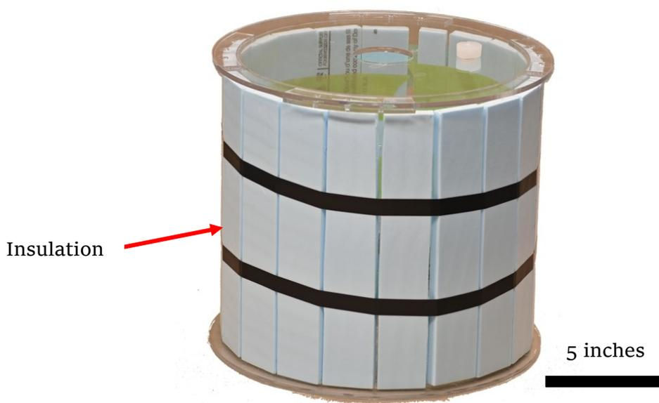
Figure 25: Acrylic aging cell with insulation
