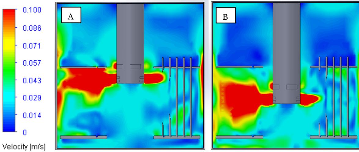
Figure 67: Vertical cross section of velocity profile with no middle plate: (A) raised case, (B) centered case
