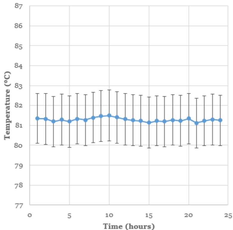
Figure 80: Stainless steel aging cell measured thermal gradients over 24 hours at 82.0°C
