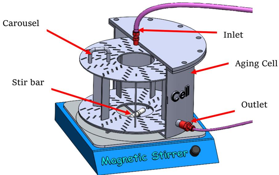
Figure 22: Close up view of aging cell showing carousel
