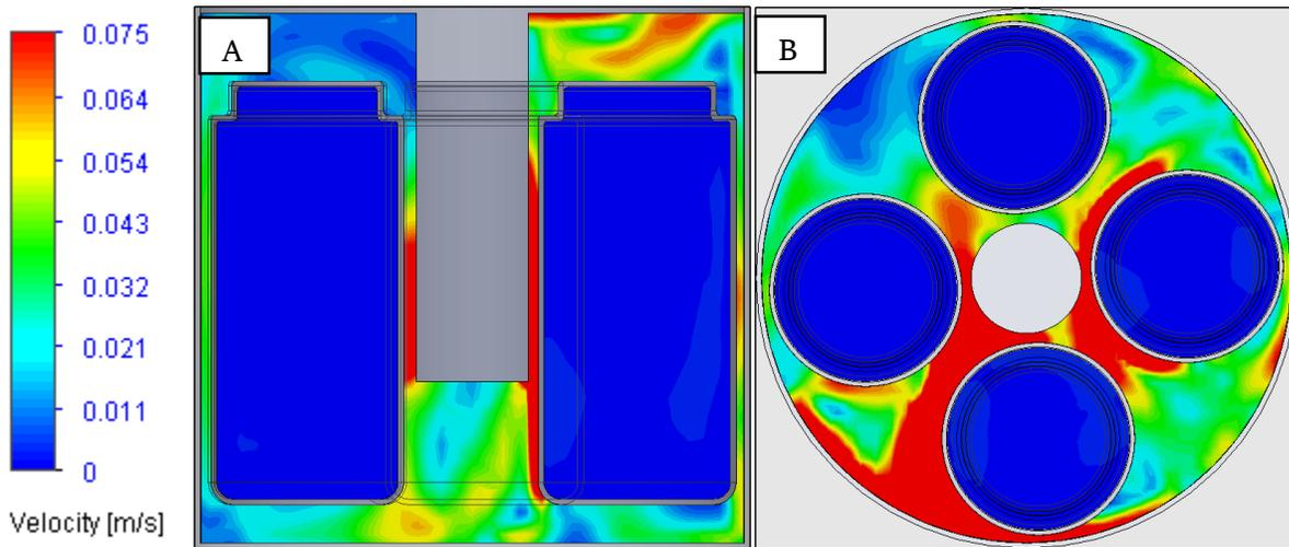
Figure 76: Cross section of velocity profile for the four jar case: (A) Front cross section, (B) horizontal cross section at the sous vide outlet
