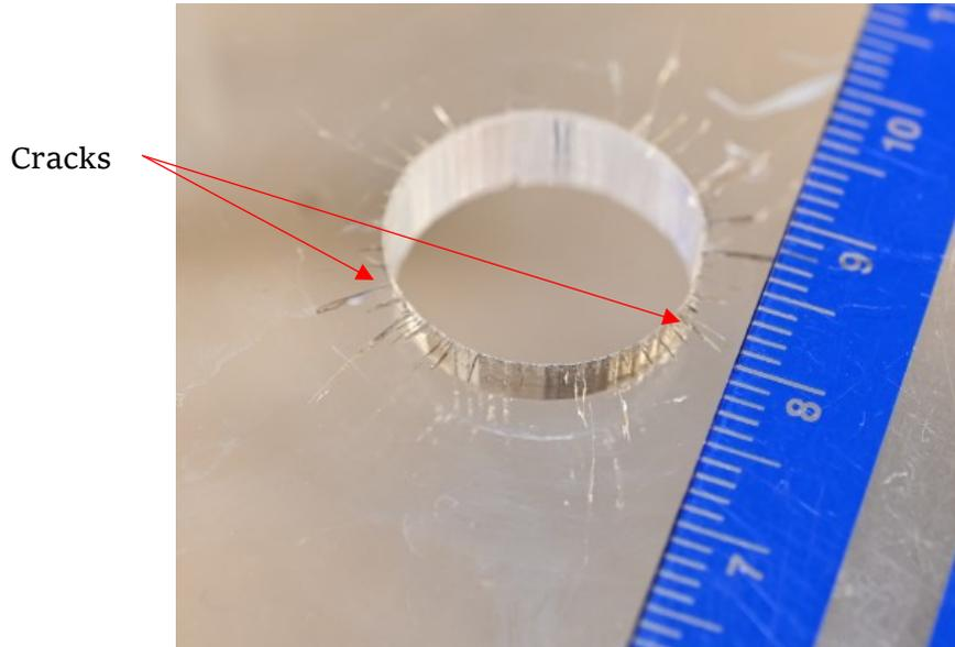
Figure 7: Cracks in acrylic around heat affected zone after exposure high temperatures and water
