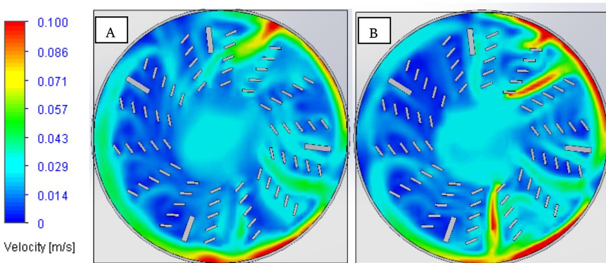
Figure 68: Horizontal cross section of velocity profile for the: (A) raised case, (B) centered case
