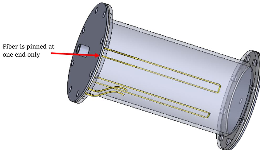
Figure 11: Design C concept of a fiber aging fixture
