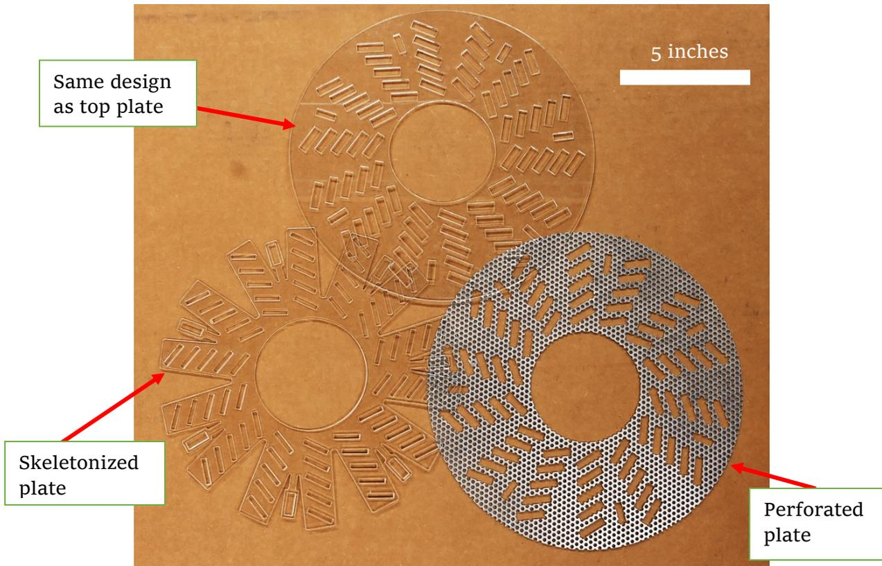
Figure 39: Various middle plate designs for the carousel
