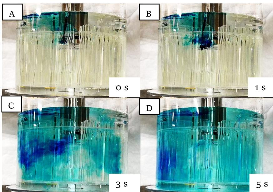
Figure 53: Dye test on initial carousel design with sous vide heater only: (A) time at 0s, (B) time at 1s, (C) time at 3s, and (D) time at 5s
