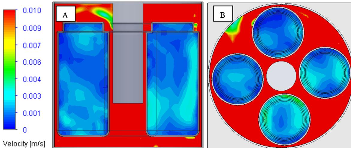
Figure 77: Cross section of velocity profile for the four jar case: (A) Front cross section, (B) horizontal cross section at the sous vide outlet
