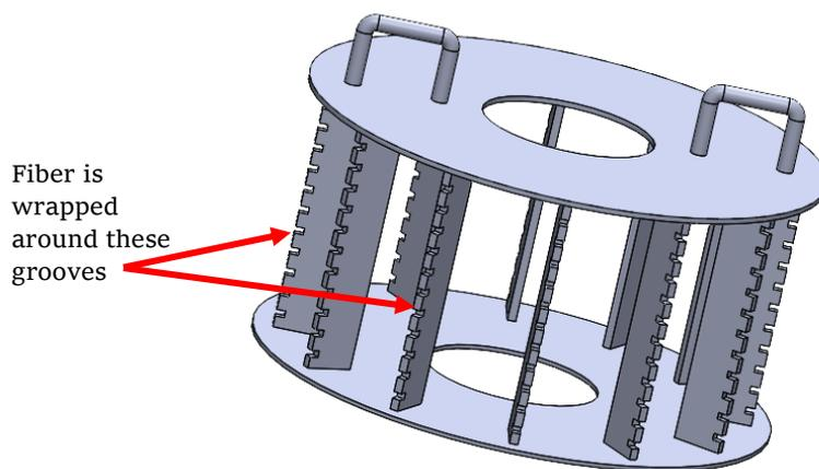
Figure 19: Design K concept of a fiber aging fixture
