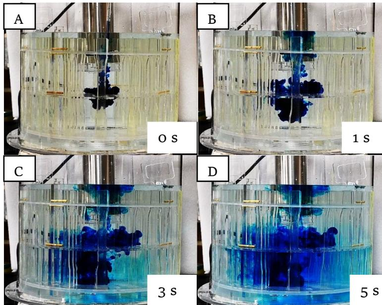
Figure 55: Dye test on modified carousel design with magnetic stirring only: (A) time at 0s, (B) time at 1s, (C) time at 3s, and (D) time at 5s
