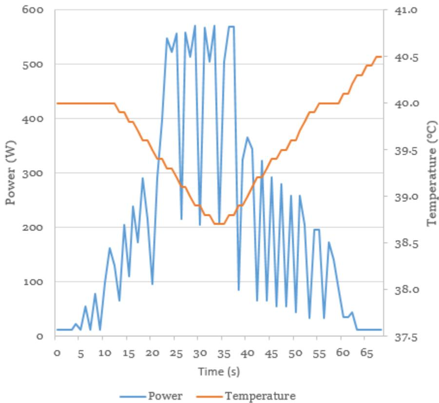
Figure 31: Sous vide heater power consumption to counteract a temperature change
