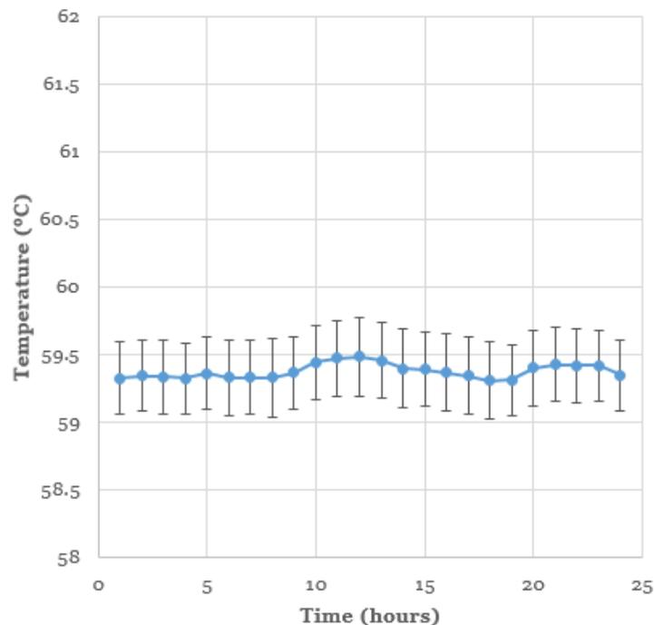
Figure 79: Acrylic aging cell measured thermal gradients over 24 hours at 60.0°C
