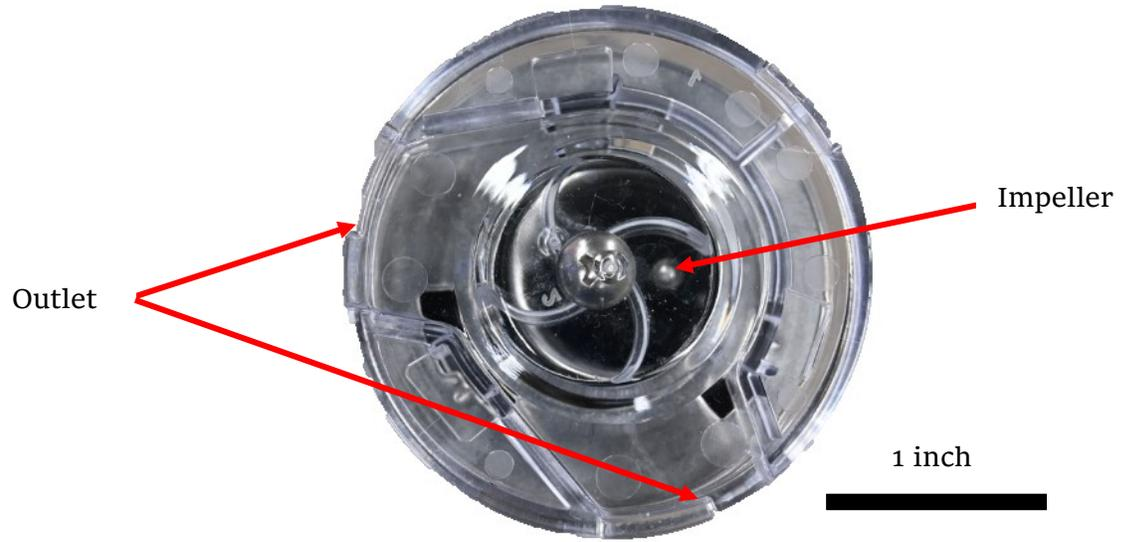
Figure 29: Bottom of sous vide heater showing the plastic centripetal pump casing with two outlets
