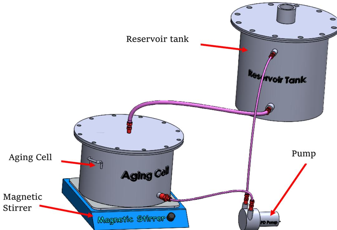
Figure 21: Initial aging design setup
