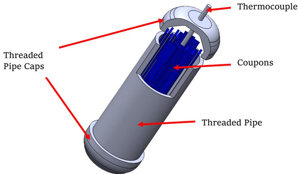
Figure 4: Current coupon aging setup (setup B)
