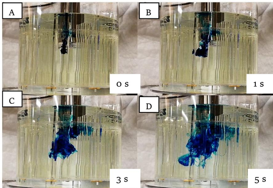
Figure 52: Dye test on initial carousel design with magnetic stirring only:
