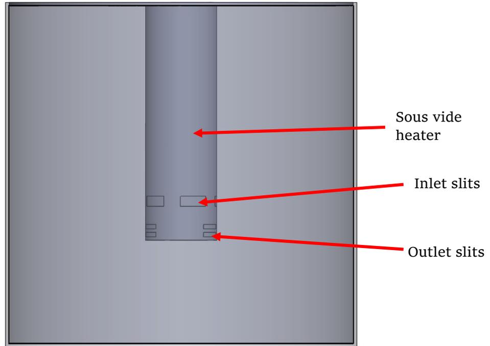
Figure 59: CFD domain with sous vide heater
