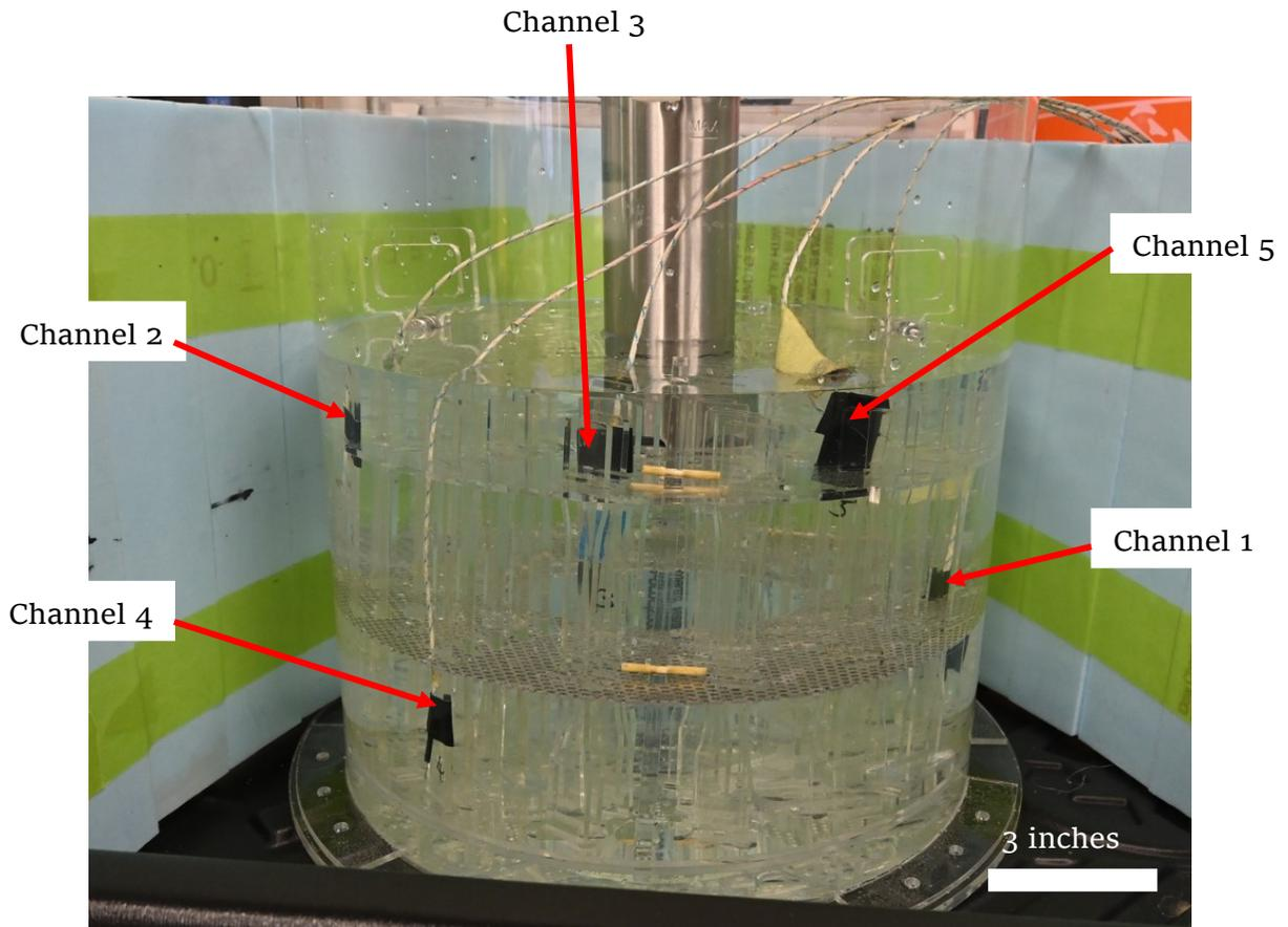
Figure 46: Acrylic aging cell with thermocouple setup
