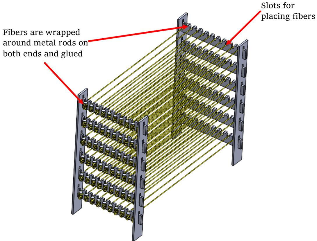
Figure 14: Design F concept of a fiber aging fixture
