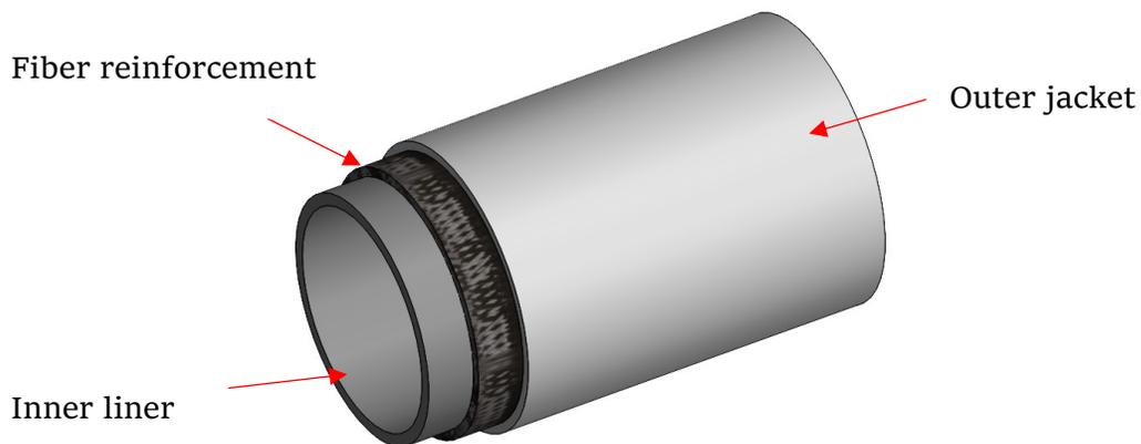
Figure 1: Schematic of reinforced thermoplastic pipe (RTP)
