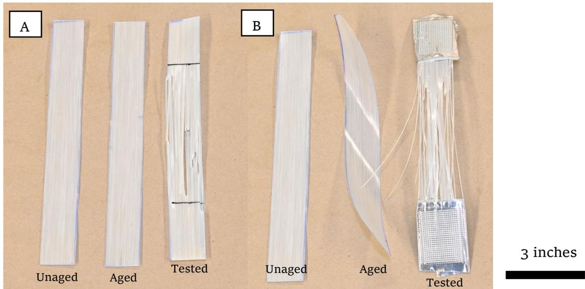
Figure 82: Fiber glass tapes: (A) PP impregnated from left to right unaged, 2 week aged, 2 week aged and tensile tested; (B) HDPE impregnated from left to right unaged, 2 week aged, 2 week aged and tensile tested
