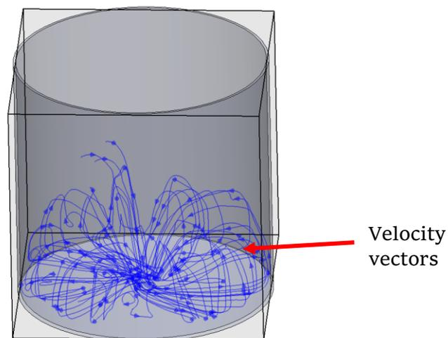
Figure 66: Velocity vectors of magnetic stirrer in aging cell
