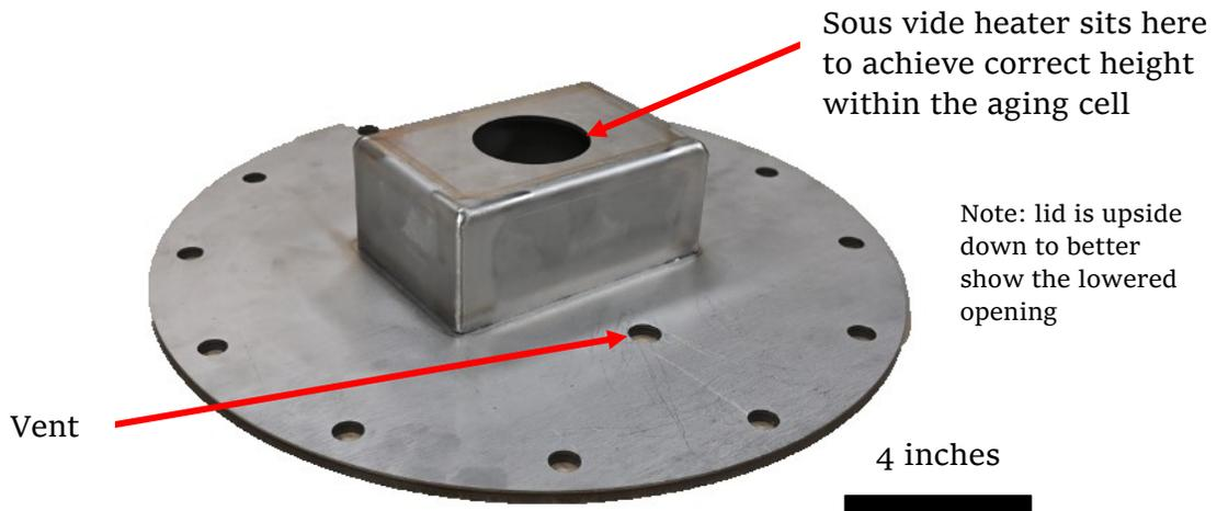
Figure 33: Stainless steel aging cell lid
