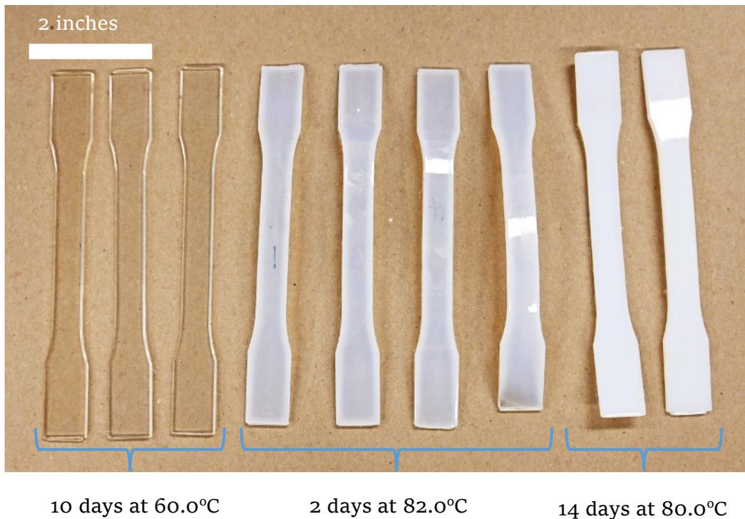
Figure 37: Polymer tensile test coupons aged at various temperatures and durations
