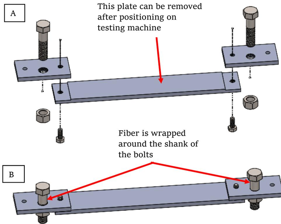
Figure 15: Design G concept of a fiber aging fixture: (A) exploded view, (B) assembled view
