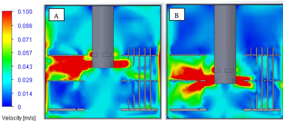
Figure 69: Vertical cross section of velocity profile with the perforated middle plate: (A) raised case, (B) centered case
