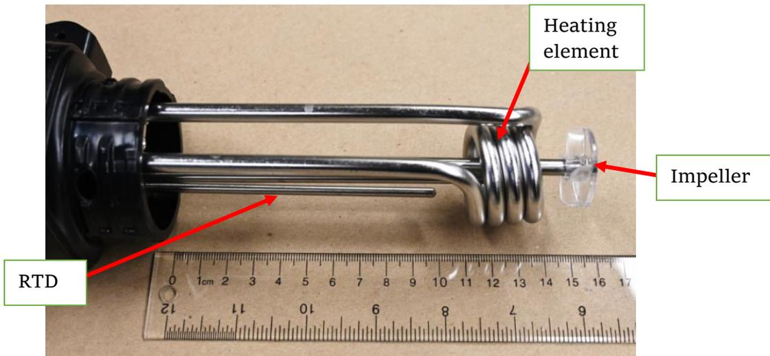
Figure 28: Inside of sous vide heater showing the RTD, heating element and open style impeller
