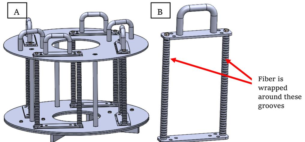
Figure 18: Design J concept of a fiber aging fixture and carousel: (A) aging fixtures inside of carousel, (B) aging fixture
