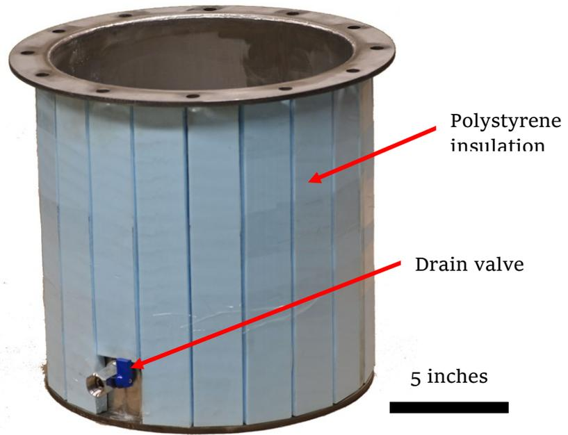
Figure 34: Stainless steel aging cell with insulation
