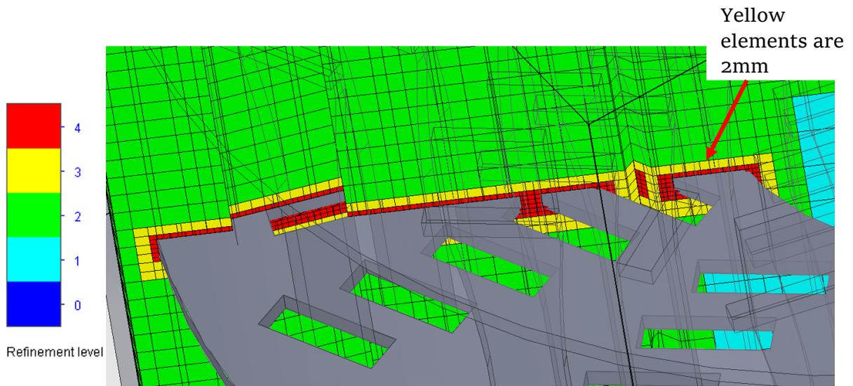
Figure 63: CFD mesh refinement detail
