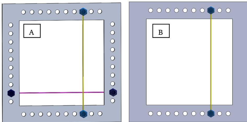
Figure 43: Design E concept of a fiber aging fixture: (A) original concept, (B) updated concept
