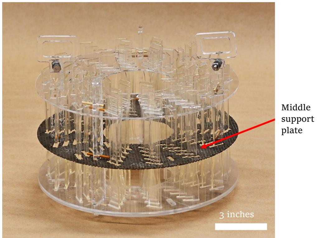
Figure 38: Acrylic carousel fitting with a stainless steel middle plate
