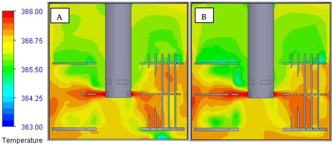
Figure 73: Vertical cross section of temperature profile with: (A) skeletonized middle plate, (B) full middle plate
