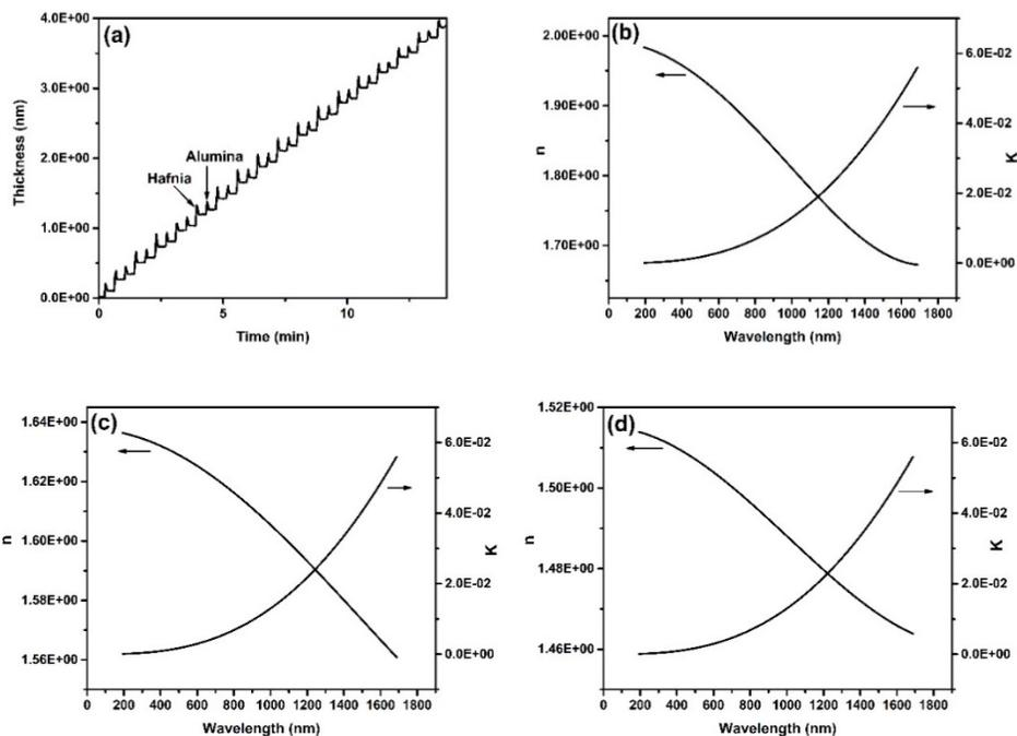
Figure 4-1(a) Thickness evolution of HAO gate dielectric during growth. Refractive index and extinction coefficient of (b) HZO, (c) HAO and (d) ZAO complex oxide dielectrics.
