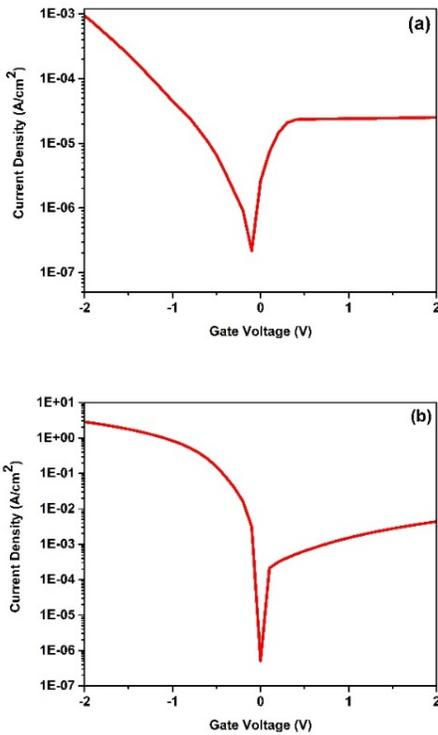
Figure 3-4 IV characteristics between -2V and 2 V of (a) plasma enhanced and (b) thermal ALD grown ZrO<sub>2</sub> MOSCAPs.
