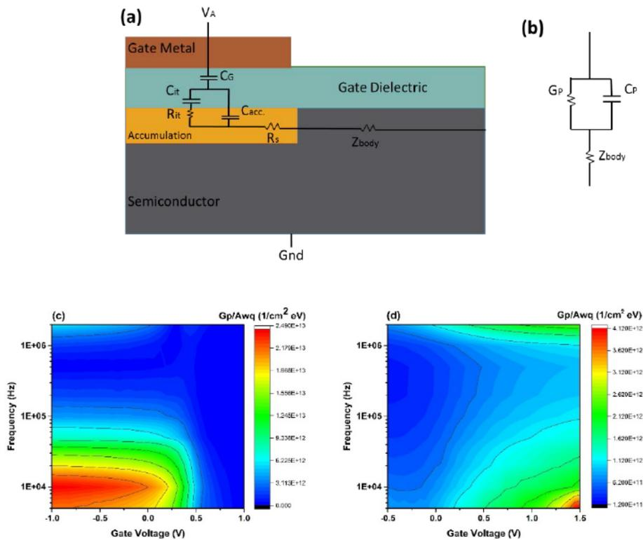
Figure 4-6(a) Equivalent circuit of a planar MOSCAP. (b) Simplified circuit layout of a planar MOSCAP. The parallel conductance ( $G_p$ ) with respect to gate voltage and sweeping frequency for hafnium zirconate dielectric on (c) silicon and (d) indium phosphide.
