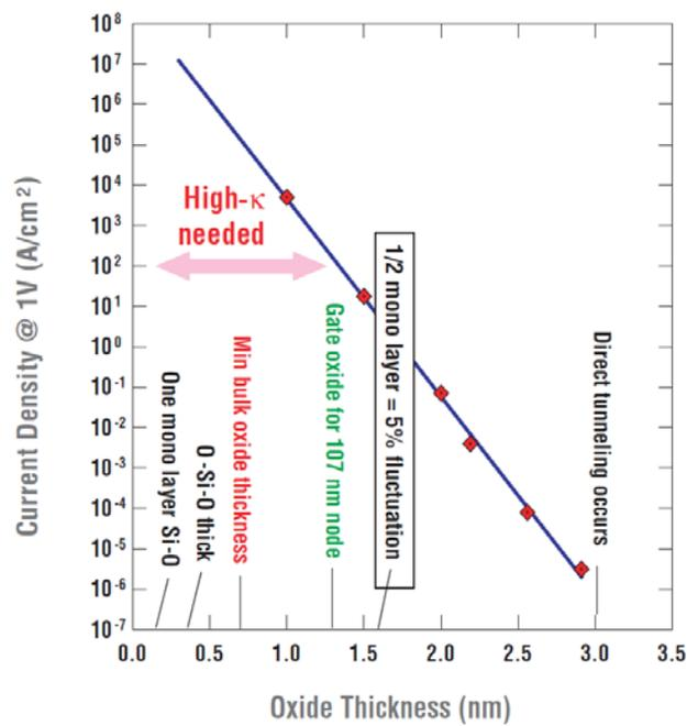
Figure 1-2 Gate dielectric leakage current increases exponentially with gate oxide thickness shrinkage<sup>10</sup>.
