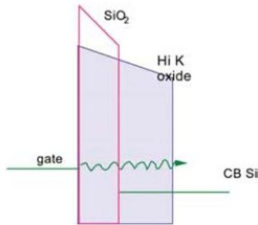
Figure 1-3 Schematic comparison between in  $\text{SiO}_2$  gate dielectrics and high- $\kappa$  gate dielectrics <sup>4</sup>.
