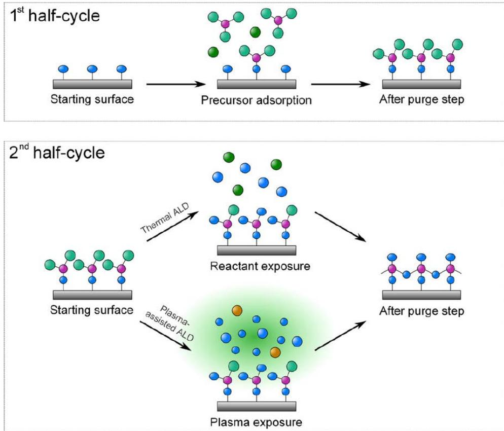
Figure 1-8 Schematic representation of one atomic layer deposition cycle
