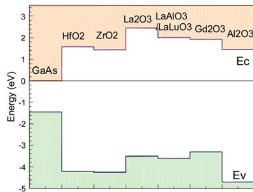
Figure 1-5 Band offsets of gate dielectric candidates over GaAs <sup>12</sup>.
