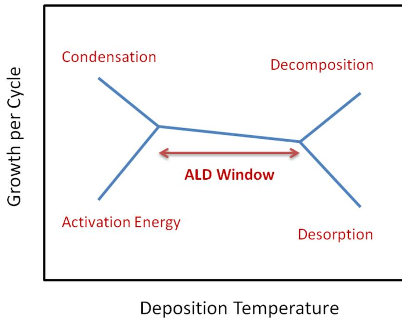
Figure 1-9 Schematic of ALD window with possible growth per cycle behavior<sup>29</sup>.
