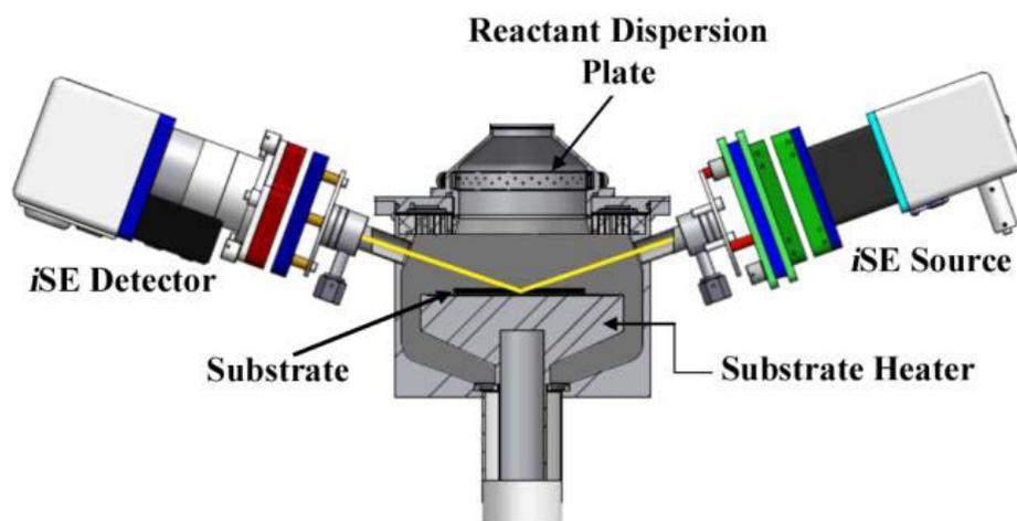
Figure 2-4 Schematic illustration of the in-situ spectroscopic ellipsometry mounted on ALD reactor <sup>65</sup>.
