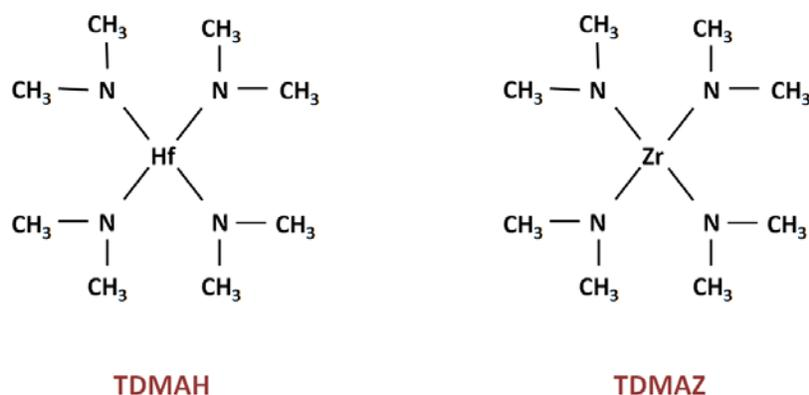
Figure 2-5 Chemical structure of the tetrakis(dimethylamino) hafnium (TDMAH) and tetrakis(dimethylamide) zirconium (TDMAZ), utilized as ALD precursors for Hf and Zr, respectively<sup>29</sup>.
