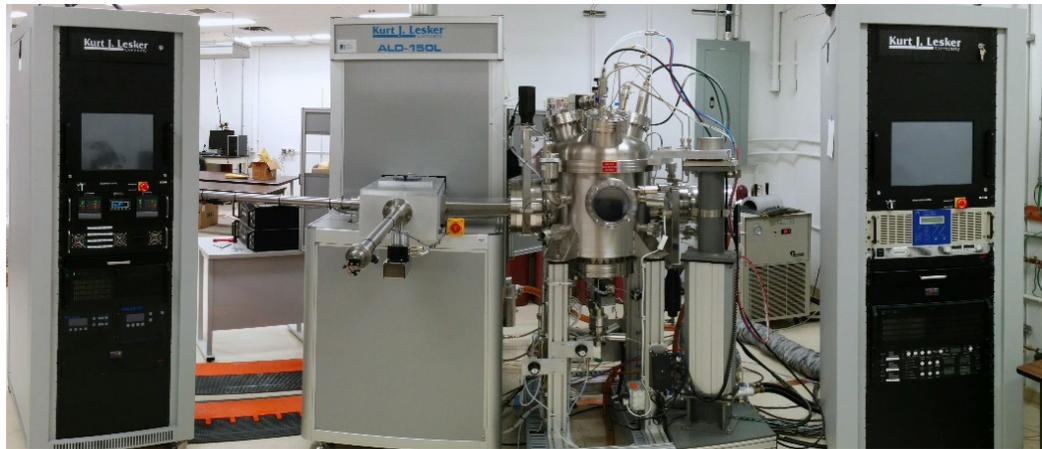
Figure 2-1 The view of the ALD system in our lab.
