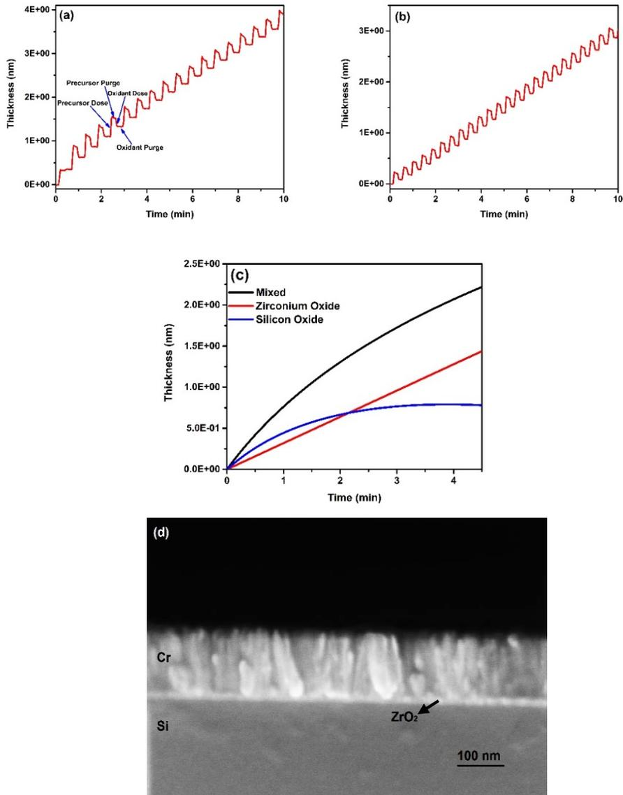
Figure 3-1 Real time thickness evolution of PEALD (a) and TALD (b) ZrO<sub>2</sub> thin films during growth (determined from in-situ ellipsometry using a Tauc-Lorentz model). (c) Resolving contributions of zirconium oxide and silicon oxide in PEALD grown ZrO<sub>2</sub> thin films assuming constant
