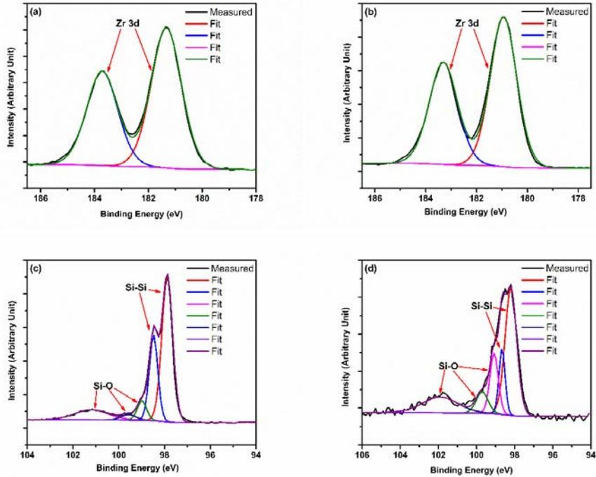
Figure 3-2 XPS results for Zr 3d for (a) TALD and (b) PEALD grown as-deposited zirconia films. Figure 3 (c) and (d) Si 2p substrate XPS peaks for TALD and PEALD grown as-deposited  $ZrO_2$ , respectively.
