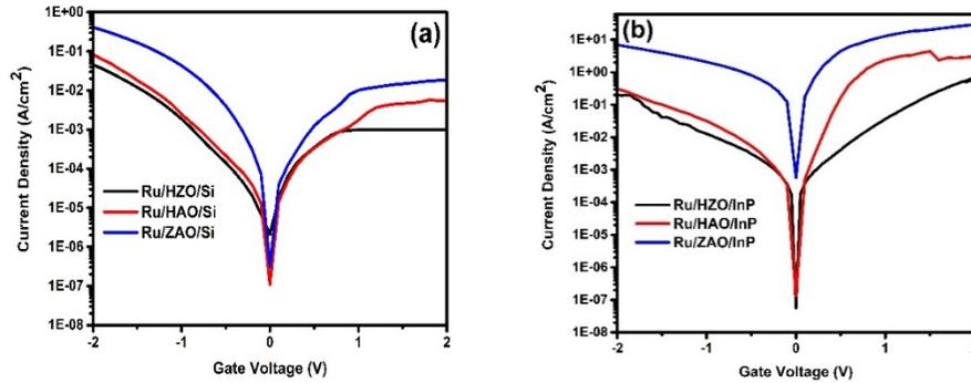
Figure 4-5 The gate dielectric leakage current for hafnium zirconate (HZO), hafnium aluminate (HAO), and zirconium aluminate (ZAO) dielectric MOSCAPs on (a) silicon and (b) indium phosphide substrates.
