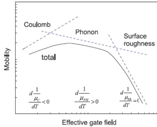
Figure 1-7 Carrier mobility with respect to effective gate field <sup>4</sup>.
