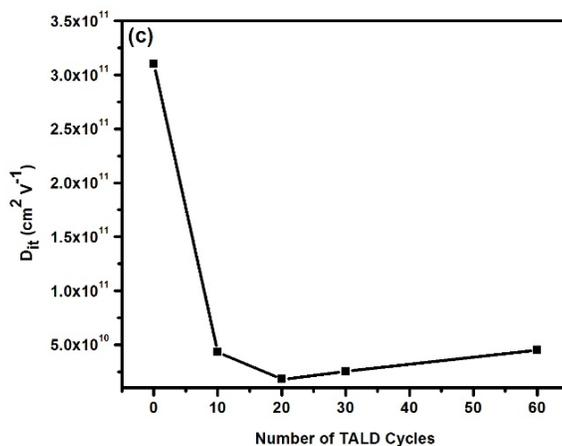
Figure 3-5 Conductance map between 0 V to 2 V and 10 KHz to 2 MHz of  $\text{ZrO}_2$  gate dielectric MOSCAPs with (a) 0 and (b) twenty cycles of thermal ALD. (c) Density of interfacial traps with respect to number of TALD cycles (total number of cycles were 60 for all specimens).
