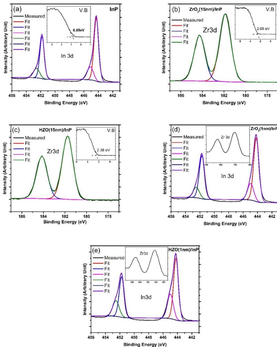
Figure 4-7 Shallow core-level and VB photoelectron spectra for (a) bare n-InP(100), (b) 15 nm  $\text{ZrO}_2/\text{InP}$ , (c) 15nm  $\text{Hf}_{1-x}\text{Zr}_x\text{O}_2(\text{HZO})/\text{InP}$ , (d) 1.4 nm  $\text{ZrO}_2/\text{InP}$ , and (e) 1.4 nm  $\text{Hf}_{1-x}\text{Zr}_x\text{O}_2(\text{HZO})/\text{InP}$  heterojunctions. The insets show high resolution scans of the VB regions for the bare (a) n-InP(100), (b) 15 nm
