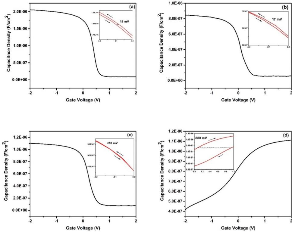
Figure 4-3 CV characteristics between -2V and 2 V of (a) hafnium zirconate, (b) hafnium aluminate and (c) zirconium aluminate gate dielectric MOSCAPs on P-type silicon (100) substrate at 100 KHz. Figure 3(d) illustrates the CV characteristics of between -2V and 2 V of hafnium zirconate gate dielectric MOSCAP on InP at 100 KHz. (Insets: hysteresis of C-V cycles at 100 KHz)
