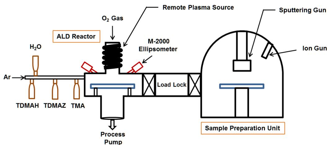
Figure 2-2 The schematic view of the ALD system in our lab<sup>29</sup>.
