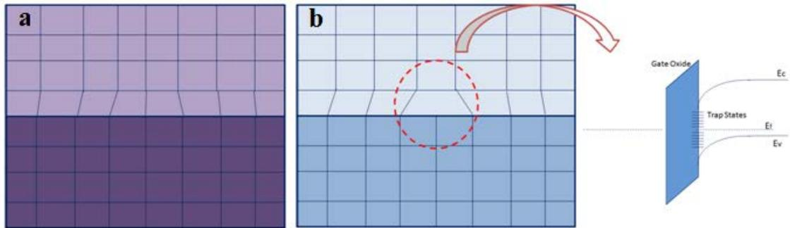
Figure 1-6 (a) Schematic view of heteroepitaxial growth and (b) the higher degree of mismatch relaxed through formation of interfacial faults.
