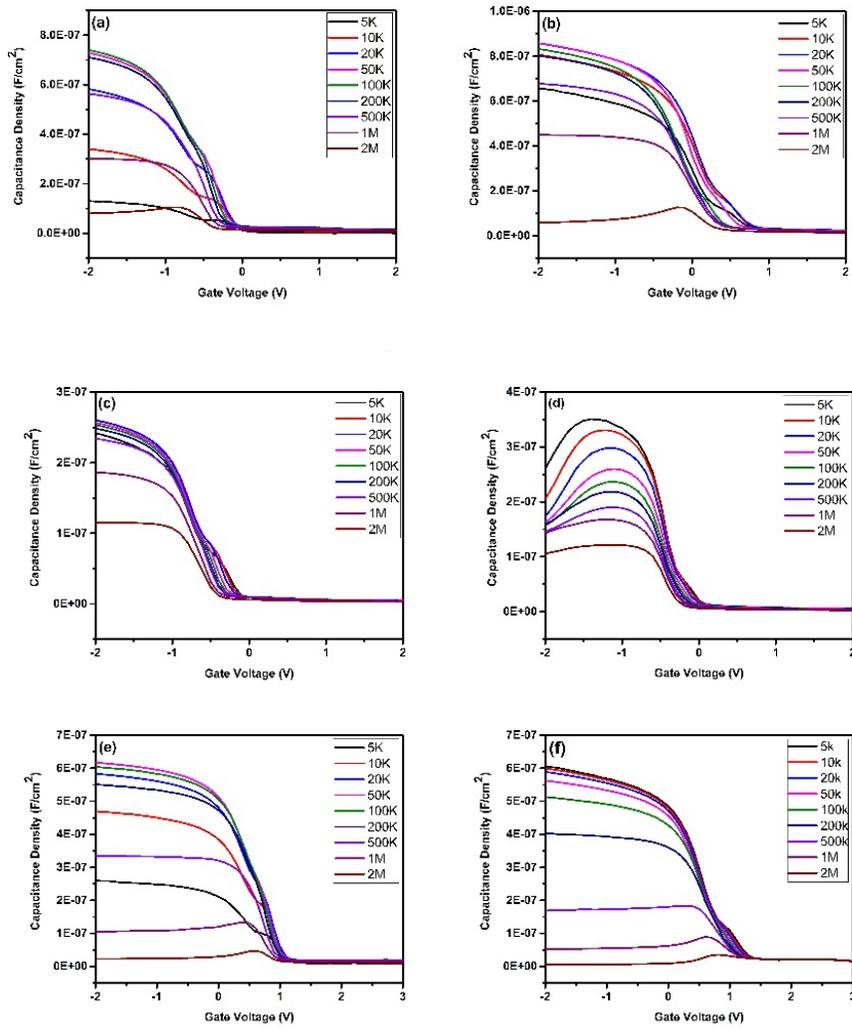
Figure 3-3 CV characteristics between -2V and 2 V of  $ZrO_2$  gate dielectric MOSCAPs with (a) 0 and (b) 10, (c) 20 and (d) 60 cycles of thermal ALD. CV characteristics of between -2V and 3 V of  $HfO_2$  gate dielectric MOSCAPs with (e) 0 and (f) 10 cycles of thermal ALD (the total number of cycles was kept 60 for all specimens).
