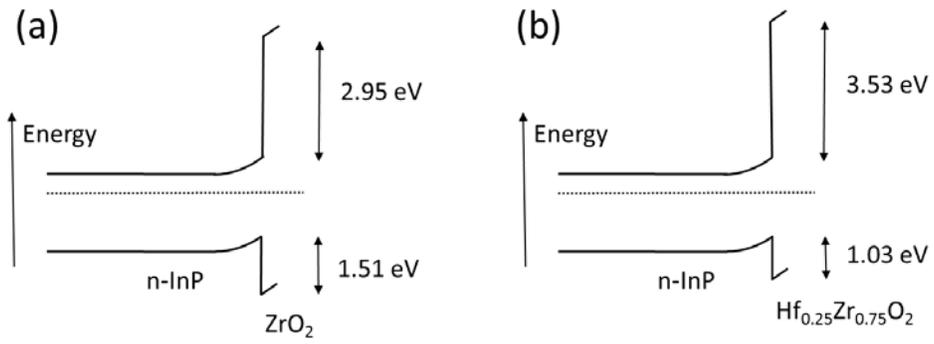
Figure 4-8 Band diagrams for (a) ZrO<sub>2</sub>/n-InP(100) and (b) Hf<sub>0.25</sub>Zr<sub>0.75</sub>O<sub>2</sub>/n-InP(100) heterojunctions.
