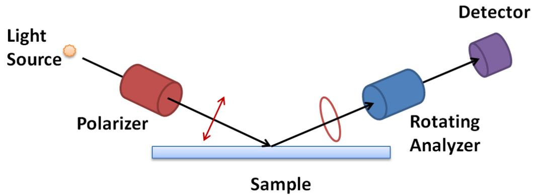
Figure 2-3 A schematic illustration of a typical ellipsometry set up<sup>29</sup>.
