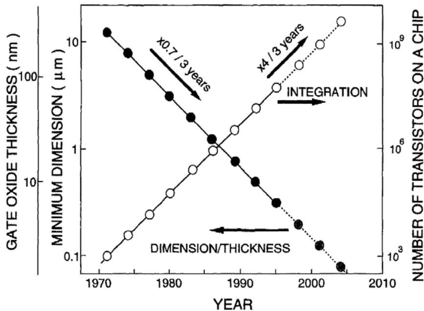
Figure 1-1 MOS transistor scaling from 1972 to 2004<sup>3</sup>.
