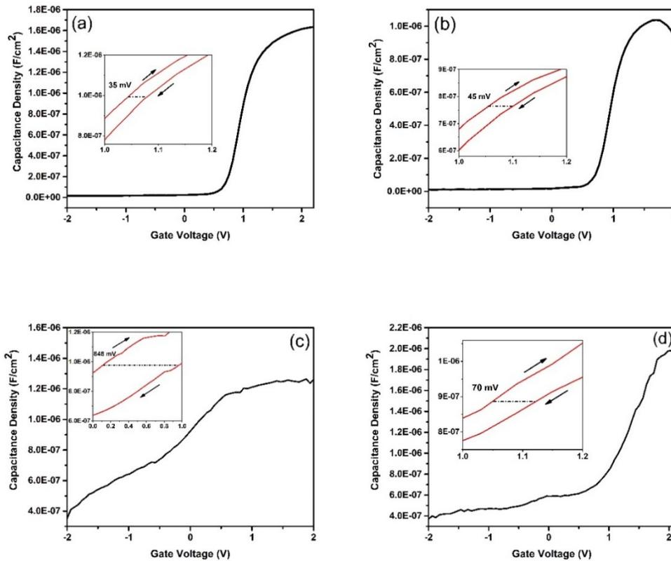
Figure 4-4 CV characteristics between -2V and 2 V of MOSCAPs at 10KHz (a) stacked on GaN, (b) nanolaminated on GaN, (c) stacked on InP and (d) nanolaminated on InP. Inset is the hysteresis in the CV characteristics of GaN and InP MOSCAPs at 10 KHz.
