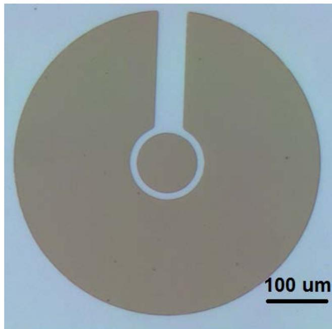
Figure 2-6 The top view of the planar MOSCAP devices.
