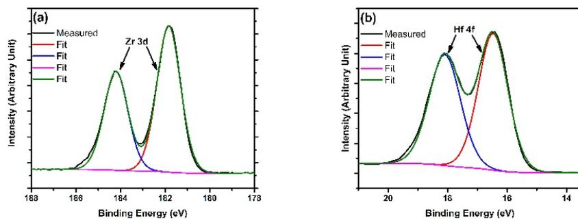
Figure 4-2(a) and (b) show the x-ray photoelectron spectroscopy (XPS) results for Zr and Hf in 15 nm thick hafnium zirconate.
