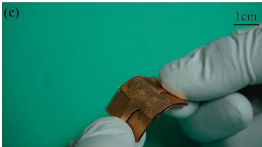
Figure 5.18 The fabricated flexible filter. (a) The flexible filter is in the rectangular shape as designed. (b) and (c) The flexible filter can be easily bent by two fingers.
