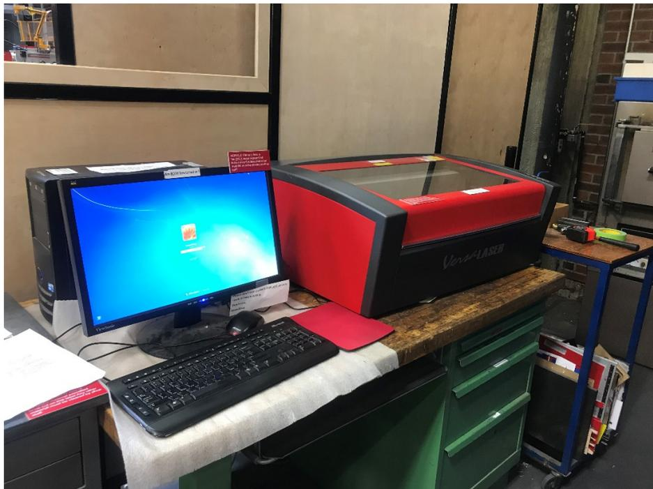
Figure 5.8 An overview of the CO<sub>2</sub> laser cutter used for the via patterning.
