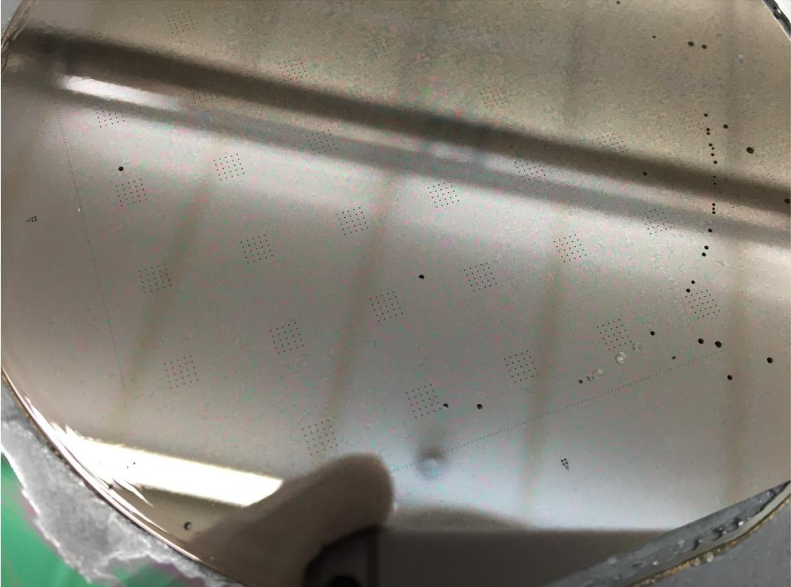
Figure 3.6 A close look at vias formed on a wafer after DRIE. Apart from desired vias, defects (bigger holes close to the edge) can be found too.
