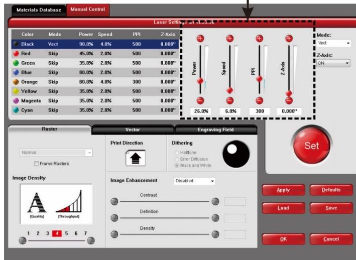
Figure 5.9 The user interface of the laser cutter. Several important settings for the laser are mode-vector, power-26%, speed-6% and PPI-300.
