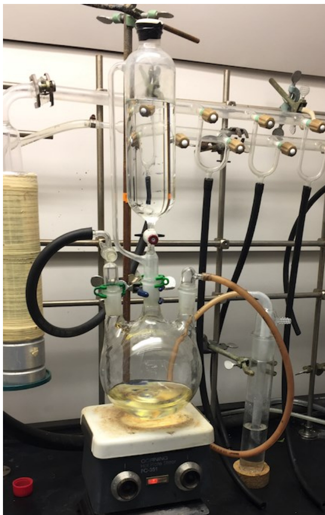
Figure 2.1. The apparatus for synthesizing HSQ.
