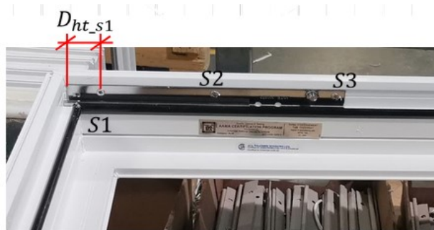
Figure 9. Hinge track screw position on frame
