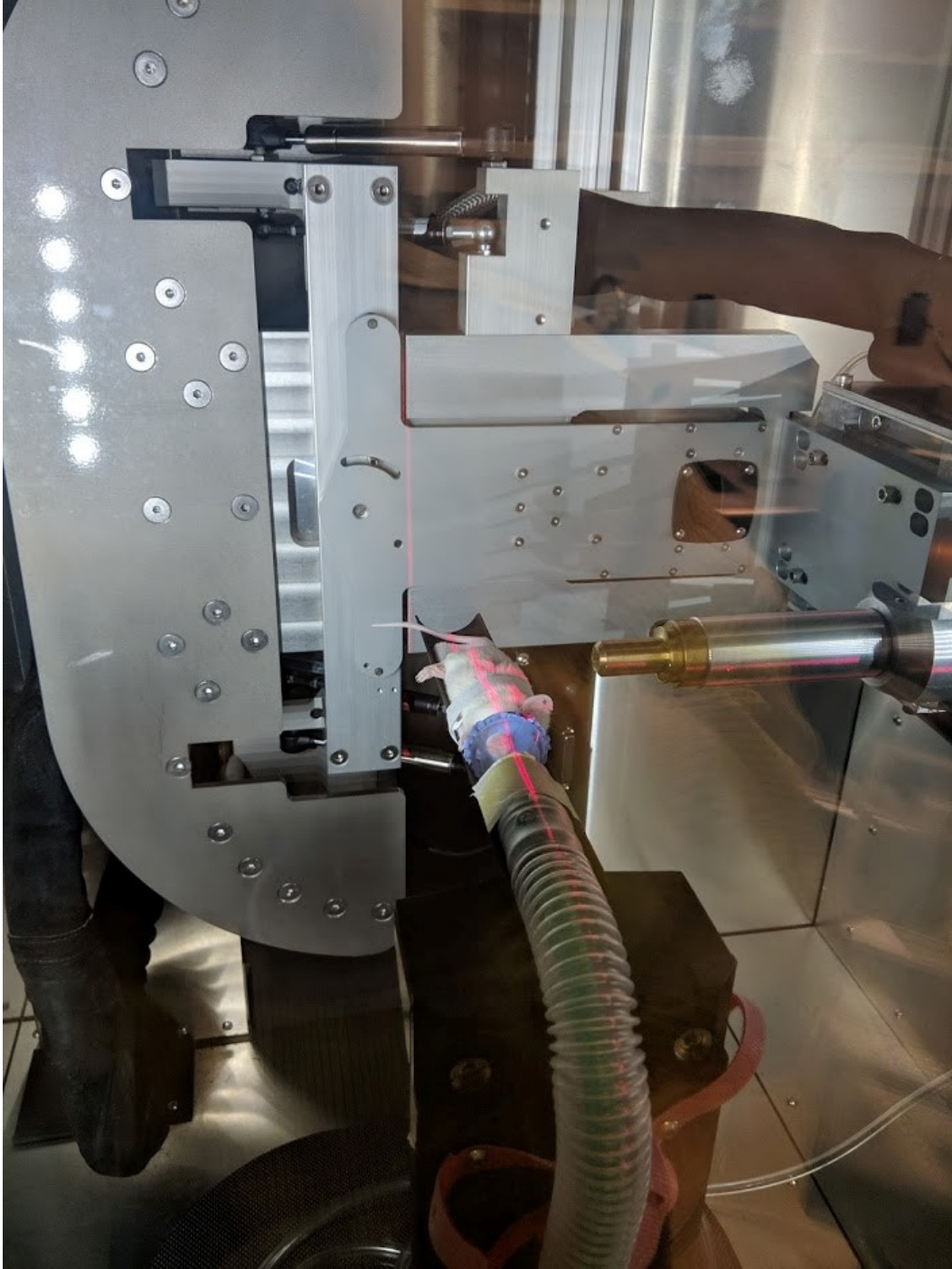
Figure 3.6: Setup of animal on SARRP system for irradiation. The mouse was positioned on the flank contralateral to the tumor thereby raising the tumor above the plane of most of the animal's body allowing targeting with tangential beams.
