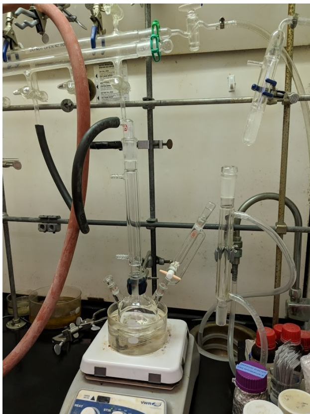
Figure 2.1 Synthesis setup for anhydrously synthesized \text{LaF}_3:\text{Ce}^{3+} NSC.
