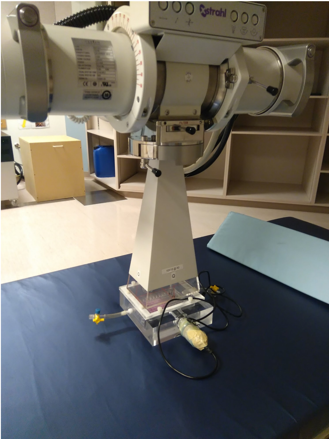
Figure 3.4. Experimental setup of in vitro irradiation conditions using an Xstrahl 300 clinical irradiator (Camberley, Surrey, UK) and an in-house developed hypoxia chamber.
