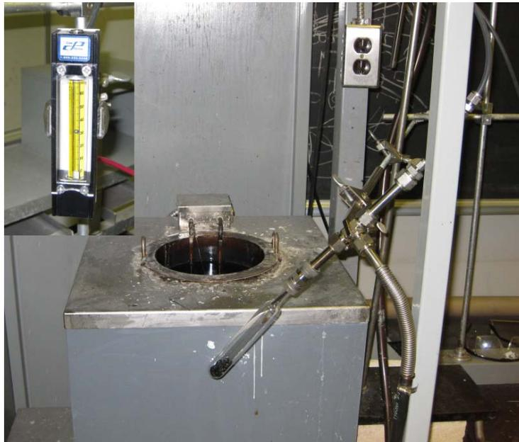
**Figure 3.12. Quartz tube and Nitrogen flow rate during purge stage**
