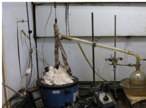
**Figure 3.5. Distillation assembly**
