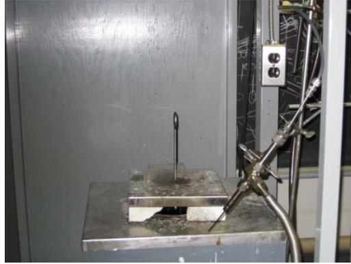
**Figure 3.7. Molten salt bath container and coking setup**
