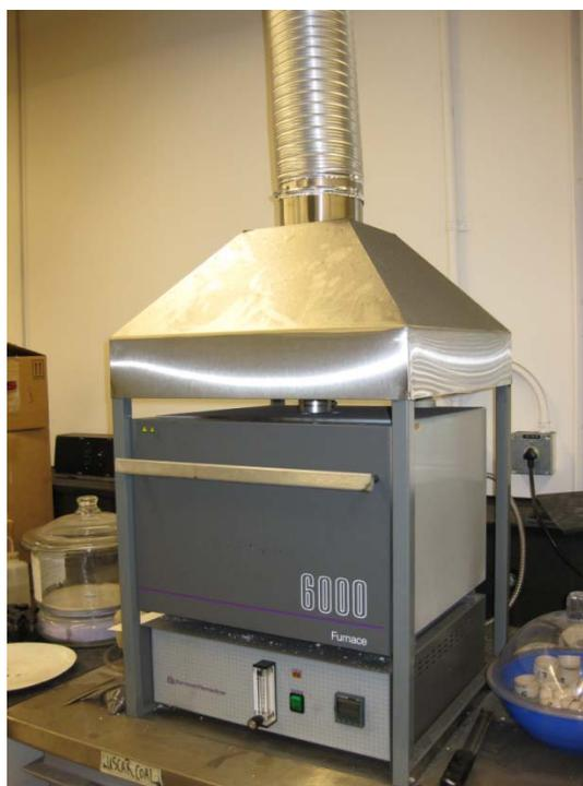
**Figure 3.15. Muffle furnace and the crucibles used for ash measurements**
