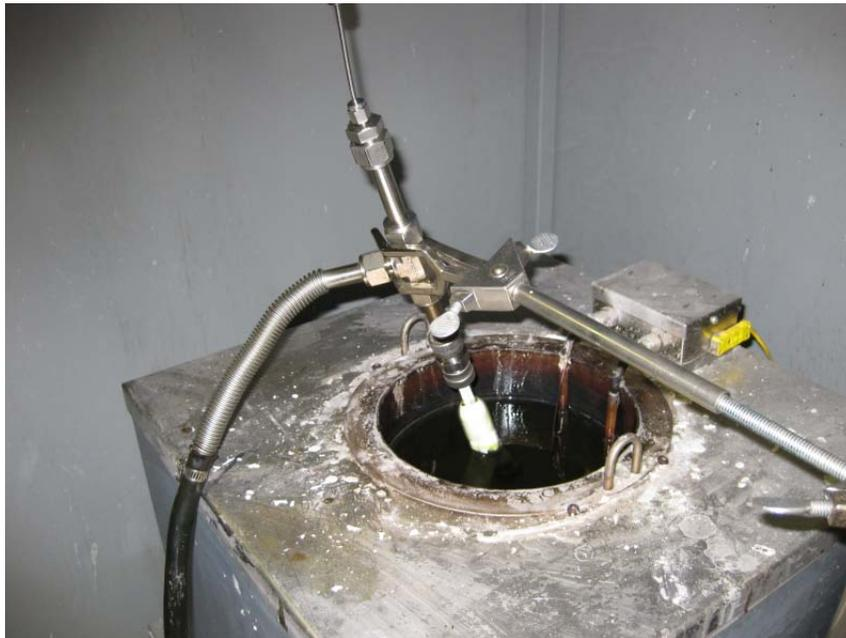
**Figure 3.13. Violent devolatilization in the start of coking experiment**
