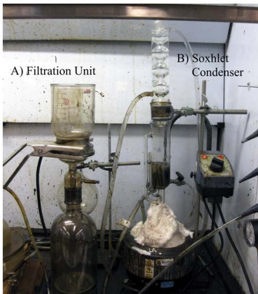
**Figure 3.4. Filtration unit and Soxhlet Condenser**
