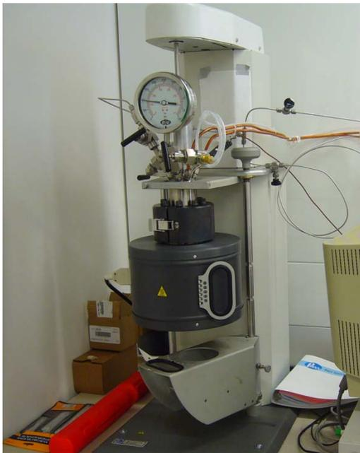
**Figure 3.2. 500 ml reactor used in liquefaction experiments**
