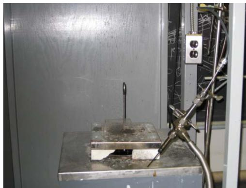
**Figure 3.7. Molten salt bath container and coking setup**
