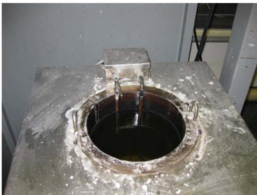
**Figure 3.6. Molten salt bath container**
