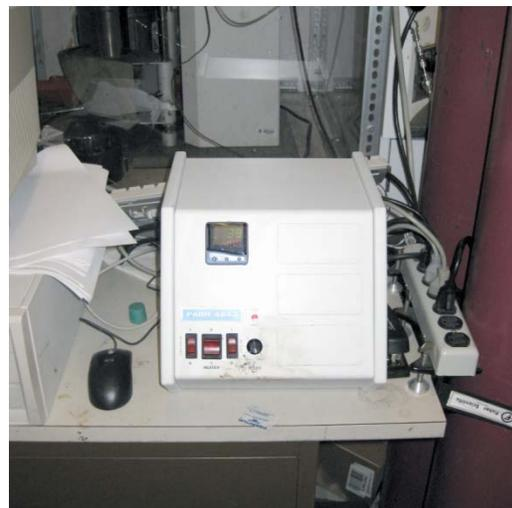
**Figure 3.3. Control console of the reactor**
