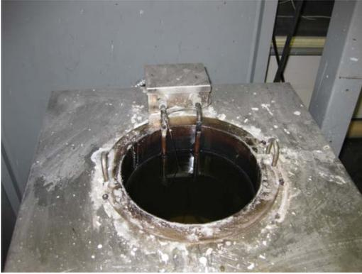
**Figure 3.6. Molten salt bath container**
