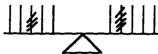
Figure 20: The balance scale with 5 pegs on each side. The left side has 3 metal disks on middle peg. The right side has 5 metal disks on the second peg from the fulcrum.
