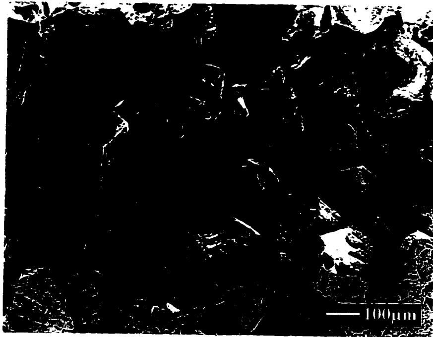
Photo 5-11: SEM Image of Reconstituted Sand Sample Subject to Freezing Cycles showing Alignment of the Thin Clay Mineral Edge Perpendicular to the Freeze Front.
