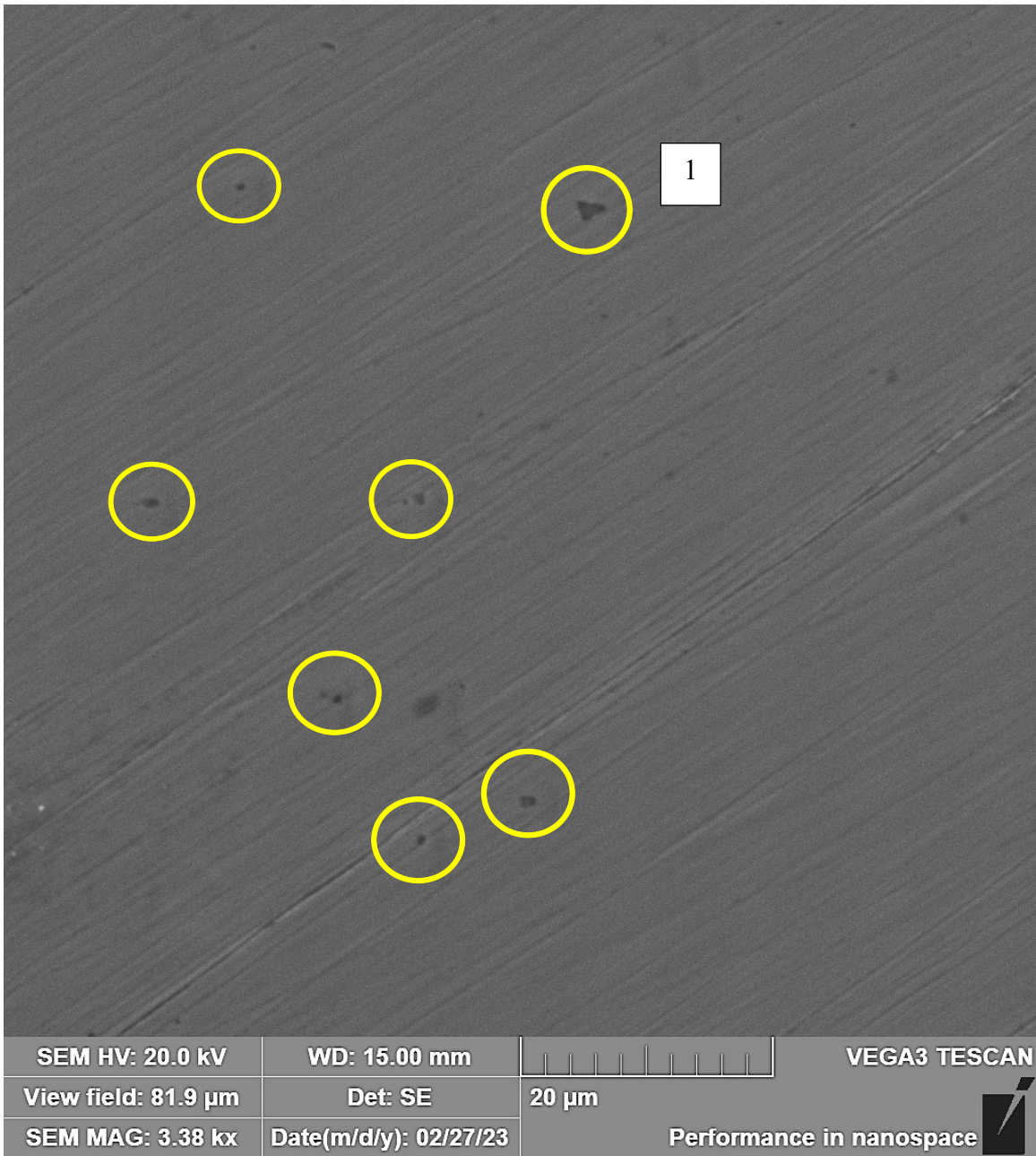
Figure 5.3 SEM image of a seven clustered (Ti,Nb)N in sample 4280
