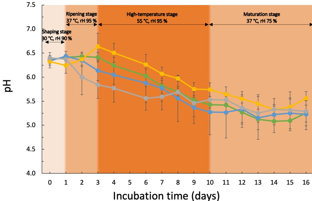
**Figure 3.3** The pH tested during the fermentation of the simplified *daqu* model. Different line colors indicate the different strains inoculated in the *daqu* fermentation: green, *B. amyloliquefaciens* Fad We; blue, *B. amyloliquefaciens* Fad 82; yellow, *B. velezensis* FUA2155; and gray, control (without addition of *Bacillus* strain). Different stages of fermentation were differentiated by the color of background.
