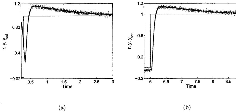
Figure 4.7: Closed loop step response of the process and model (example 2). (a) Identification data (b) Validation data.
