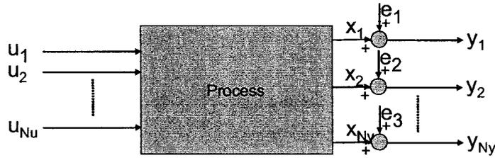
Figure 5.1: Block diagram of a MIMO open-loop process with  $N_u$  inputs and  $N_y$  outputs.
