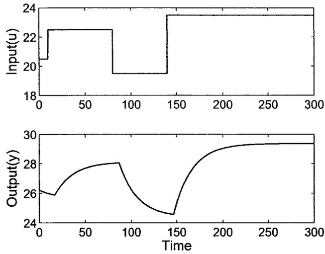
Figure 4.3: *Output response of the process (example 1) to three successive steps in the input.*
