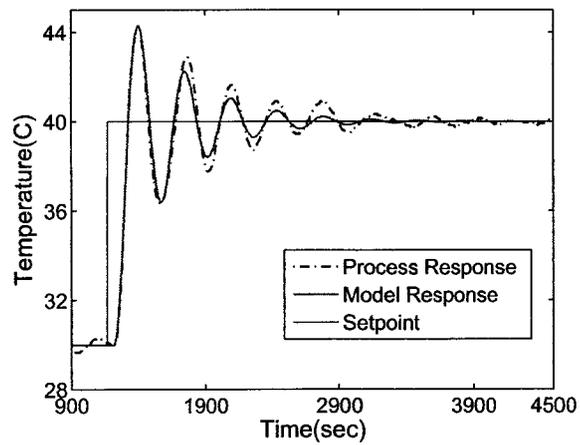
Figure 4.13: *Closed loop response of the heating tank process and its estimated model for a step change in steam flow.*
