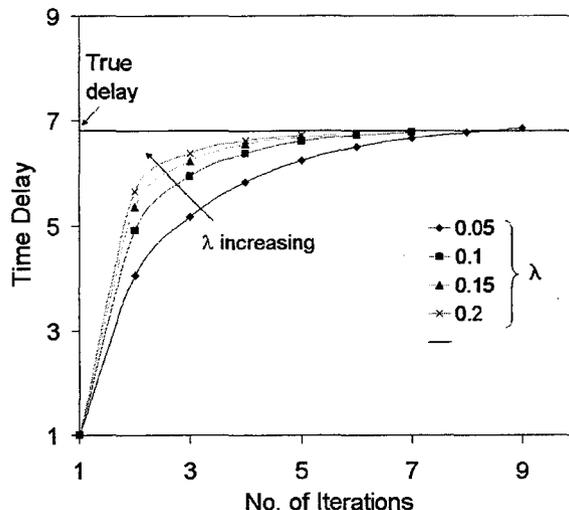
Figure 2.3: *Effect of filter parameter on the rate of convergence.*
