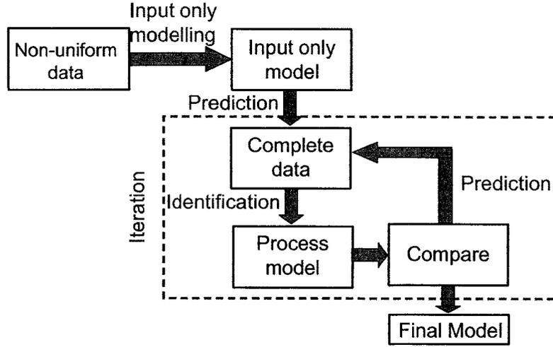
Figure 3.1: Graphical representation of the iterative prediction algorithm for identification from non-uniformly sampled data.
