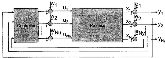
Figure 5.2: *Block diagram of a MIMO process under closed loop with dither inputs.*
