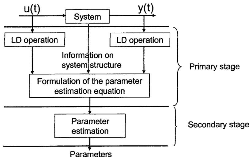
Figure 1.1: *General scheme for continuous-time parameter estimation.*
