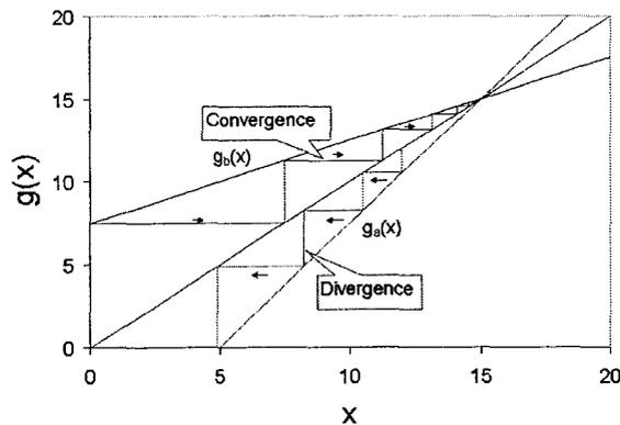
Figure A.1: *Graphical representation of fixed point iteration.*
