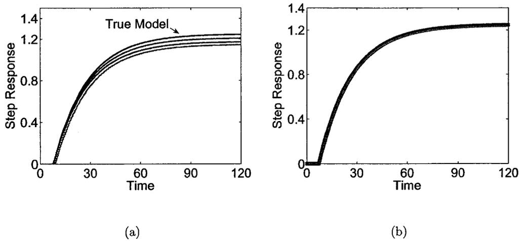
Figure 4.4: *Step responses of the estimated models using (a) MATLAB SYSID Toolbox (b) proposed method (example 1).*
