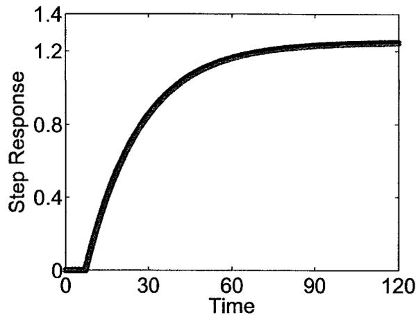
Figure 4.6: *Step responses of the estimated models using data when process initially at far away from steady state (example 1).*
