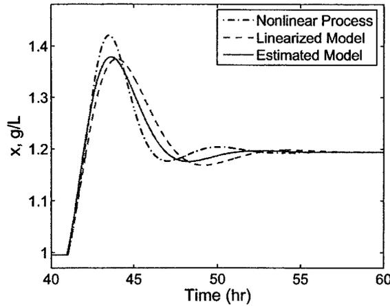
Figure 4.9: *Closed loop step response of the nonlinear bio-reactor model, linearized model and the estimated linear model (example 3).*
