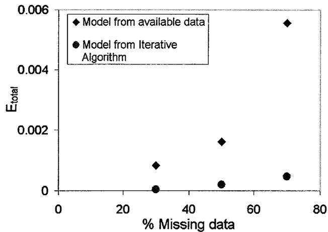
Figure 3.5: *Improvement of model quality using the iterative algorithm for the mixing process.*
