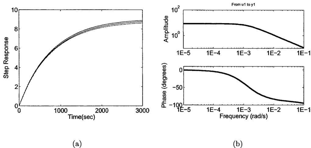
Figure 4.11: *Step and frequency responses of the three identified model of the mixing process.*
