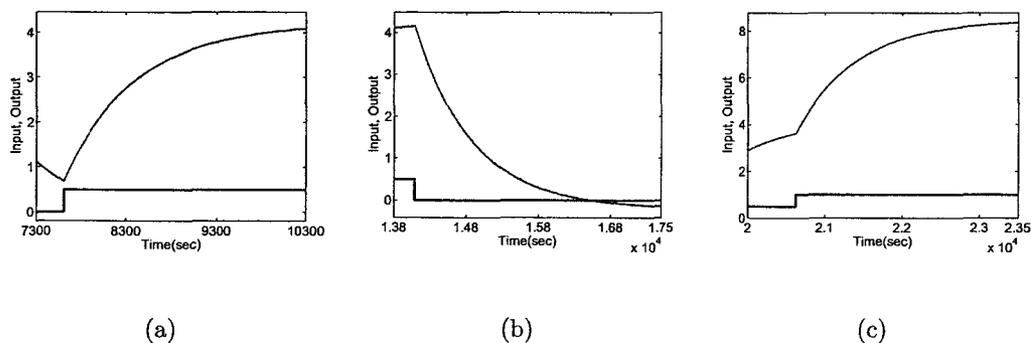
Figure 4.10: *Step response of the mixing process with different initial conditions.*
