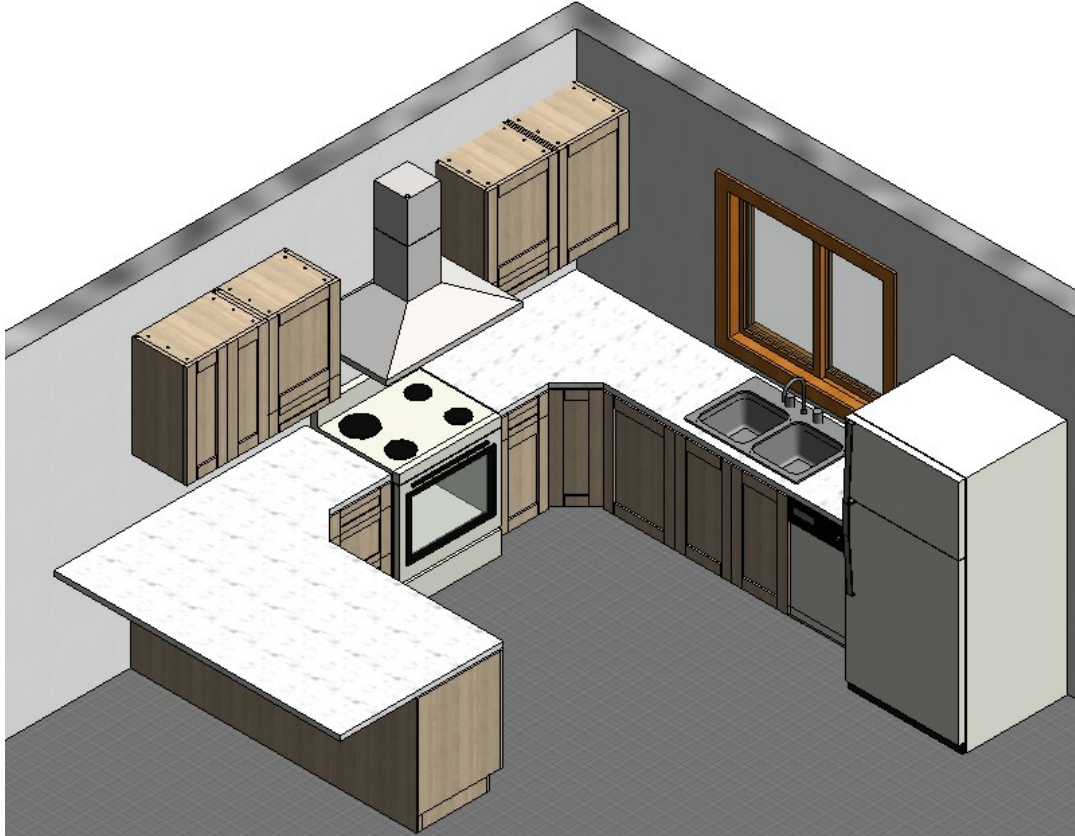
Figure 4-13: Auto-generated cabinet layout plan using the prototype system
