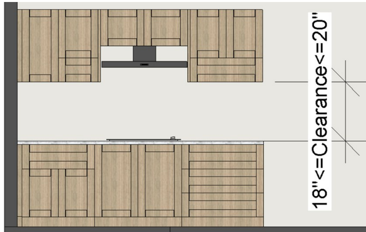
Figure 3-8: Rule of Clearance between the top of countertop to the bottom of wall cabinet.
