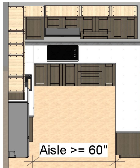
Figure 3-7: Rule of walking aisle width for U-shaped layout.
