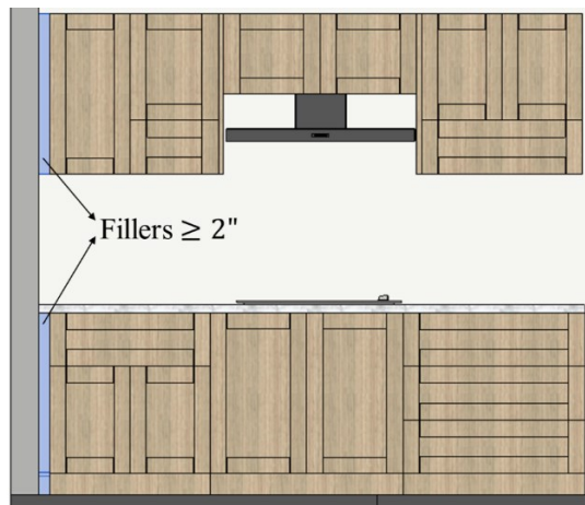
Figure 3-11: Fillers between cabinets and wall
