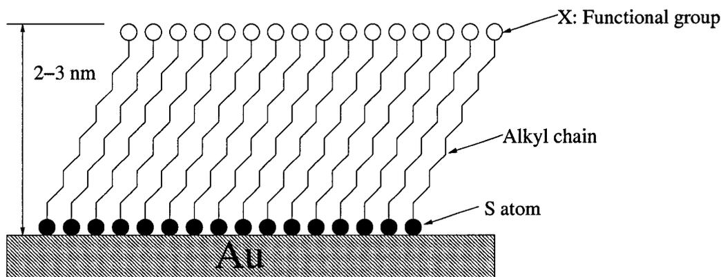
Figure 2.1: Schematic of a highly ordered monolayer of alkanethiolate formed on a gold surface.
