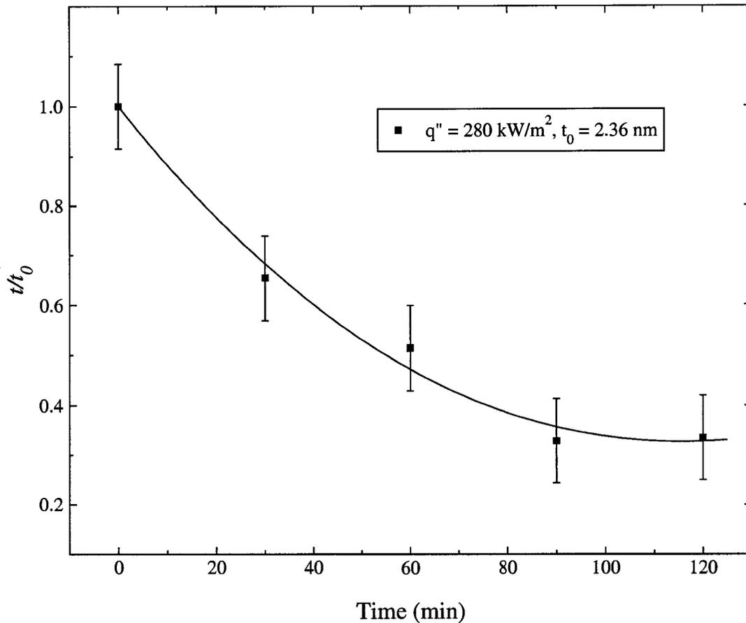
Figure 4.4: Normalized thickness of SAMs derived from 1-octadecanethiol on gold-coated-copper substrates as a function of condensation duration for heat flux  $q'' \approx 280 \text{ kW/m}^2$ .  $t_0$  is the initial film thickness reference. Error bars are  $\pm 0.2 \text{ nm}$  in reference to  $t_0$  and represent typical measurement errors for ellipsometry.
