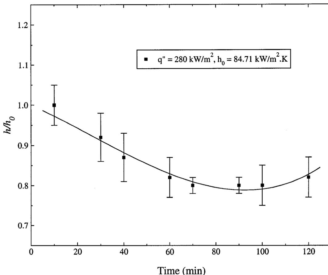
Figure 4.5: Normalized heat transfer coefficient as a function of condensation duration for heat flux  $q'' \approx 280 \text{ kW/m}^2$ .  $h_0$  is the heat transfer coefficient after 10 minute condensation. Error bars are 95% confidence limits.
