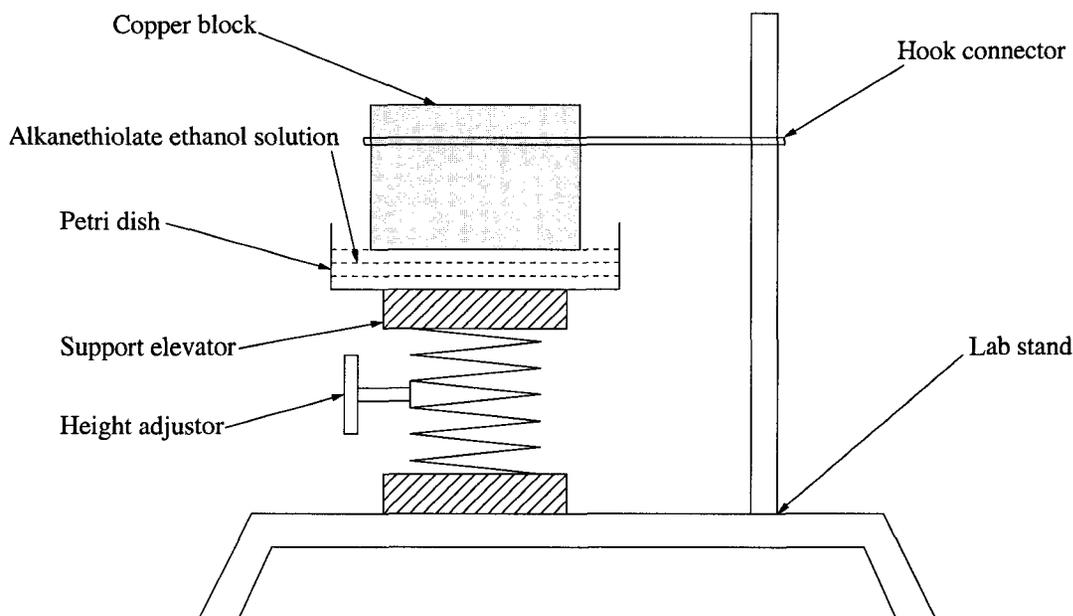
Figure 3.3: Schematic of the deposition of alkanethiol SAMs on a copper surface.
