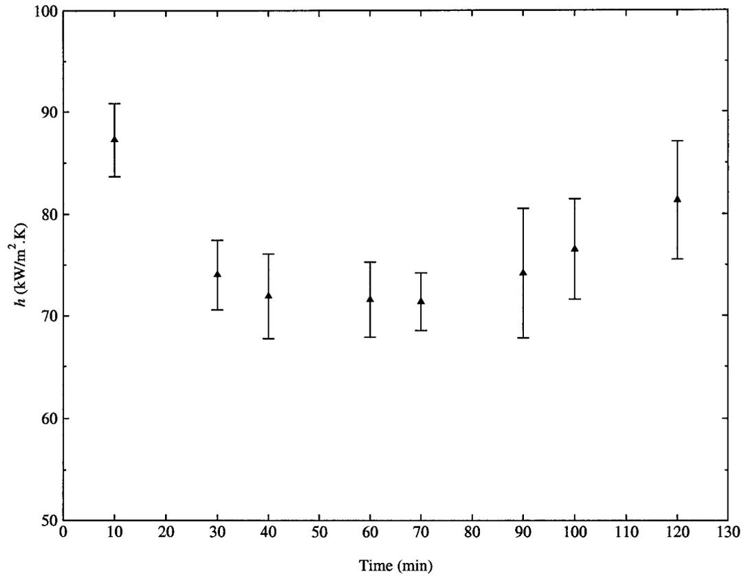
Figure 4.9: Heat transfer coefficient as a function of condensation duration for heat flux  $q'' \approx 400 \text{ kW/m}^2$ . Error bars are 95% confidence limits.
