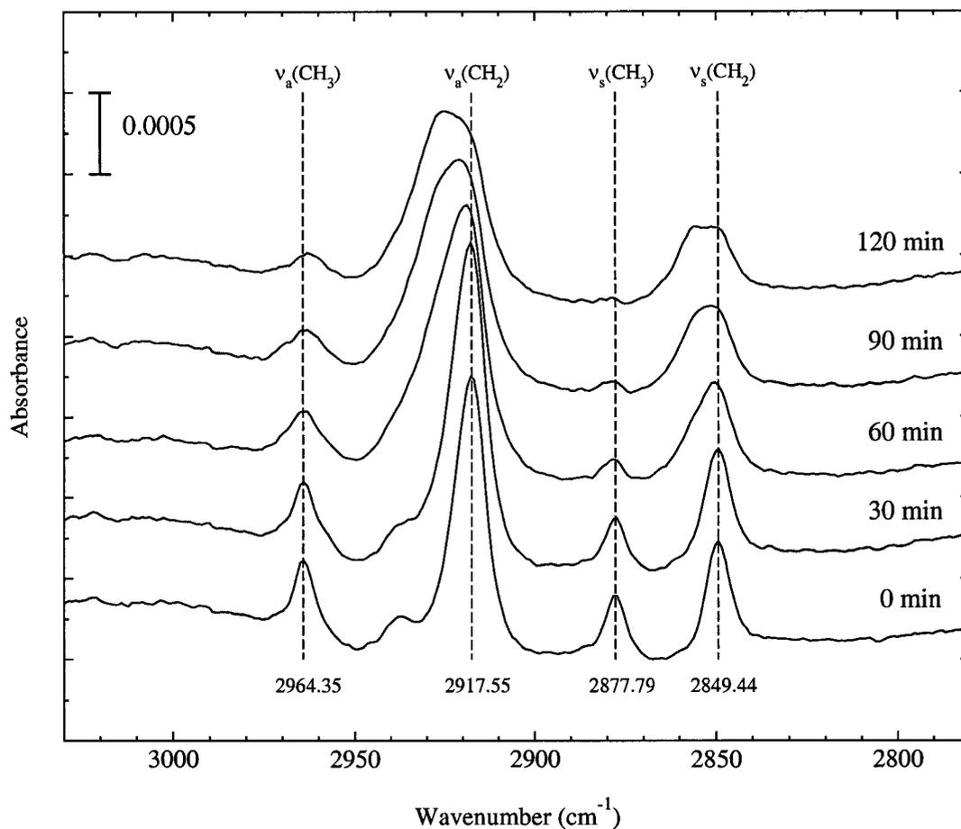
Figure 4.3: Reflectance FT-IR spectra for SAMs derived from 1-octadecanethiol on Au/Ti/Cu substrates subjected to steam condensation in various duration ( $q'' \approx 280 \text{ kW/m}^2$ ). The dashed lines represent the positions of the original modes for a trans-extended monolayer. The spectra have been offset for clarity.
