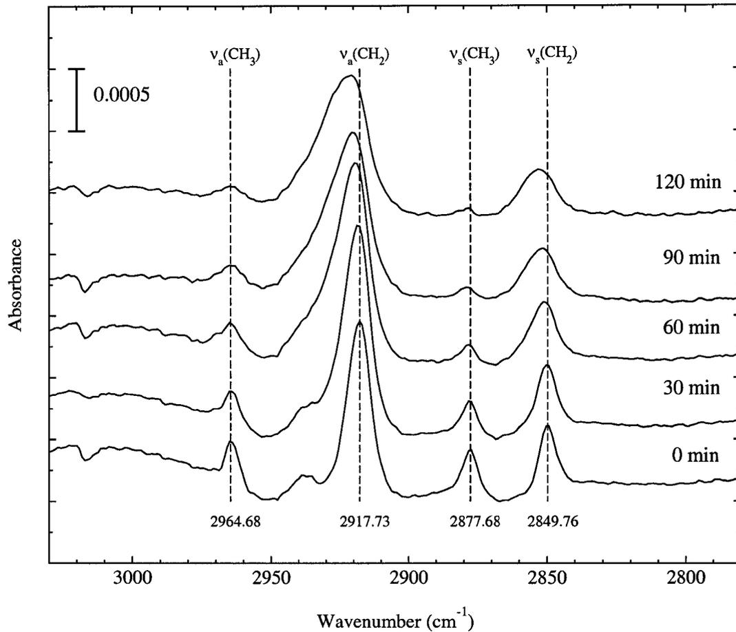
Figure 4.12: Reflectance FT-IR spectra for SAMs derived from 1-octadecanethiol on Au/Ti/Cu substrates subjected to steam condensation in various duration ( $q'' \approx 360 \text{ kW/m}^2$ ). The dashed lines represent the positions of the original modes for a trans-extended monolayer. The spectra have been offset for clarity.
