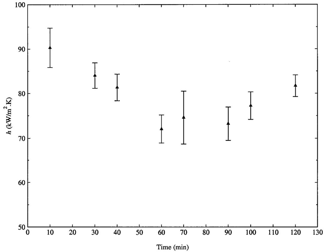
Figure 4.7: Heat transfer coefficient as a function of condensation duration for heat flux  $q'' \approx 320 \text{ kW/m}^2$ . Error bars are 95% confidence limits.
