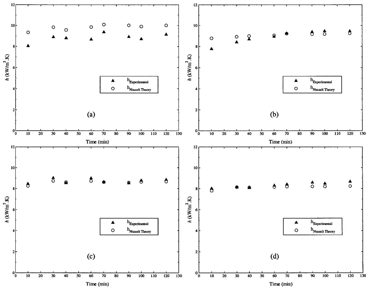
Figure 4.6: Experimental and theoretical film condensation heat transfer coefficients of 16-mercaptohexadecanoic acid SAMs on evaporated Au/Ti/Cu substrates as a function of time during steam condensation: (a)  $q'' \approx 140 \text{ kW/m}^2$ ; (b)  $q'' \approx 200 \text{ kW/m}^2$ ; (c)  $q'' \approx 230 \text{ kW/m}^2$ ; (d)  $q'' \approx 270 \text{ kW/m}^2$ .
