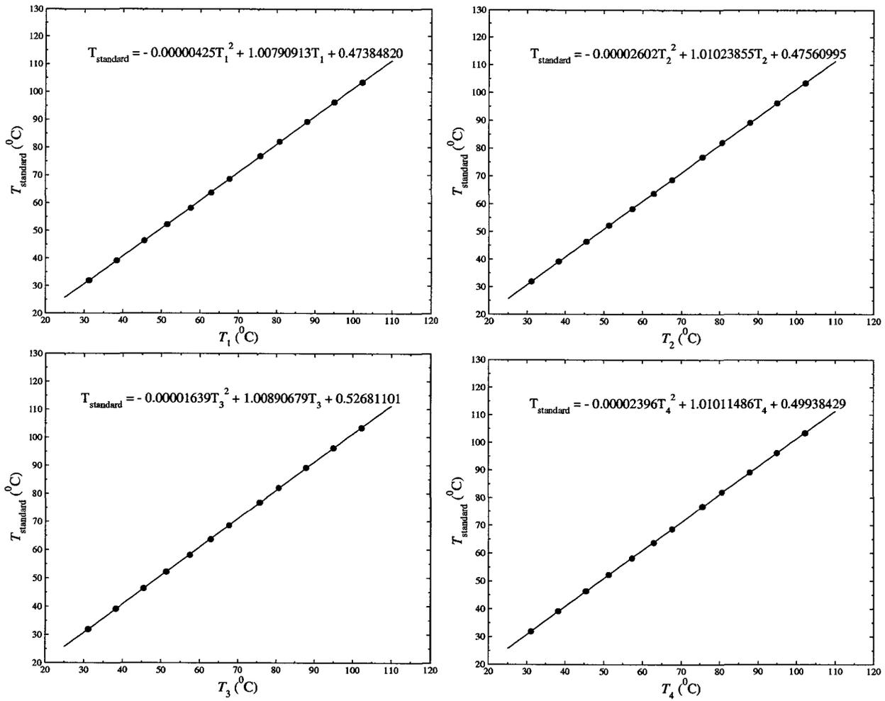
Figure 3.10: Polynomial regression curve-fittings of the four thermocouple probes.
