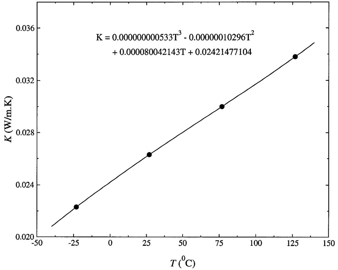
Figure 3.8: Polynomial regression curve-fitting of air thermal conductivity.
