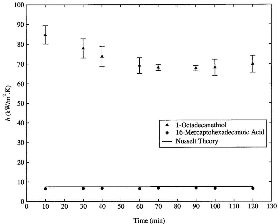
Figure 4.1: Condensation heat transfer coefficient of SAMs on evaporated Au/Ti/Cu substrates as a function of time during steam condensation at standard atmosphere pressure. Steam velocity passing through the condensing surface is  $\sim 6$  m/s and heat flux is  $\sim 280$  kW/m<sup>2</sup>.
