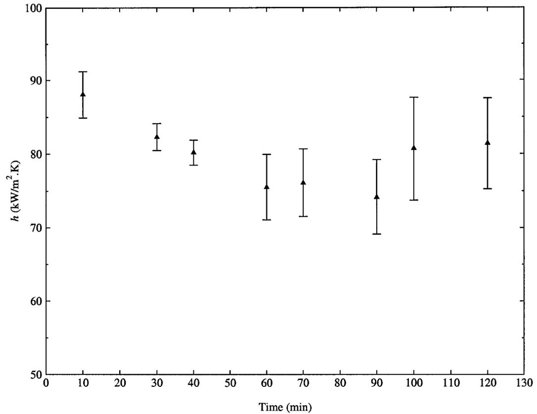
Figure 4.8: Heat transfer coefficient as a function of condensation duration for heat flux  $q'' \approx 360 \text{ kW/m}^2$ . Error bars are 95% confidence limits.
