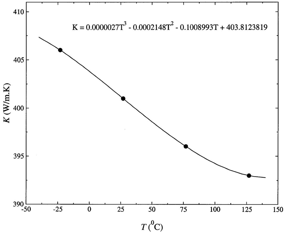
Figure 3.7: Polynomial regression curve-fitting of copper thermal conductivity.
