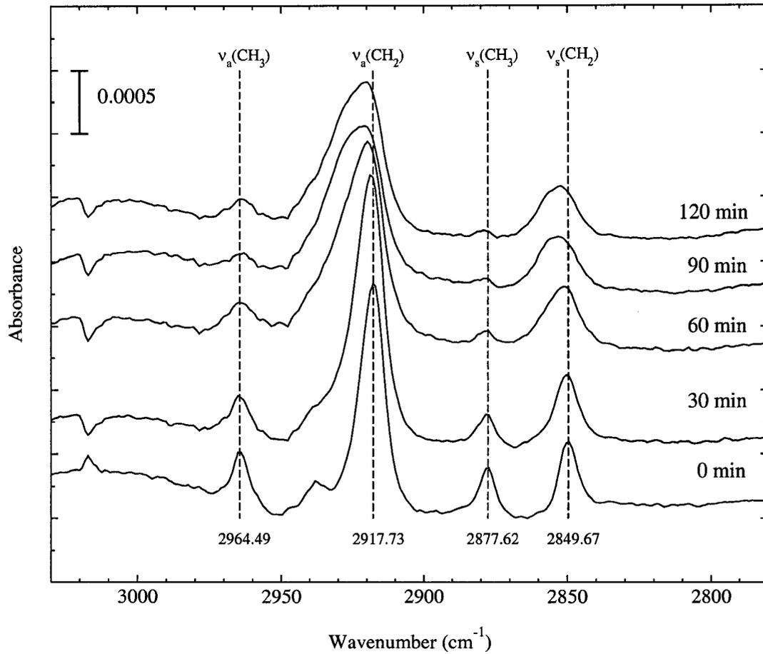
Figure 4.13: Reflectance FT-IR spectra for SAMs derived from 1-octadecanethiol on Au/Ti/Cu substrates subjected to steam condensation in various duration ( $q'' \approx 400 \text{ kW/m}^2$ ). The dashed lines represent the positions of the original modes for a trans-extended monolayer. The spectra have been offset for clarity.
