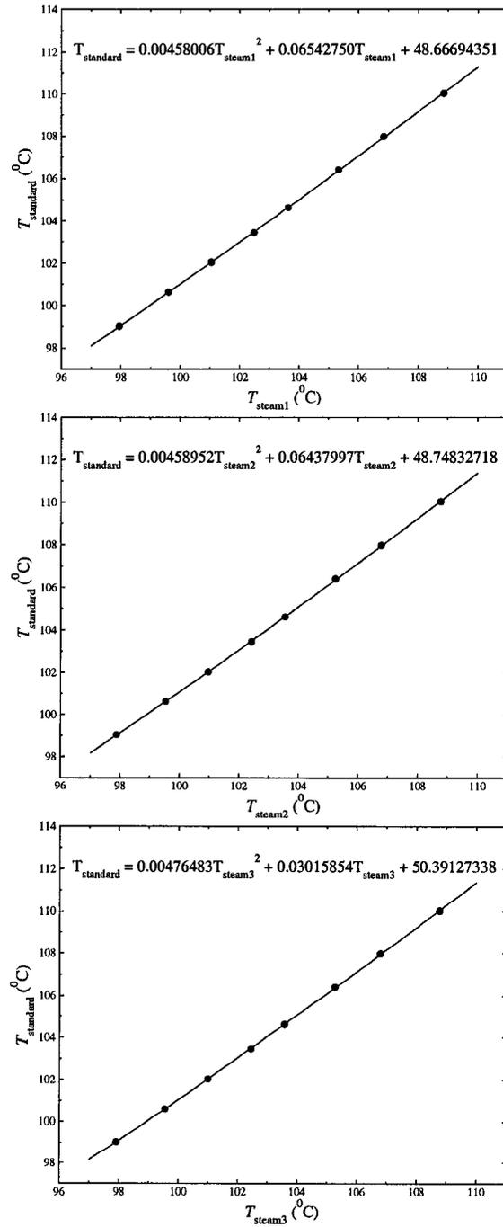
Figure 3.11: Polynomial regression curve-fittings of the three thermocouple wires.
