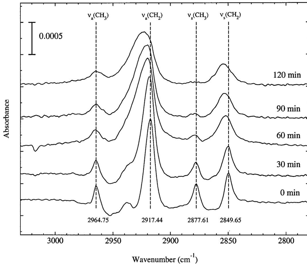
Figure 4.11: Reflectance FT-IR spectra for SAMs derived from 1-octadecanethiol on Au/Ti/Cu substrates subjected to steam condensation in various duration ( $q'' \approx 320 \text{ kW/m}^2$ ). The dashed lines represent the positions of the original modes for a trans-extended monolayer. The spectra have been offset for clarity.
