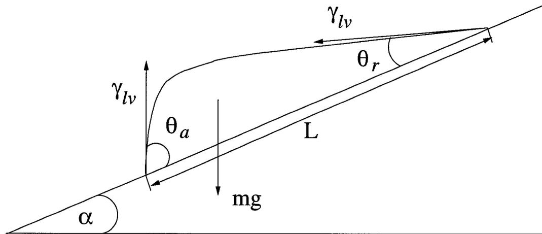
Figure 3.2: Profile of a drop on an inclined surface.
