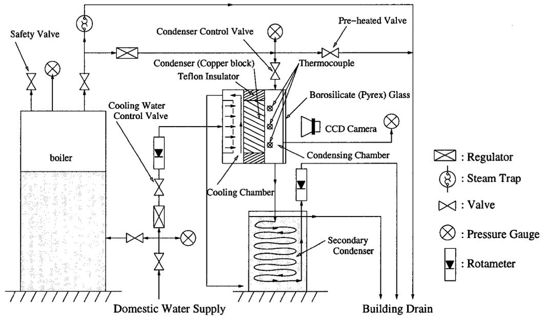
Figure 3.4: Schematic of an experimental set-up for the measurements of the condensation heat transfer coefficient.
