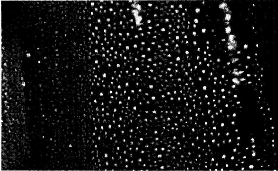
Figure 4.2: Dropwise condensation of steam on self-assembled monolayers (SAMs) derived from 1-octadecanethiol [ $\text{HS}(\text{CH}_2)_{17}\text{CH}_3$ ] onto gold-coated-copper substrates.
