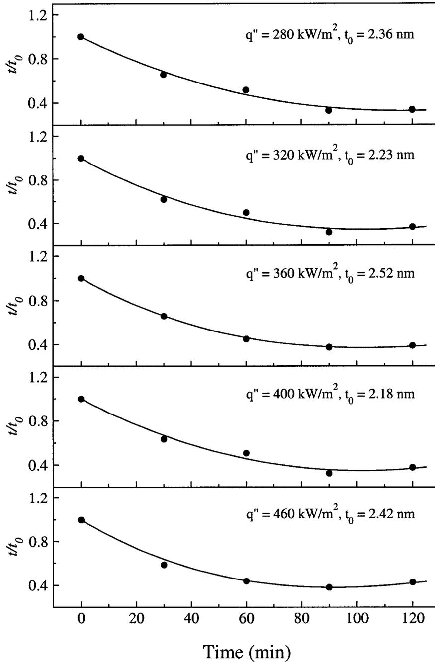
Figure 4.15: Normalized thickness of SAMs derived from 1-octadecanethiol on Au/Ti/Cu substrates as a function of condensation duration for different heat fluxes.  $t_0$  is the initial film thickness reference.
