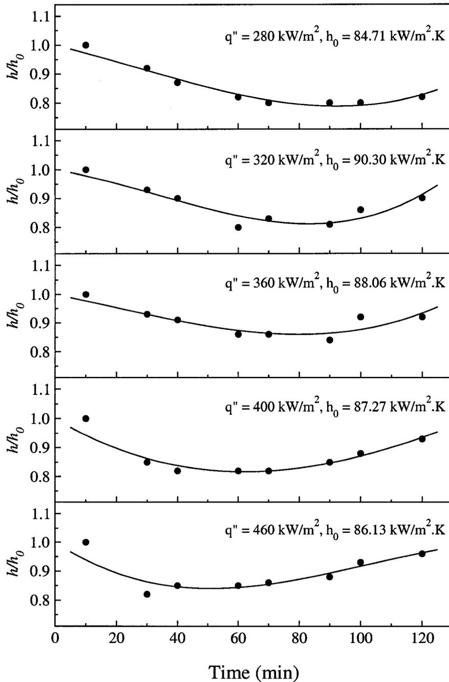
Figure 4.16: Normalized heat transfer coefficient of SAMs derived from 1-octadecanethiol on Au/Ti/Cu substrates as a function of condensation duration for different heat fluxes.  $h_0$  is the heat transfer coefficient after 10 minute condensation.
