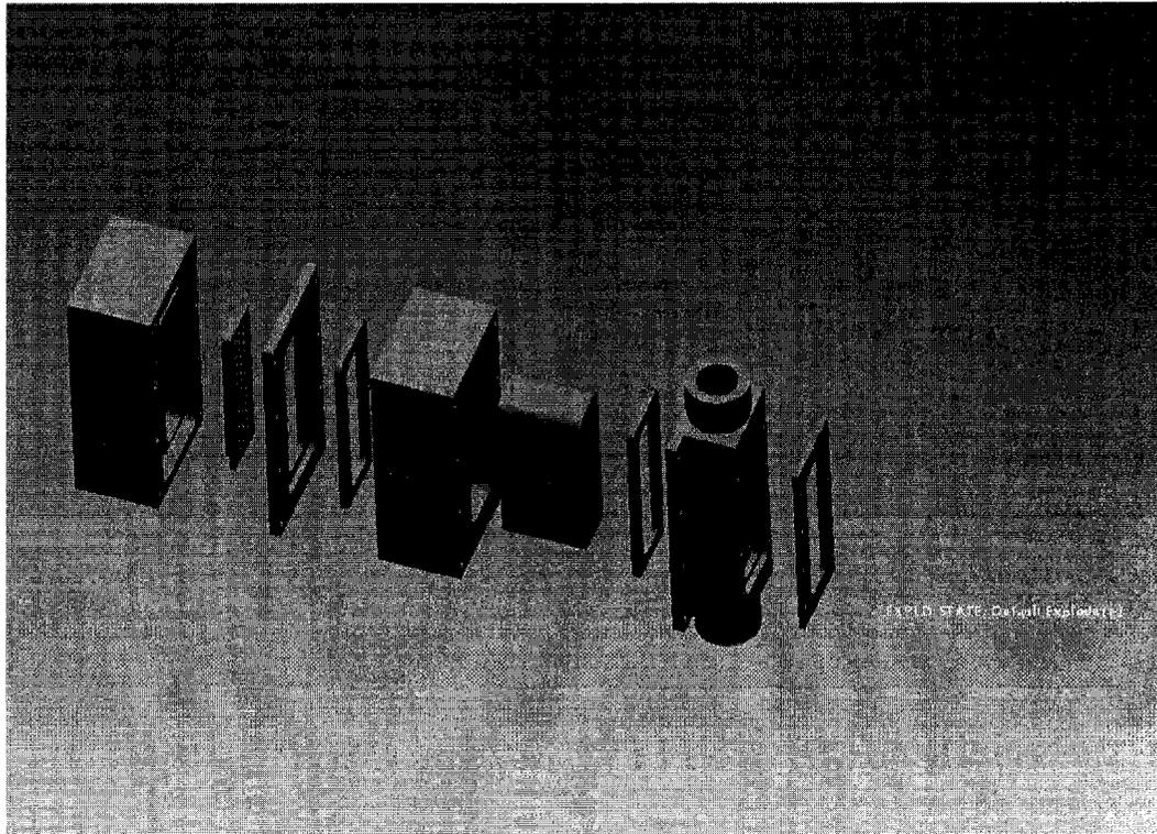
Figure 3.5: An exploded view of the condensation test assembly.
