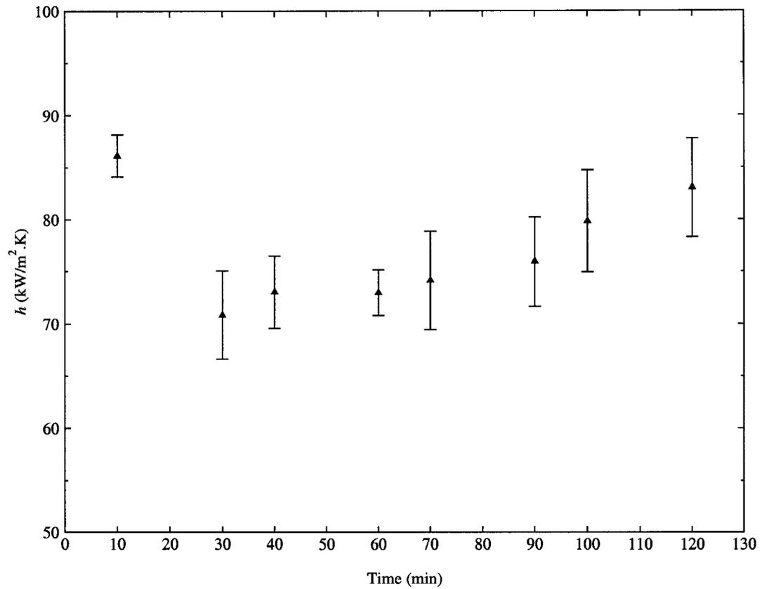
Figure 4.10: Heat transfer coefficient as a function of condensation duration for heat flux  $q'' \approx 460 \text{ kW/m}^2$ . Error bars are 95% confidence limits.
