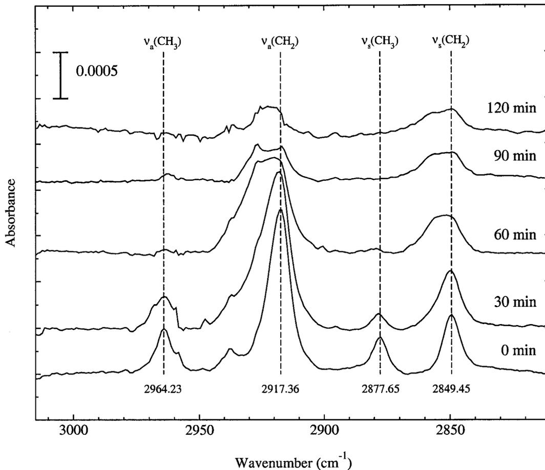
Figure 4.14: Reflectance FT-IR spectra for SAMs derived from 1-octadecanethiol on Au/Ti/Cu substrates subjected to steam condensation in various duration ( $q'' \approx 460 \text{ kW/m}^2$ ). The dashed lines represent the positions of the original modes for a trans-extended monolayer. The spectra have been offset for clarity.
