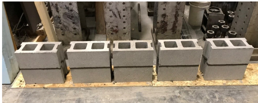
Figure 3.9 – 2 Course Hollow Masonry Prisms
