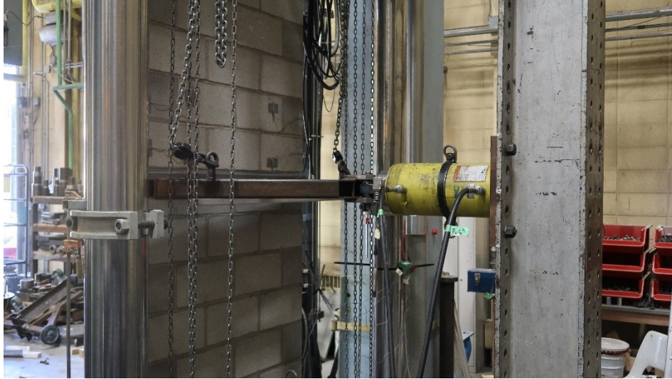
Figure 3.18 – Lateral Load Application
