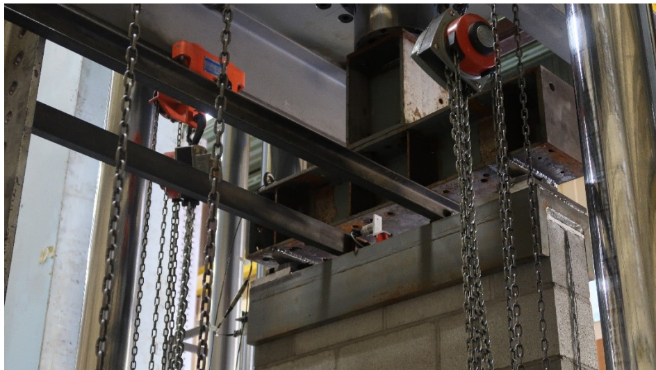
Figure 3.14 – Bottom Lateral Bracing Fixture
