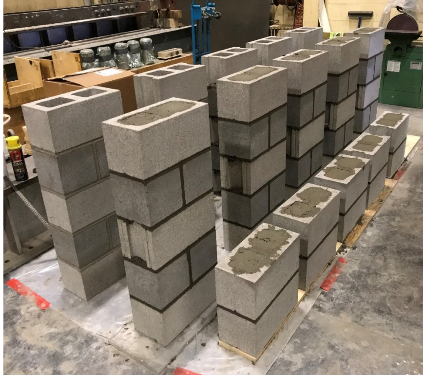
Figure 3.8 – 5-Course (Hollow and Grouted) and 2-Course Grouted Masonry Prisms
