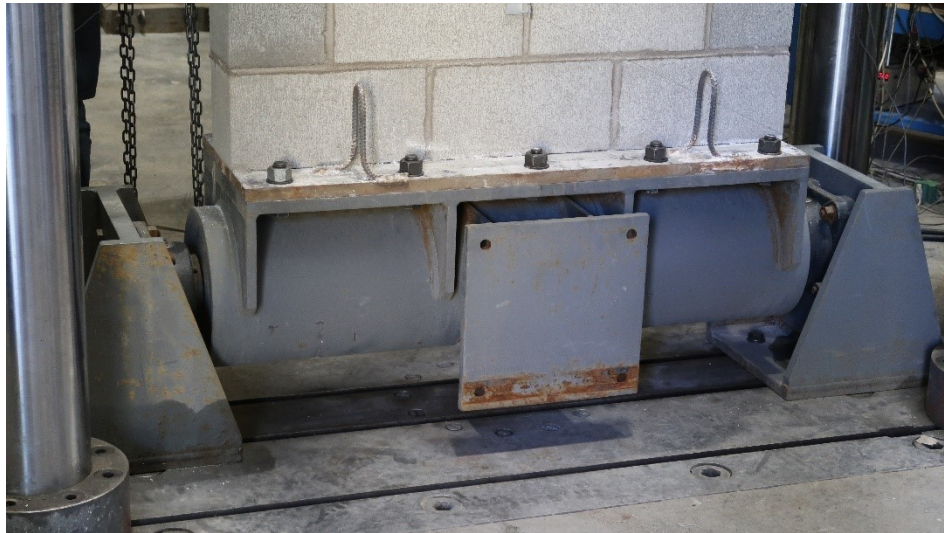
Figure 3.14 – Bottom Lateral Bracing Fixture
