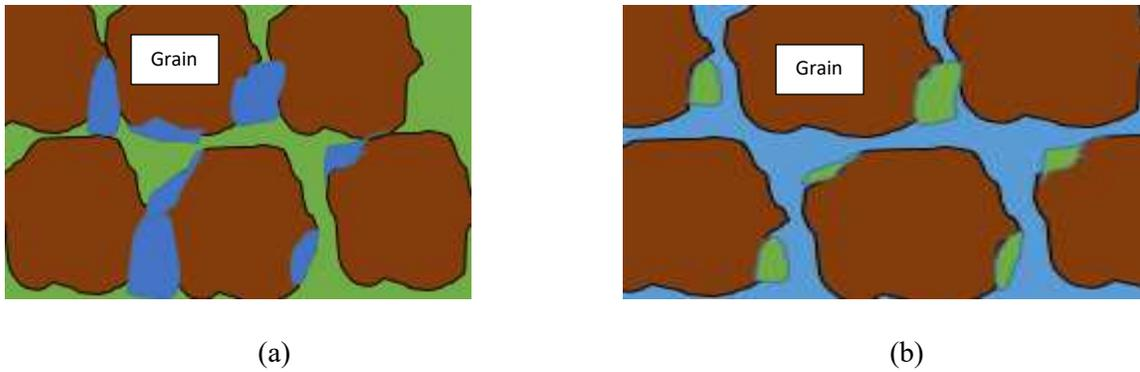
Figure 1 - Schematics of (a) oil-wet and (b) water-wet states of wettability on a microscopic level.
