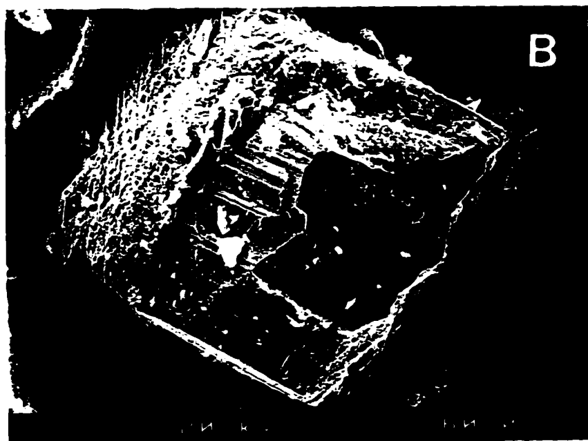
Fig. 3.1.6 Scanning electron micrographs of heat treated gels: a) \text{GeO}_2 crystal in 1A; b) \text{GeO}_2 crystal in 1B;
