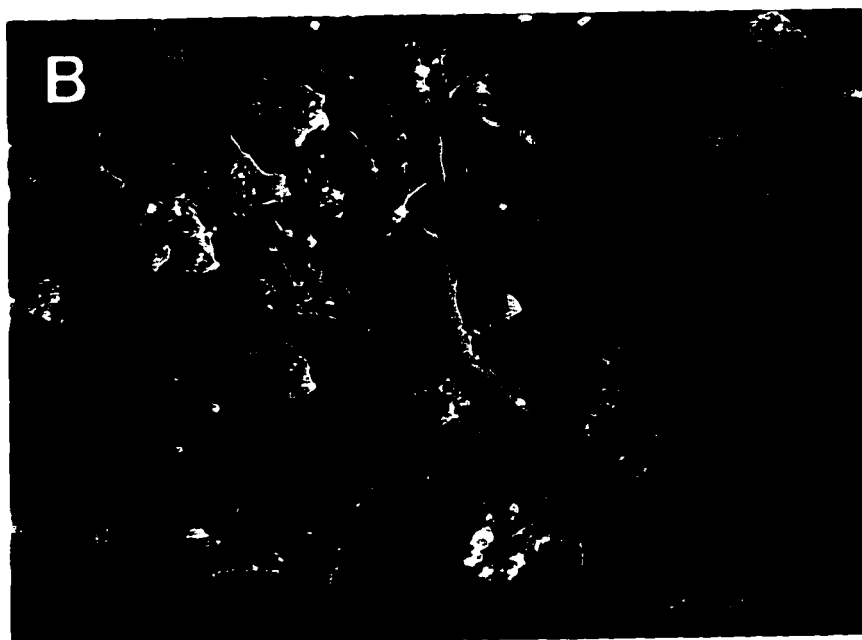
Fig. 3.2.3 Scanning electron micrographs of: a) gel \text{GeS}_x\text{-GeO}_x ; b) sulfur crystals deposited in the gel;
