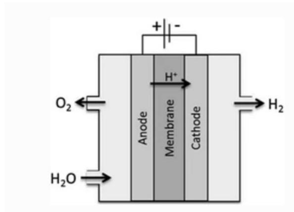
Figure 4 Setup of a Proton Exchange Membrane Electrolyzer, Source (Lehner et al. 2014)
