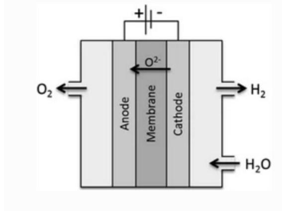
Figure 5 Setup of a Solid Oxide Electrolyzer, Source (Lehner et al. 2014)
