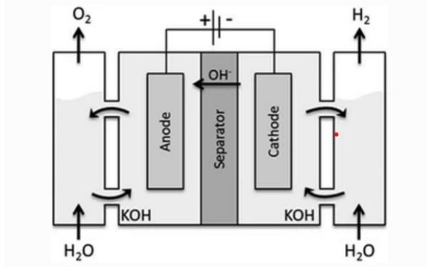
Figure 3 Setup of an Alkaline Electrolyzer, Source (Lehner et al. 2014)
