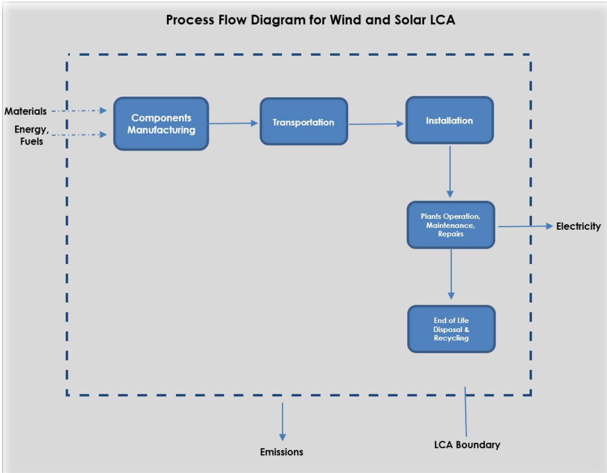
Figure 1: Process Flow Diagram for Wind and Solar LCA
