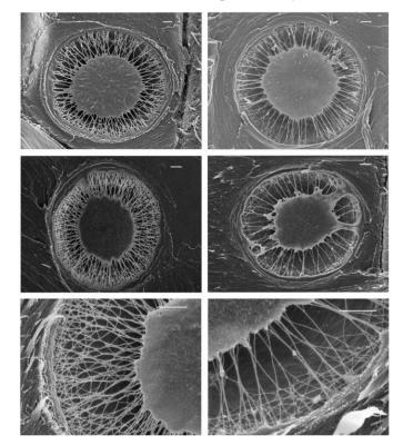
Top two images show typical bordered pit structures of open (left) and understory grown (right) lodgepole pine; Middle images show open (left) and understory grown (right) black spruce, bottom images are a close-up views of the margo (the filamentous zone where water passes through). White bar represents 1  $\mu$ m.
