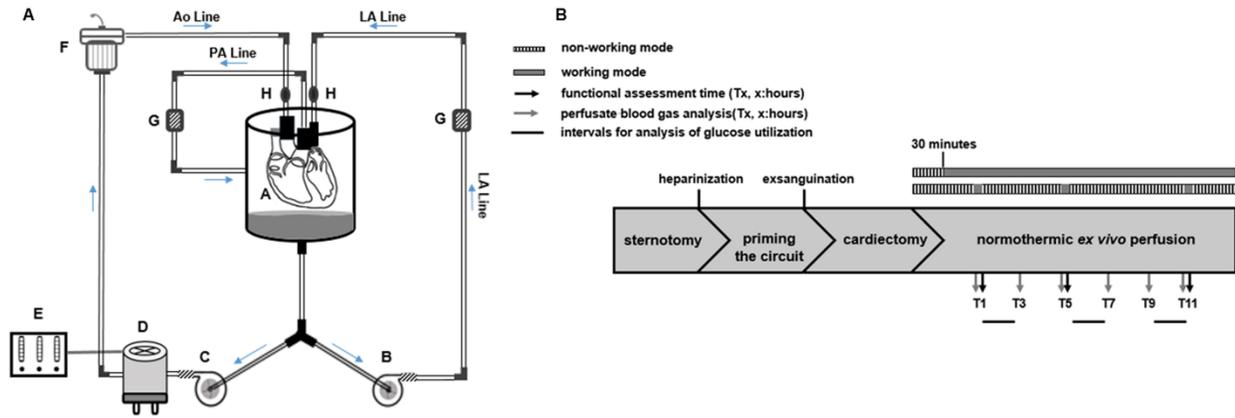
T(x); x-hours after the start of the perfusion; A, venous reservoir; B, left atrial pump; C, Aortic pump; oxygenator/heat exchanger; D, oxygen/heat exchanger; E, medical gas mixer; F, leukocyte filter; G, Flow sensor; H, Pressure sensor; Ao, Aorta; LA, left atrium; PA, pulmonary artery.
