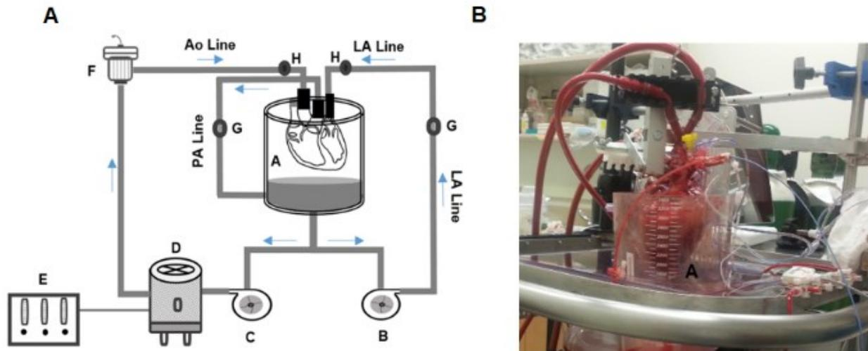
A, venous reservoir; B, left atrial pump; C, Aortic pump; D, oxygen/heat exchanger; E, medical gas mixer; F, leukocyte filter; G, Flow sensor; H, Pressure sensor; Ao, Aorta; LA, left atrium; PA, pulmonary artery.
