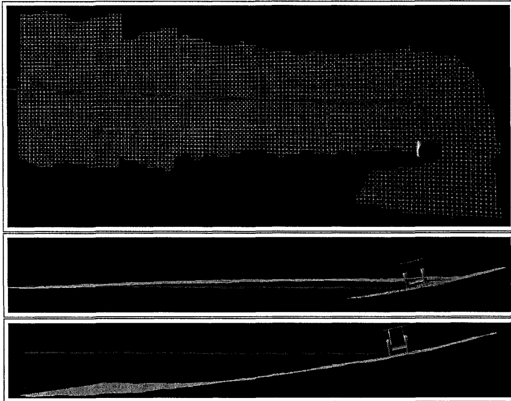
Figure 4.6: The significant difference estimating z can make on the terrain map is shown here. These three images are obtained from teleoperating the robot straight up a hill then turning right. The top image is a birds eye view of the terrain map, the purple line indicates the robot's trail. The other two images show the same grid except from the side, note that the entire trail is drawn at the current z -value of the robot. The middle image shows the grid obtained when the z was assumed to be zero and the bottom image is obtained when z was estimated.
