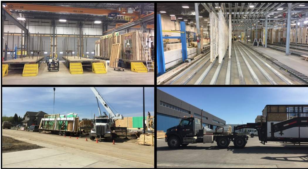
Figure 43 Panelized construction facility and operations (courtesy of ACQBUILT, Inc.)
