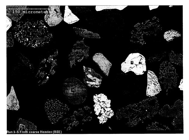
Figure 31: Typical backscattered SEM image from primary froth heavies.
