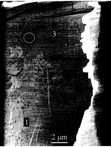
Figure 39: HAADF- STEM image of "leucoxene" particle showing three distinct regions. The dark spots shown in the micrograph are pores while the bright streaks are areas that were found to be rich in iron (FEI Tecnai F20).
