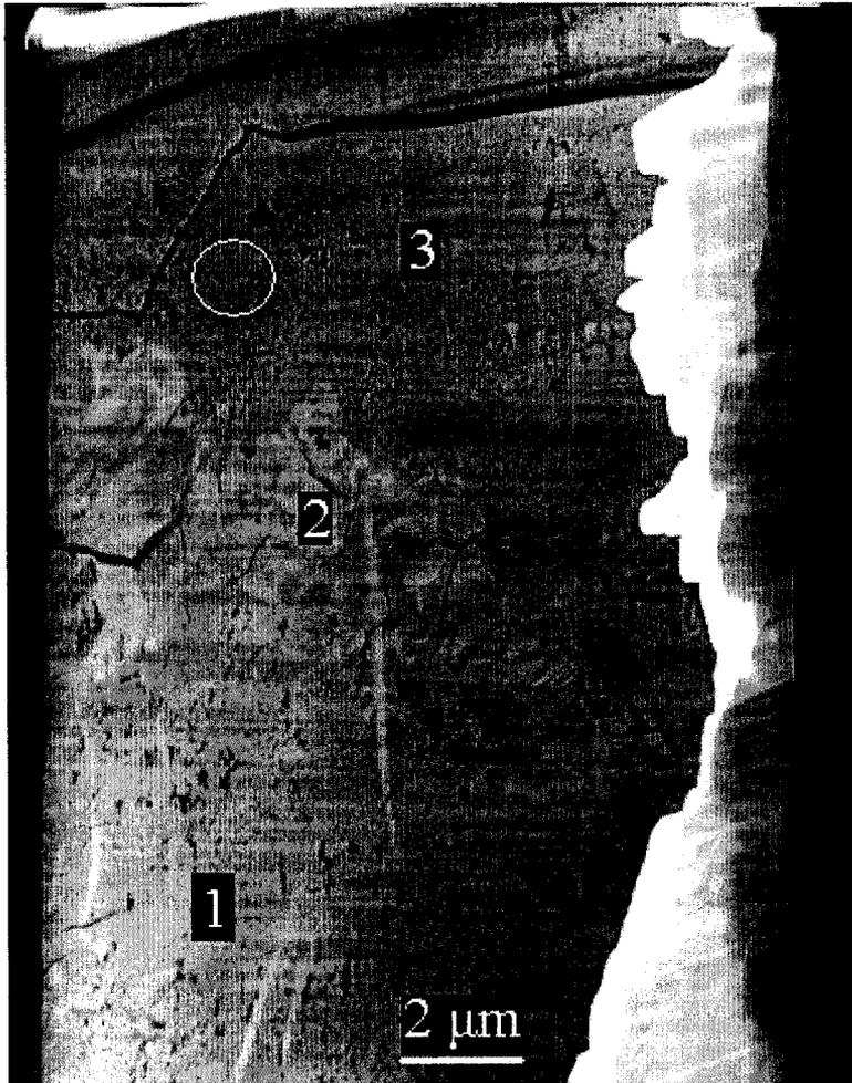
**Figure 39: HAADF- STEM image of “leucoxene” particle showing three distinct regions. The dark spots shown in the micrograph are pores while the bright streaks are areas that were found to be rich in iron (FEI Tecnai F20).**
