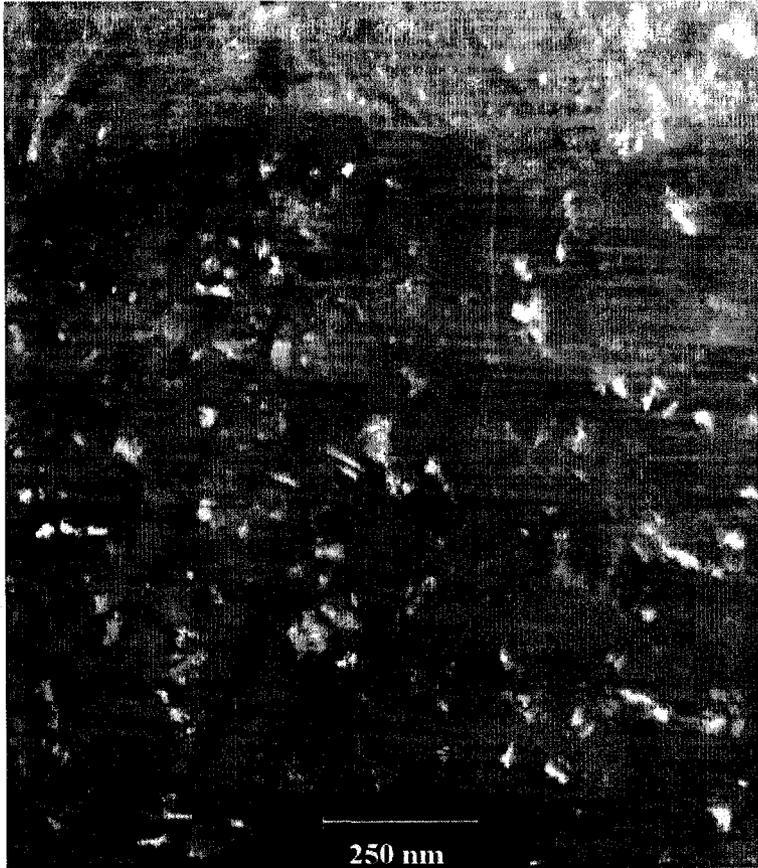
**Figure 49: Dark field image showing TiO particles (bright) in anatase matrix (FEI Tecnai F20).**
