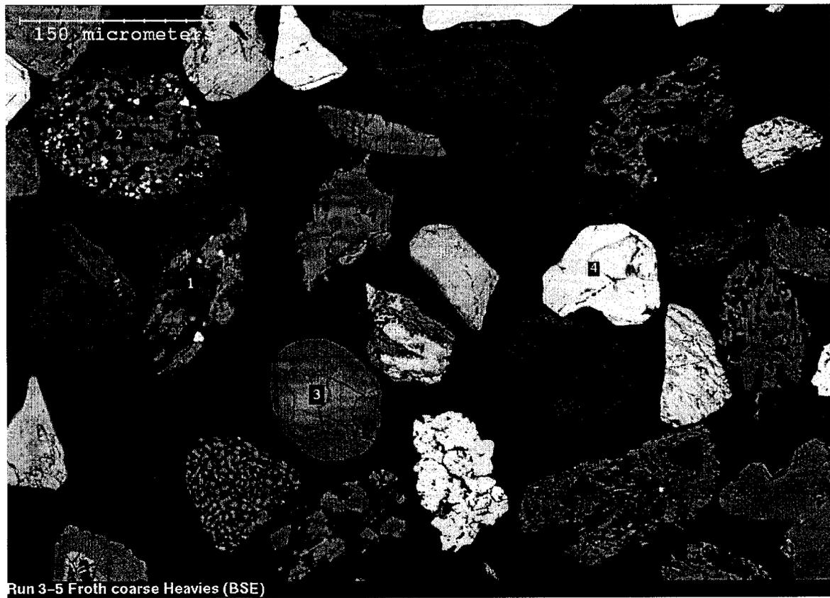
Figure 31: Typical backscattered SEM image from primary froth heavies.
