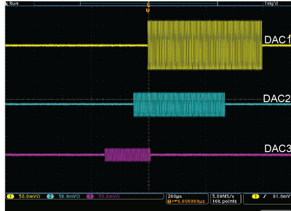
d) Waveforms generation with an aliasing issue
