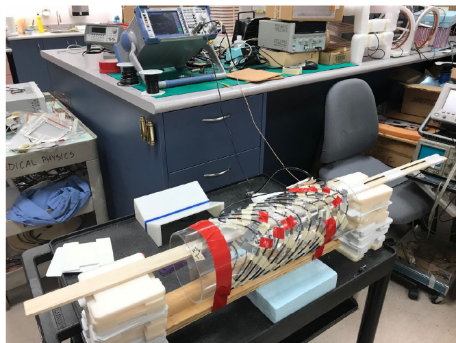
Figure 4.7: Photos of constructed small pick-up coil and the experimental setup for the measurements of B_1 field components B_x and B_y .
