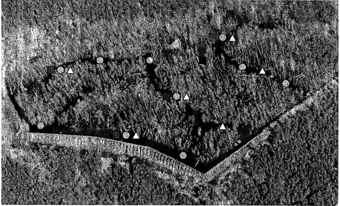
Figure 2.1: Aerial view of the reservoir three years after flooding (photograph: J. Shearer, Freshwater Institute, Winnipeg). Yellow circles represent dissolved \text{SF}_6 sampling sites; red squares, dissolved \text{CO}_2 and \text{CH}_4 sampling sites; white triangles, FC positions; and blue square, anemometer position.
