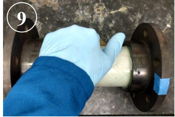
Figure 67-1 to Figure 67-9: Procedure for strain gauge application
