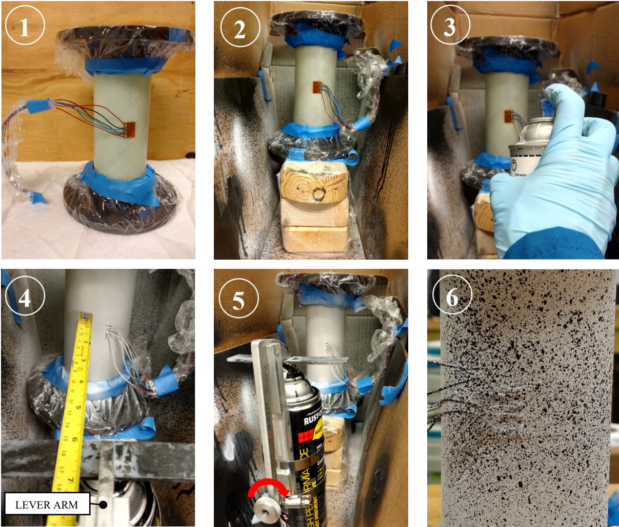
Figure 70-1 to Figure 70-6: Procedure for applying speckle pattern
