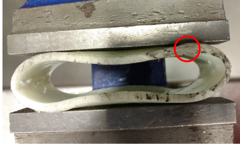
Figure 32: Crush test to check bond quality
