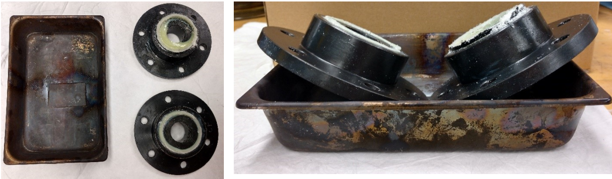
Figure 80: Placement of end fittings for epoxy burnout
