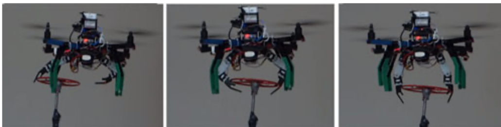
Figure 1.2: Quadrotor UAV Autonomous Valve Interfacing Task [36]
