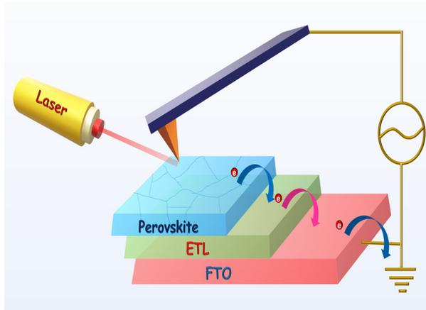
**Fig. S4.** Schematic illustration of KPFM measurement setup.
