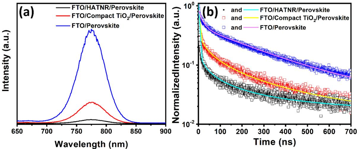
**Fig. 5.** (a) Steady state photoluminescence (PL) spectra of glass/perovskite (blue), perovskite deposited over compact  $\text{TiO}_2$  (red) and perovskite/HATNR array (black); (b) The PL lifetime decay curve of perovskite with no ETL (blue; double exponential fit, magenta line), compact  $\text{TiO}_2$  (red; double exponential fit, yellow line) and perovskite/HATNR array (black, double exponential fit, cyan).
