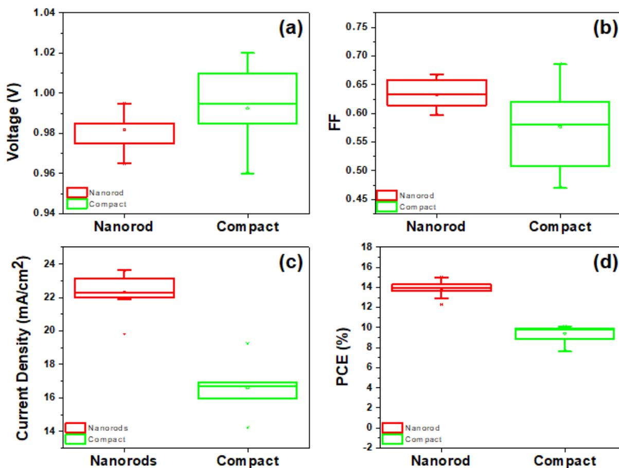
**Fig. S6.** Summary of the performance of halide perovskite solar cells for compact TiO<sub>2</sub> and HATNR morphologies: (a)  $V_{oc}$ , (b) FF, (c)  $J_{sc}$ , and (d) PCE. All the performance data were measured at AM 1.5G.
