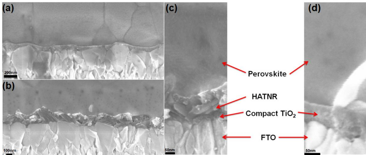
**Fig. S2.** High resolution FESEM images showing cross-sectional view of a perovskite solar cell (with different magnification) made with compact  $\text{TiO}_2$  layer (a) and (d) HATNRs (b) and (c).
