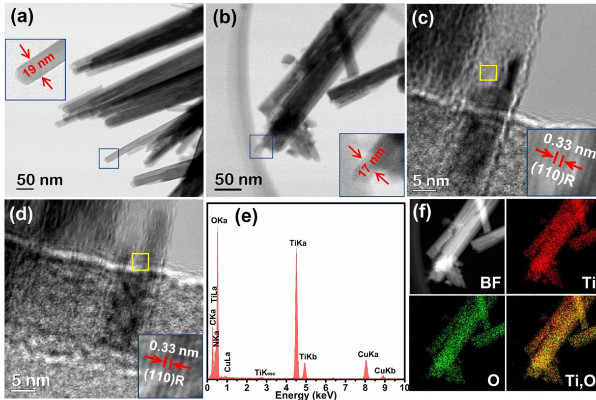
**Fig. 2.** (a, b) HR-TEM images HATNRs images at 50 nm scale bar showing bundles of nanorods and inset showing individual nanorods and their respective diameter (c, d) high magnification images at 5 nm scale bar showing lattice fringes (e) EDX pattern showing presence of Ti and O and (f) Bright field image and EDX elemental mapping for Ti, O and their summed-up image.
