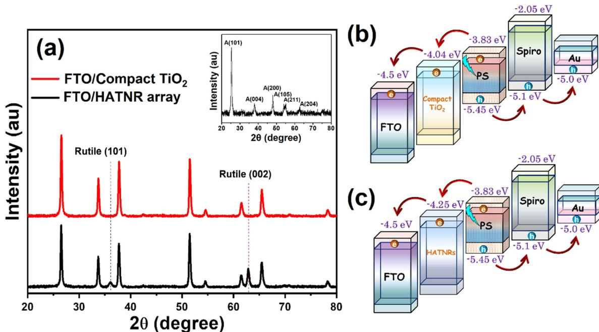
**Fig. 4.** (a) X-ray diffractograms of compact TiO<sub>2</sub> (red) and HATNR array (black) on FTO substrate. Inset shows XRD pattern of compact TiO<sub>2</sub> on bare glass substrate. Energy band diagram of perovskite solar cells made with (b) Compact TiO<sub>2</sub> and (c) HATNR arrays.
