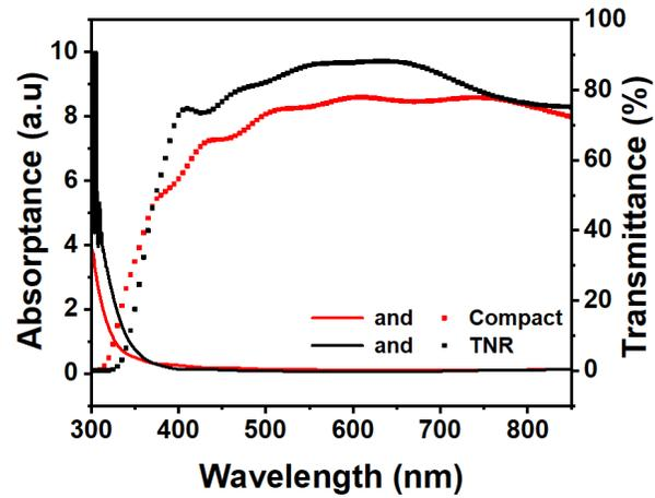
**Fig. S1.** Absorbance and transmittance spectra of compact  $\text{TiO}_2$  and HATNR array deposited over FTO substrate.
