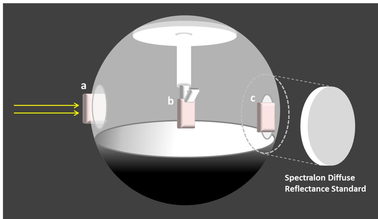
**Fig. S8.** Schematic illustration of the integrating sphere accessory used for UV-Vis-NIR spectroscopic measurements, and the placement of samples corresponding to different configurations. ‘a’, ‘b’ and ‘c’ refer to different possible sample positions, fully explained in section S 1.2.
