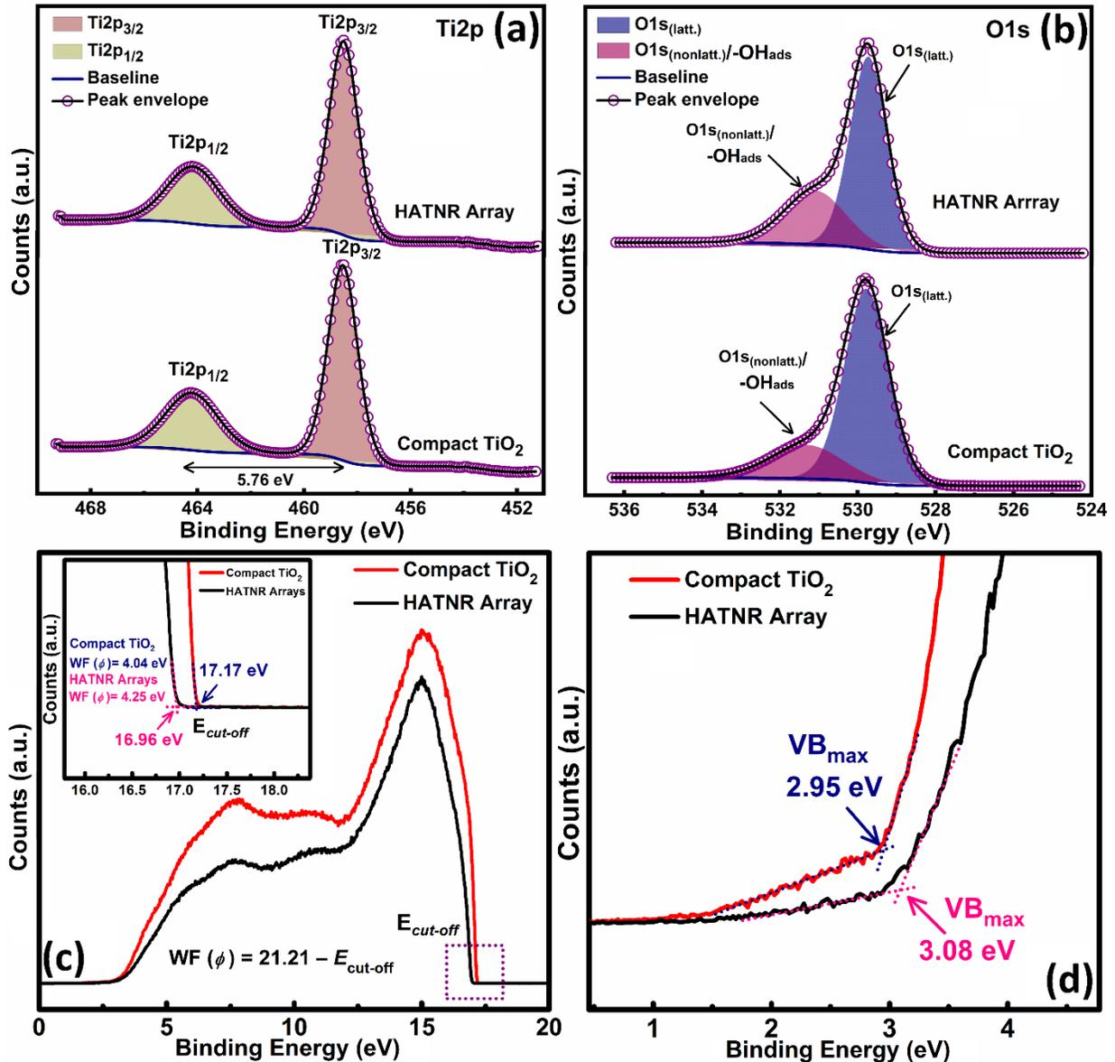
**Fig. 3.** HR XPS spectra of compact TiO<sub>2</sub> and HATNR array in (a) Ti2p region and (b) O1s region; (c) UPS work function spectra of compact TiO<sub>2</sub> and HATNR array. Inset shows the secondary electron cut-off energy ( $E_{cut-off}$ ) while the value of work function (WF) was determined using the equation,  $WF(\phi) = 21.21 - E_{cut-off}$ ,
