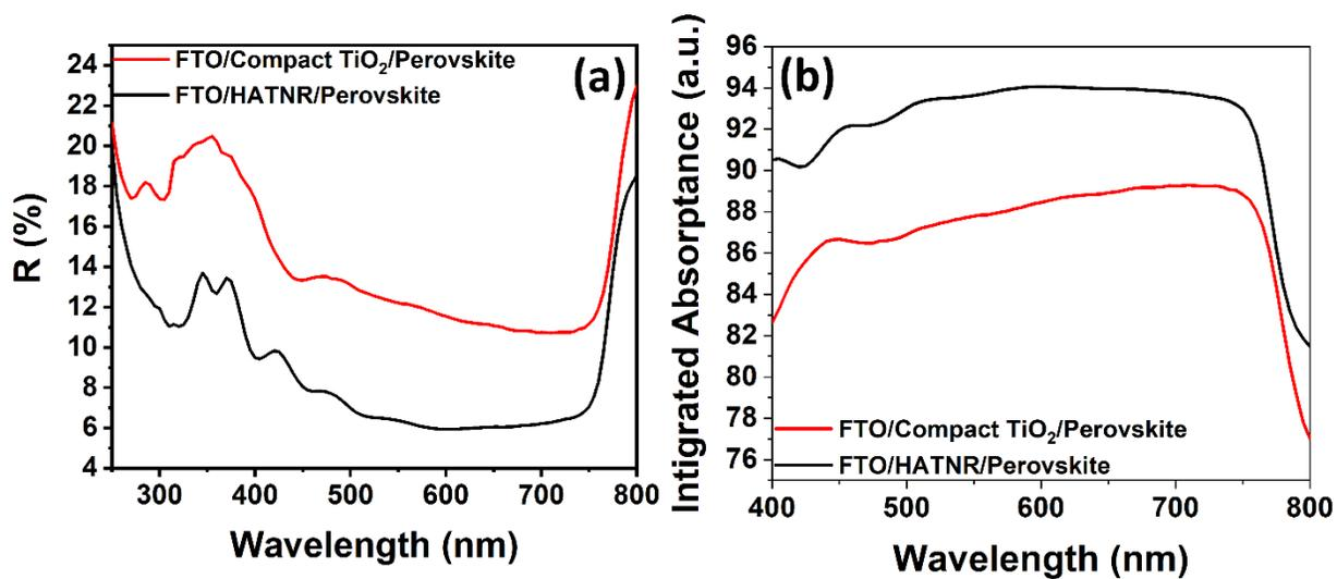
**Fig. S9.** UV-Vis spectra showing diffuse reflectance (a) and integrated absorbance (b) measured from samples consisting of perovskite layers deposited over compact TiO<sub>2</sub> ETL (red) and HATNR ETL (black) on FTO substrate.
