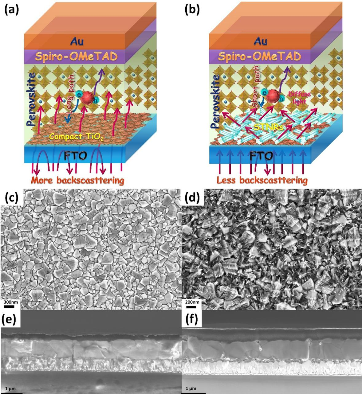
**Fig. 1.** Graphical representation of perovskite solar cells made with (a) Compact  $\text{TiO}_2$  and (b) Nanostructured HATNRs obtained by hydrothermal method; Topographic FESEM image of (c) compact and (d) HATNRs. Cross-sectional view of a perovskite solar cell made with (e) Compact  $\text{TiO}_2$  layer and (f) HATNR arrays.
