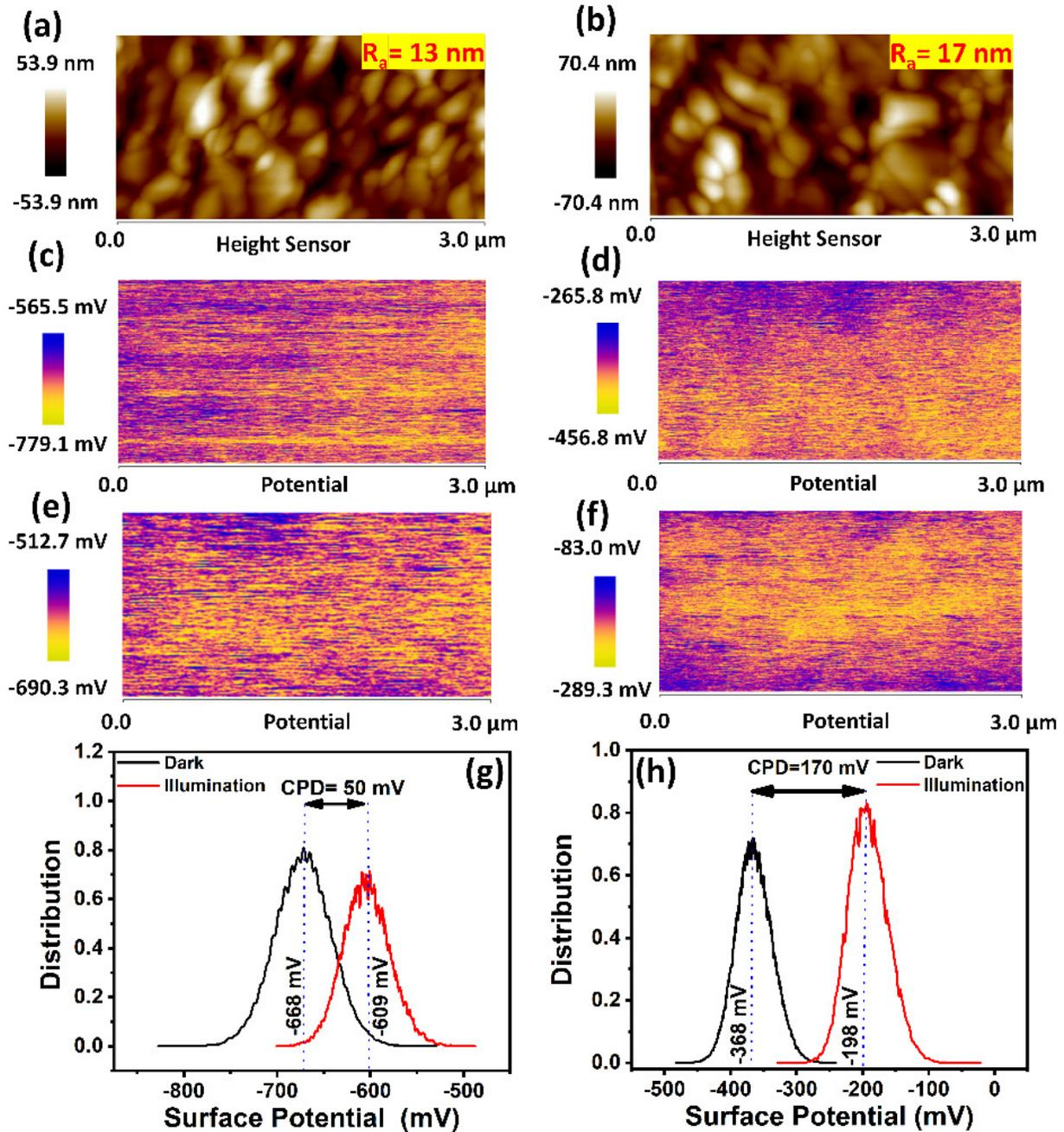
**Fig. 6.** Topography of perovskite layer deposited over compact TiO<sub>2</sub> (a) and HATNR (b). Surface potential map of perovskite deposited over compact TiO<sub>2</sub> (c) and HATNR (d) in dark. Surface potential map of perovskite deposited over compact TiO<sub>2</sub> (e) and HATNR (f) under illumination with 450 nm laser. Surface potential distribution on perovskite layer deposited over (g) compact TiO<sub>2</sub> and (h) HATNR in dark and under illumination with 450 nm laser.
