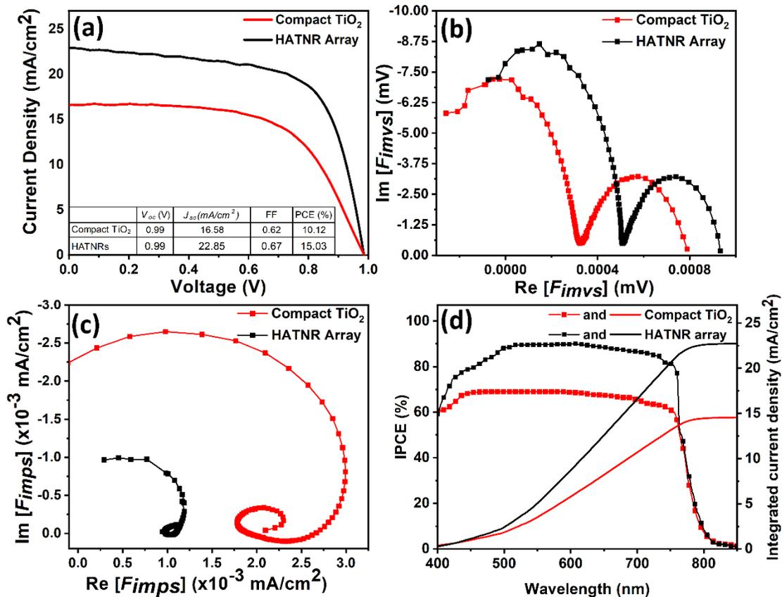
**Fig. 7.** Current density–voltage (*J-V*) curves measured under AM 1.5G condition (a), IMVS Nyquist plots measured with 633nm LED (b), IMPS Nyquist plots measured with 633nm LED (c) and external quantum yield of best-performing perovskite solar cells based on compact TiO<sub>2</sub> (red) and HATNR (black) electron transporting layers (d).
