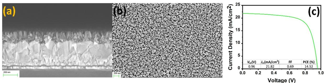
**Fig. S5.** Cross-sectional view (a), top view (b) of vertically oriented TiO<sub>2</sub> nanorods. Current density–voltage ( $J$ - $V$ ) curve (c) of perovskite solar cells made with vertically oriented nanorods measured under AM 1.5G condition.
