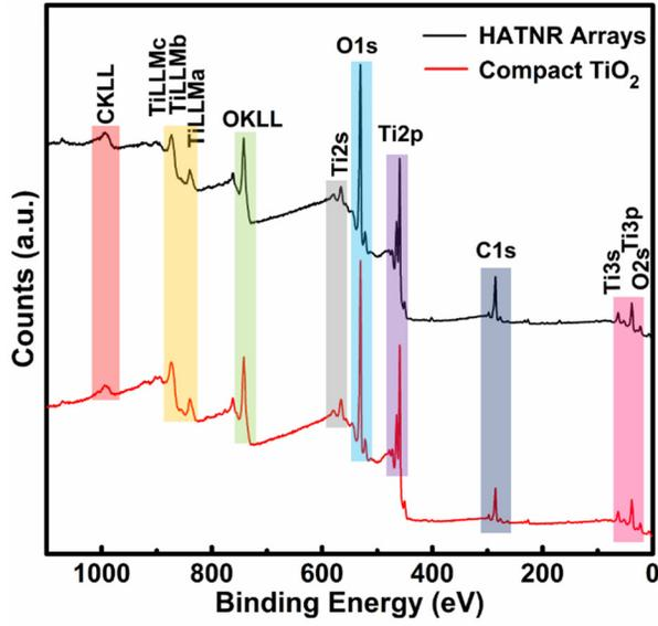
**Fig. S3.** XPS elemental survey scan of compact TiO<sub>2</sub> (red) and HATNR arrays (black).
