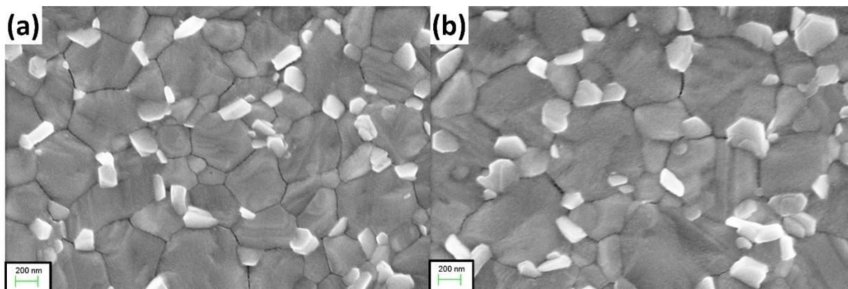
**Fig. S10.** FE-SEM topographic image of perovskite layer deposited over (a) Compact  $\text{TiO}_2$  layer and (b) HATNR arrays.
