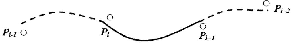
Figure 3.6: B-spline approximation between two control points  $P_i$  and  $P_{i+1}$ .
