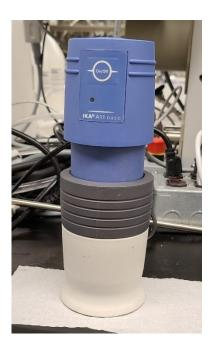
Figure C.1 Grinder used for milling POS
