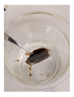
Figure C.3 Final mat-like gelled-oil at the end of the oil removal experiments of diluted bitumen using POS. SOR of 1:8, 3 h.
