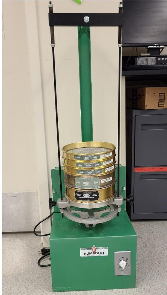
**Figure C.2** Mechanical sieve shaker machine with different sieve mesh sizes (45, 250, 500, 850, 1000  $\mu$ ).
