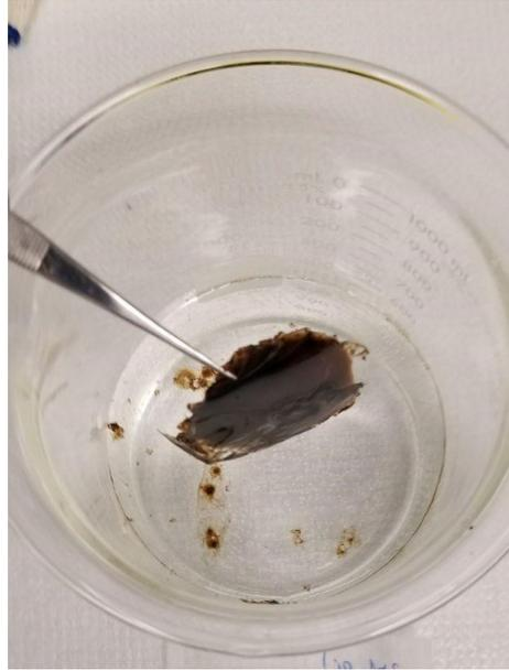
**Figure C.3** Final mat-like gelled-oil at the end of the oil removal experiments of diluted bitumen using POS. SOR of 1:8, 3 h.
