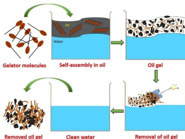
**Figure 1.8** Schematic representation of oil spill containment using LMWO. [4]
