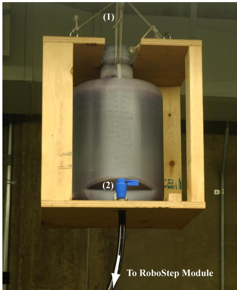
Figure 3.10 The dye reservoir, and dye reservoir support frame. The frame connects to a cable winch at location (1), and the flow can be controlled by the valve at (2).
