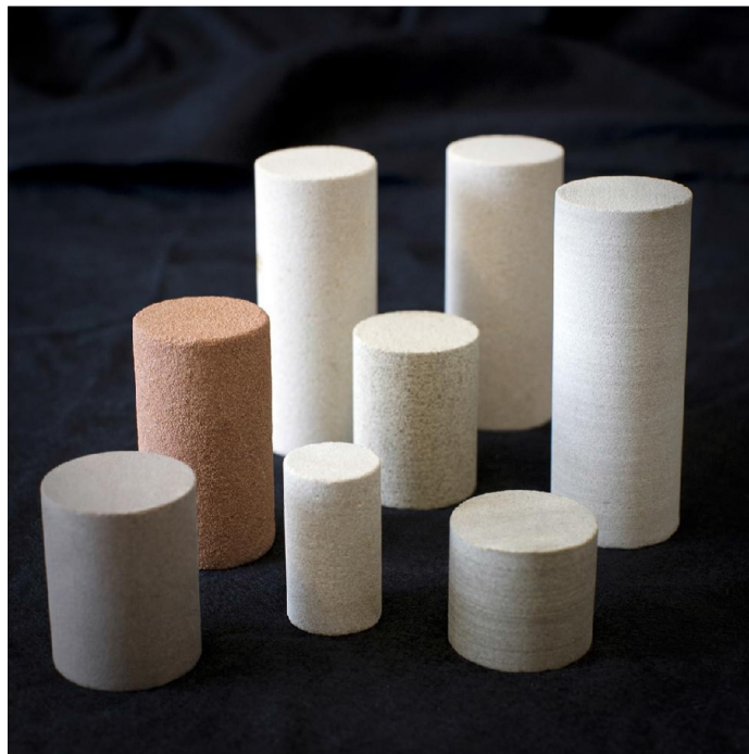
Figure 1.1.1: Photograph of multiple rock cores showing variation in texture and color depending on where the sample was extracted [4].
