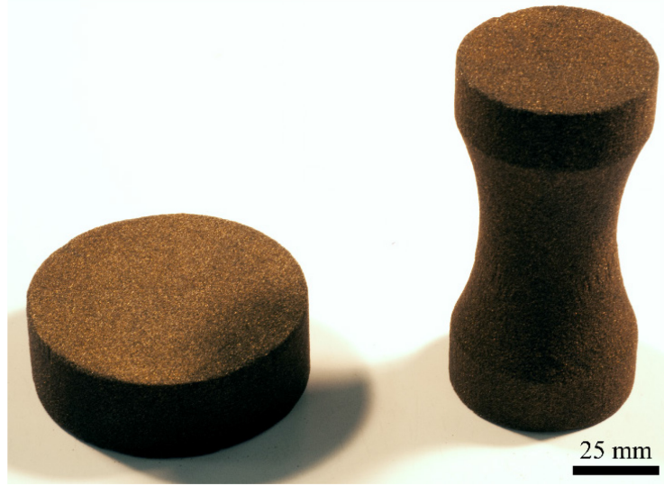
Figure 2.1.2: A photograph of a 3D-printed shear sample and tensile specimen, from left to right respectively, fabricated via the M-Flex Sand Printer.
