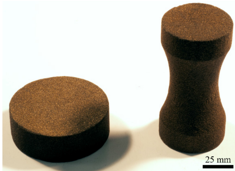
Figure 3.2.2: Photograph of 3D-printed samples fabricated on the M-Flex sand printer.
