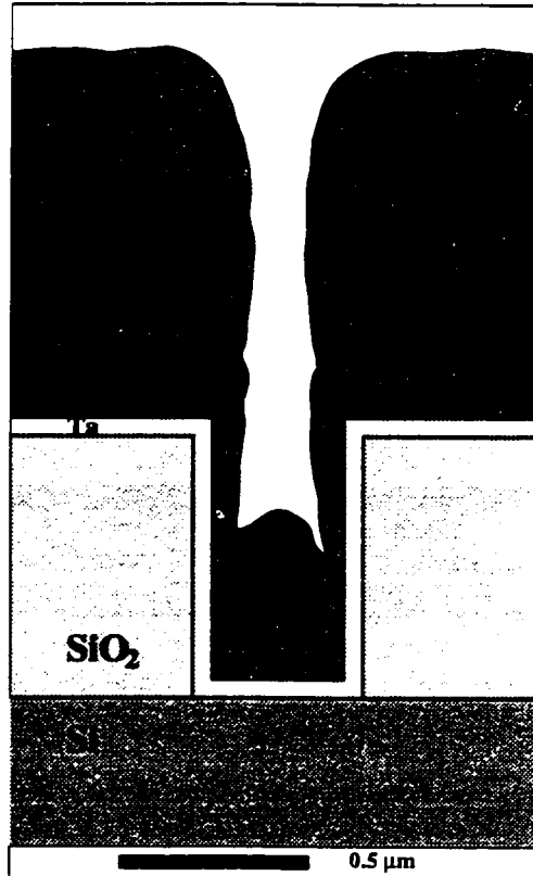
Figure 5.24 The original deposition profile without any microstructure. This simulation is used as the starting point for each of the following reflow simulations where the grain boundaries are arbitrarily added one at a time.
