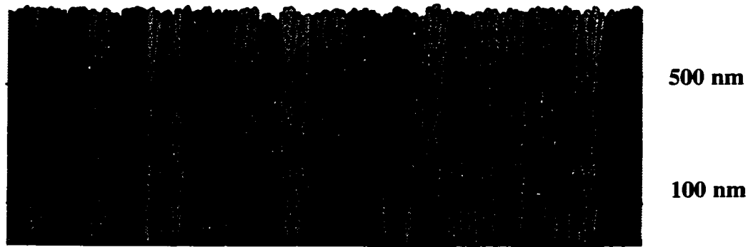
Figure 4.9 GROFILMS simulation of a thin film with possible Zone I microstructure. Many voids exist between the columns though not visible at the current resolution.
