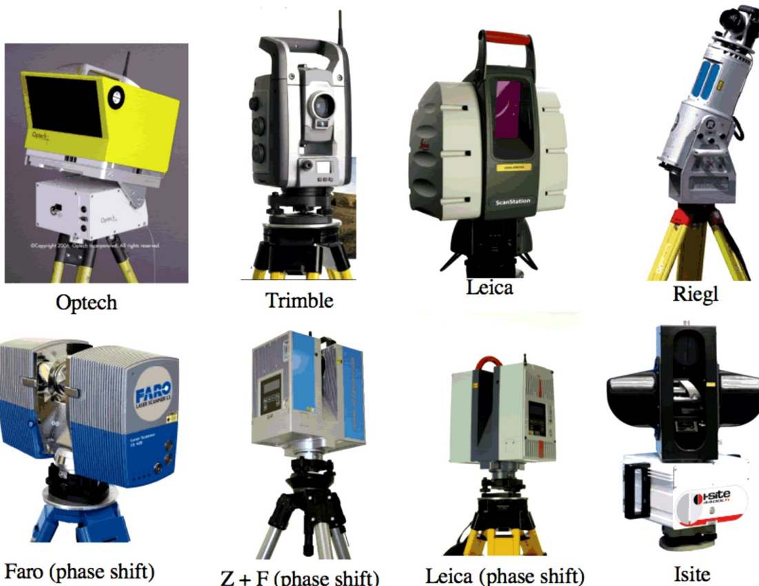
Figure A-1 Terrestrial laser scanners (Kemeny & Turner, 2008)
