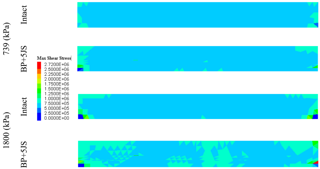
Figure 6-24 Shear stresses (Pa) developed in confined caprock models
