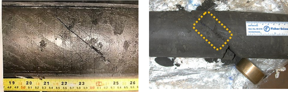
Figure 8-3 Laboratory core logging and specimen (S3) extraction with circular steel cutting ring
