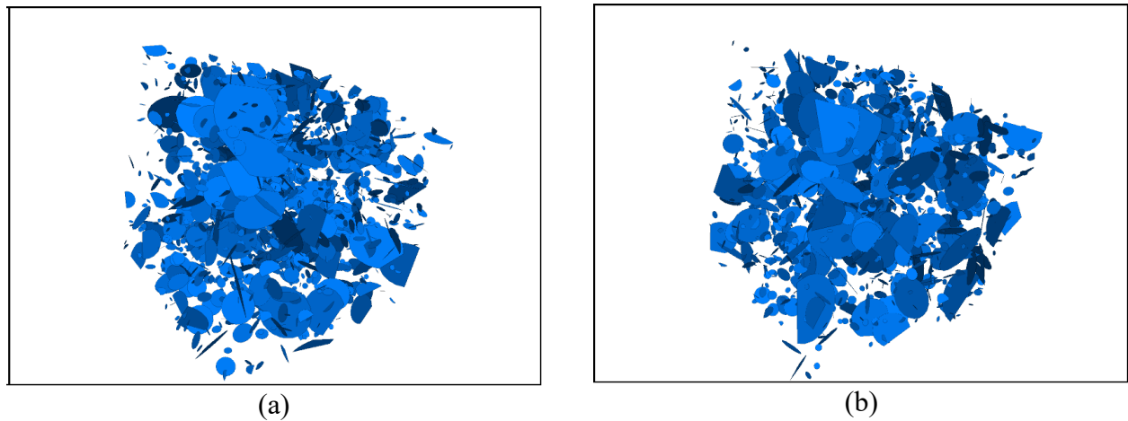
Figure 7-42 Stochastic DFN Case I dip angle rotated at (a) 0^\circ and (b) 90^\circ – boundary conditions Case II
