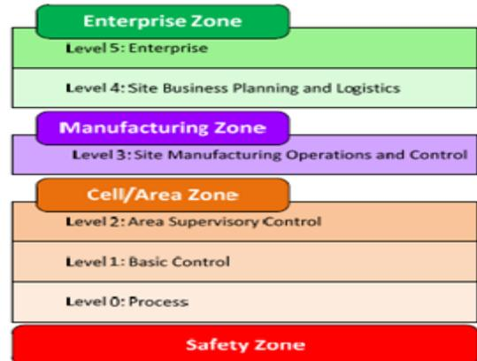
Fig. 2. Purdue Model for Control Hierarchy [14]
