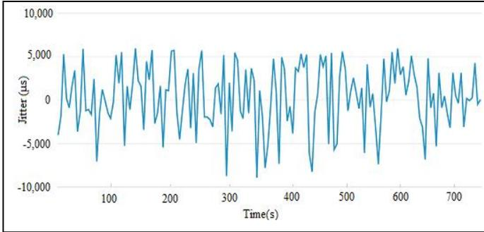
Fig. 5. Master to slave jitter when basic rules are configured.
