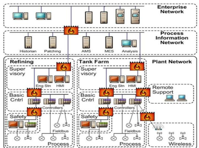
Fig. 1. An example of IACS segmentation using firewalls [6]
