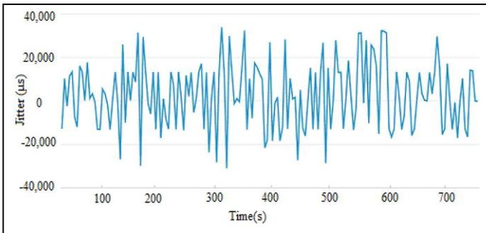
Fig. 6. Master to slave jitter when basic and Modbus rules are configured.
