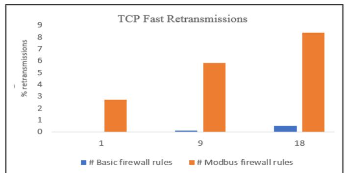
Fig. 7. Average TCP Fast Retransmissions in different filtering modes
