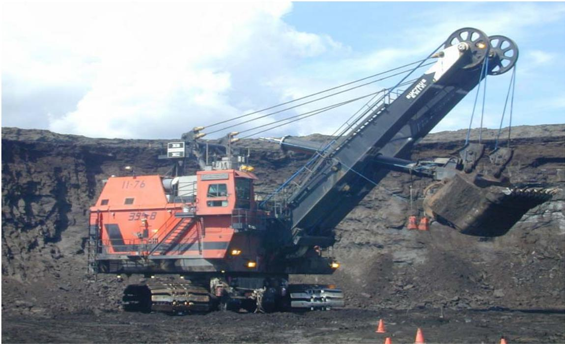
Fig. 2.1 Shovel digging and scooping oilsand at Syncrude
