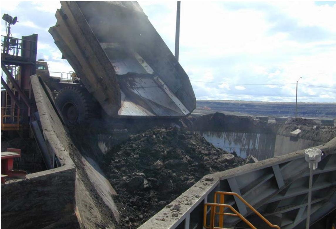
Fig. 2.6 A view of the diamond shaped hopper from top
