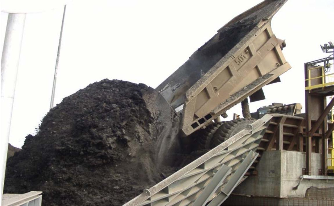
Fig. 2.3 Haul truck dumping oilsand into the crusher hopper (Aurora II, Syncrude)
