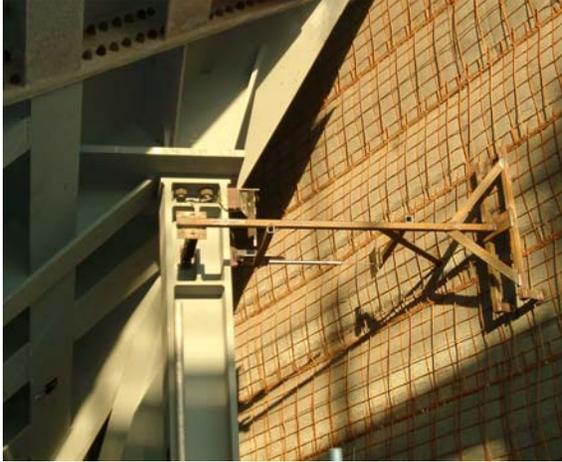
Fig. 3.17 LVDT set up at column top
