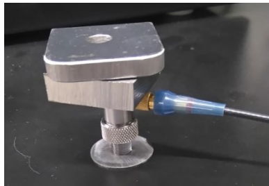
Figure 3.20 – Longitudinal wave probe V202-RM held steady with weight blocks on a disc sample of a Grade 483 Q&T end quench specimen.
