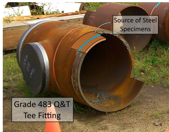
Figure 3.3 – Grade 483 Q&T Tee fittings at a testing facility, where sections were removed for this research project.
