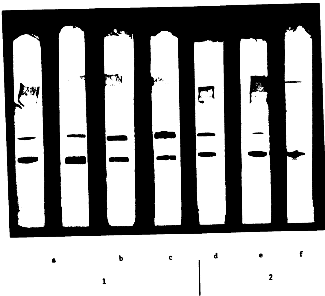
Fig. 8: Disc-gel electrophoresis at 9.5 in 8 M urea of SH-tropomyosin. Numbers 1 and 2 denote two different preparations.
