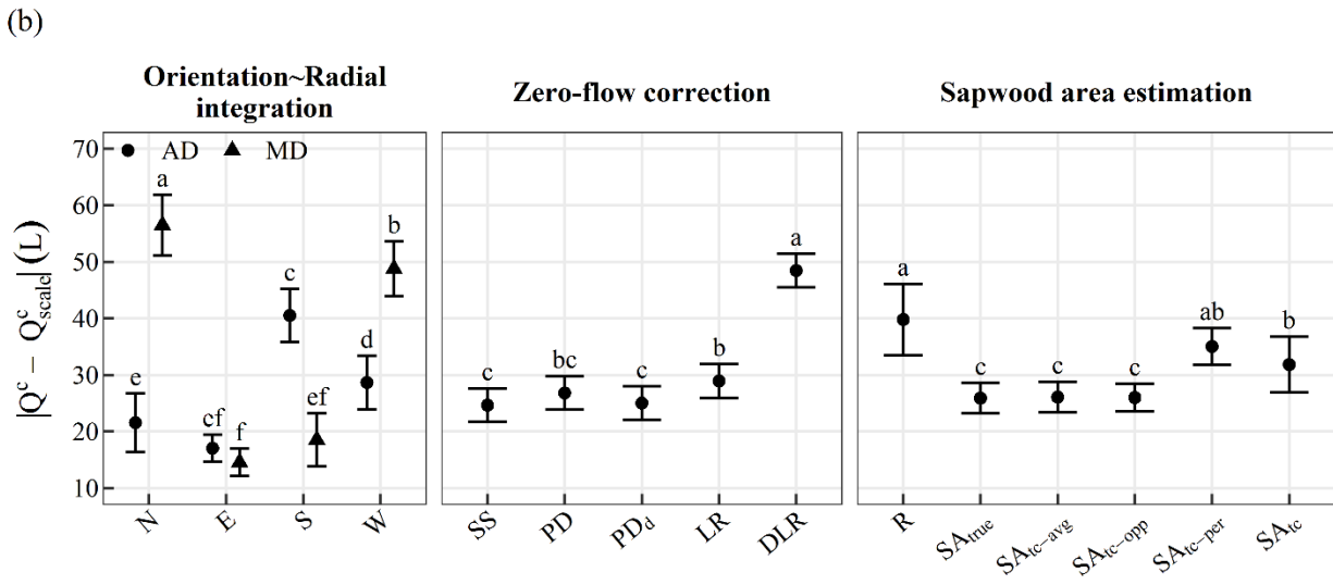
Figure 3. 4. Difference between sensor ( Q^c ) and gravimetric ( Q^c_{scale} ) estimates of cumulative water uptake over the five days after the cut for cardinal placement of the sap flow sensor and the three
