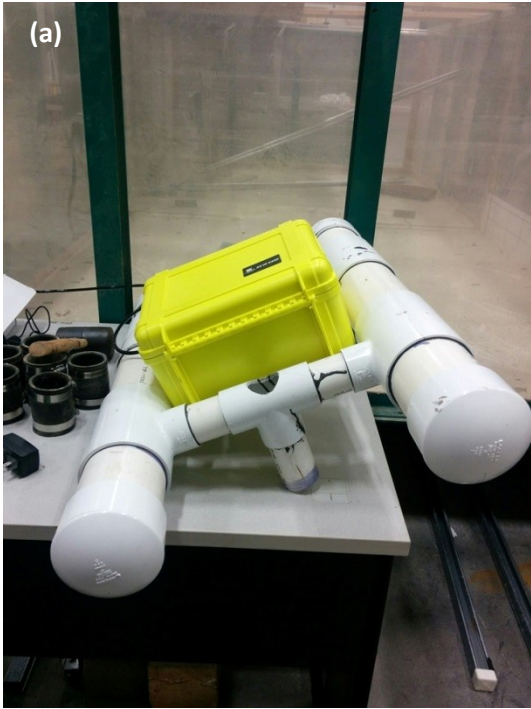
Figure 2.4: Floating platform (a) and anchors (b) for TDG probe deployment
