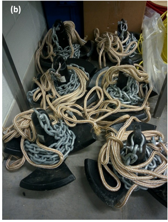
Figure 2.4: Floating platform (a) and anchors (b) for TDG probe deployment
