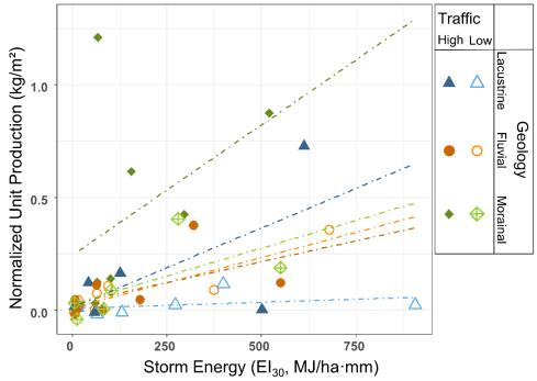
Figure 2-5. Sediment production rate versus storm energy by settling tank plot
