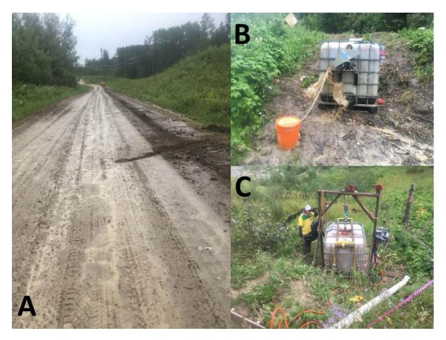
Figure 2-2. Settling tank plot components (A) open top wooden culverts draining a road segment, (B) tipping bucket mechanism, (C) weighing frame with battery-operated winch
