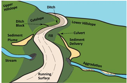
Figure 1-2. Theoretical road prism showing features of the road environment, connectivity pathways, and consequences for road erosion
