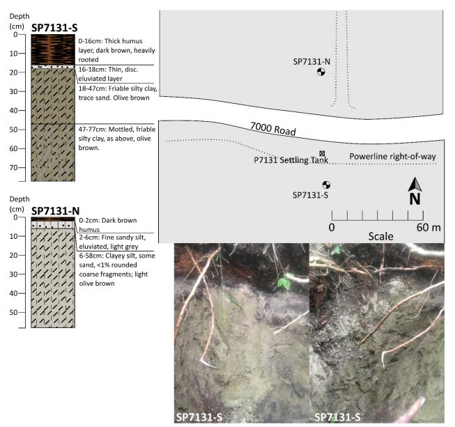
Figure A10. P7I3I site map with soil pits showing compact silty clay with a few coarse fragments. Olive-brown to greyish colours with mottling indicate site is imperfectly-drained. Thin eluviated horizons in both soil pits.
