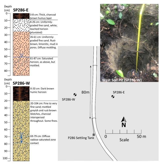
Figure A8. P286 site diagram and soil pits. This was the sandiest and best-drained site encountered in the study.
