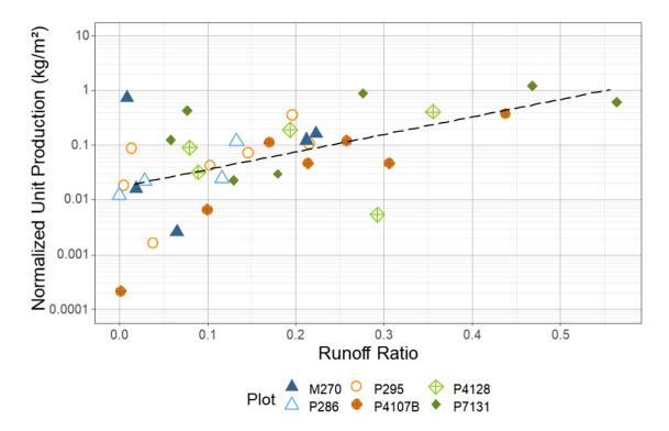
**Figure 2-7. Sediment yield compared with runoff efficiency for settling tank plots.** *Vertical scale is logarithmic. Note that sediment production generally increases with runoff ratio and rate of increase is non-linear.*
