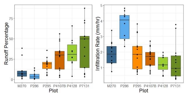
**Figure 2-6. Plot runoff-generating efficiency (left) and peak infiltration rate by plot (right)** *Plot colours represent traffic and surficial geology, with blue representing lacustrine sediment, orange fluvial sediment, and green morainal sediment, lighter shades represent low traffic, and darker shades high traffic.*
