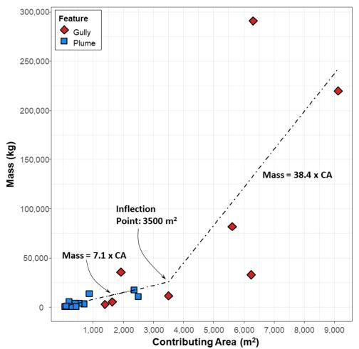
Figure 5-2. Erosion and contributing area relationships for measured sediment plumes (blue), and gullied ditch segments (red). Erosion increases rapidly for sections of road larger than 3500 m<sup>2</sup>
