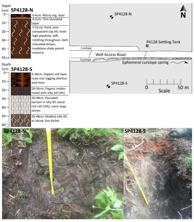
Figure A12. P4128 plot diagram and soil pits showing compact, silt and clay-rich morainal soil.
