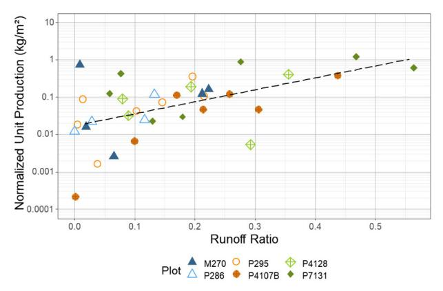
Figure 5-1. Normalized sediment production (logarithmic axis) versus plot runoff ratio for road plots in the Simonette
