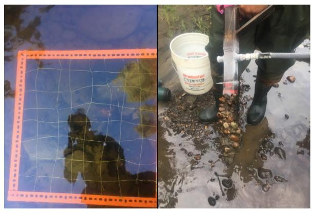
Figure 4-4. Stream physical sampling equipment: counting frame (left); metal freezecoring device with attached bed substrate material (right)
