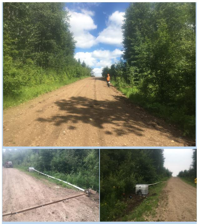
Figure A9. P286 site photograph showing well-gravelled sandy surface texture (top); bottom culvert and tank set-up (bottom left); tank set-up looking upslope (bottom right)
