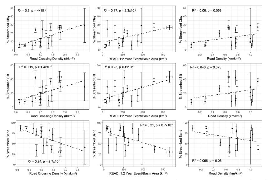
Figure 5-4. Gravel matrix composition compared to road crossing density (#/km), READI values, and road density (km/km<sup>2</sup>) from left to right. The most significant correlations are between road crossing density and gravel matrix composition, and the least are between road density and gravel matrix composition.
