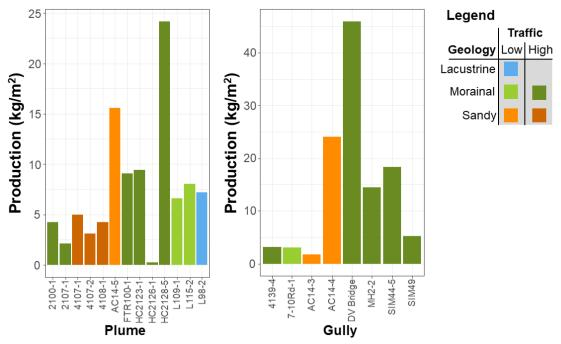
Figure 2-8. Comparison of erosion rates estimated from plume extent and thickness from non-gullied road segments (left), and gully surveys (right)
