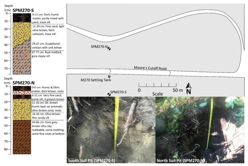
Figure A7. M270 site map and soil pits. This site had well-drained soil not overcompacted by glacial overriding.
