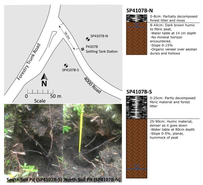
Figure A2. P4107B site map and soil pits. Soil pits show that the road was built out of imported sandy fill material used to cross a deep organic bog. Alternating bog and sand-hill deposits are common in aeolian terrain.
