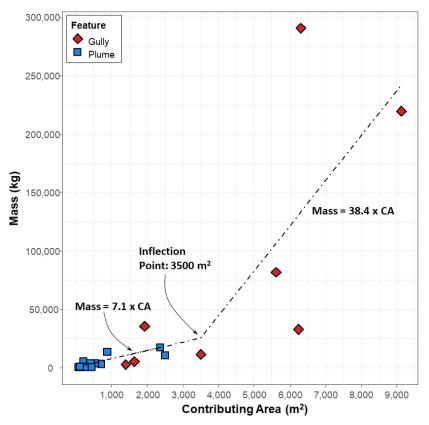
Figure 2-9. Relationship between contributing area and mass for plumes (blue) and gullies (red) showing threshold erosion behaviour for contributing areas greater than 3500 m<sup>2</sup>
