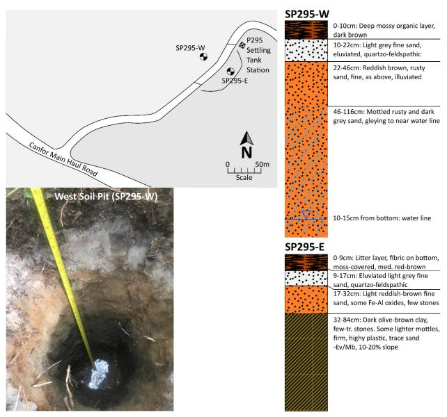
Figure A4. P295 site map and soil pits. Water table encountered at bottom of west soil pit. Thin, relatively well-drained sand over firm (compact) poorly-drained glacial clay.
