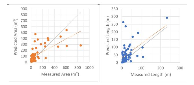
Figure 3-7. Predicted versus modelled values for plume area (left) and length (right) using parameter average values and the READI model. 1:1 line is plotted in grey. Values above the 1:1 line are over-predictions, and values below the line are under-predictions. Red dashed lines are the trend lines of the prediction.
