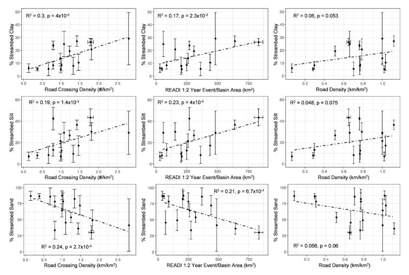
Figure 4-6. Relationship between streambed gravel matrix composition and road pressure variables, showing increased silt and clay percentage with higher road crossing density (#/km<sup>2</sup>) and READI indexed sediment loading per km<sup>2</sup> basin area. Road density does not significantly predict streambed gravel matrix composition.
