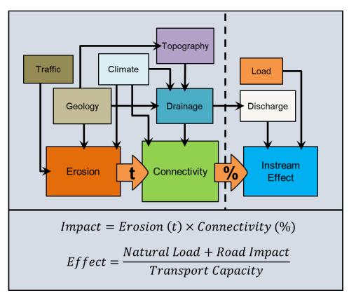
Figure 1-6. Conceptual model of point source impact to the stream environment.
