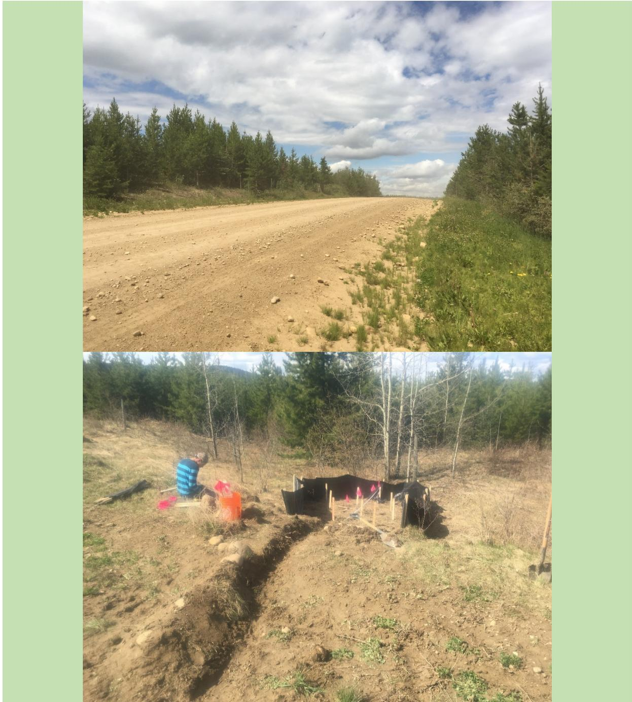
**Figure AI7. Site photos of P4126. Site was installed in a low-gradient (2.5°) segment of road (top), and a turnout berm was hand-excavated just up-gradient of a previous settling location with some sediment in it (bottom). Overall low slope and possible bypass may have compromised the ability of this plot to produce a meaningful sediment signature.**
