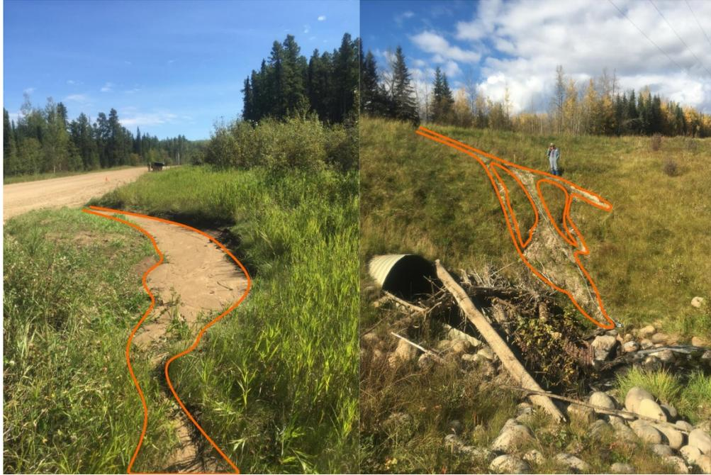
**Figure 1-4. Examples of road sediment plumes: a sediment plume filling a roadside turnout (left), and a large road sediment plume connected to a stream channel (right).**
