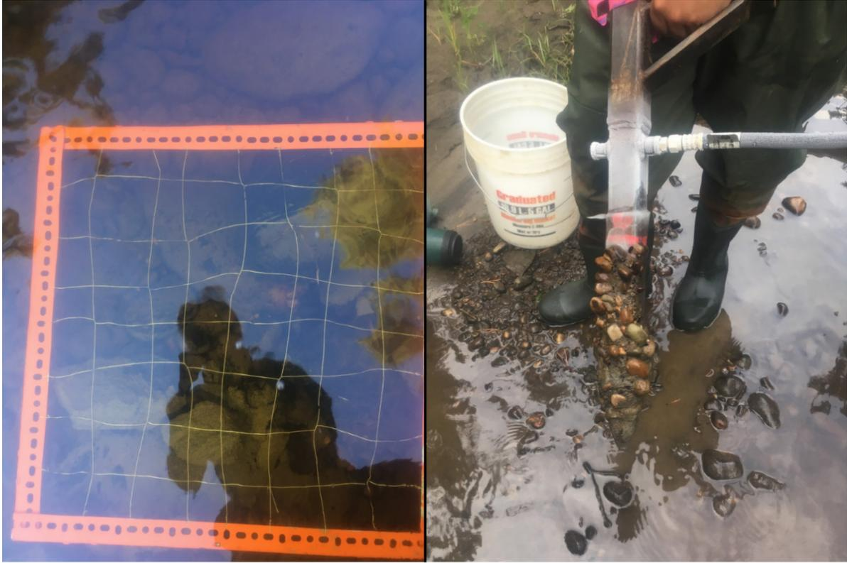
**Figure 4-4. Stream physical sampling equipment: counting frame (left); metal freezing device with attached bed substrate material (right)**
