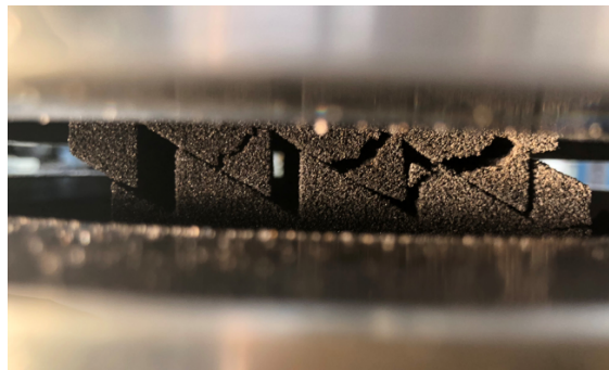
Figure 4.10. Cracking near the tips of triangular teeth in profile 3 during shearing.
