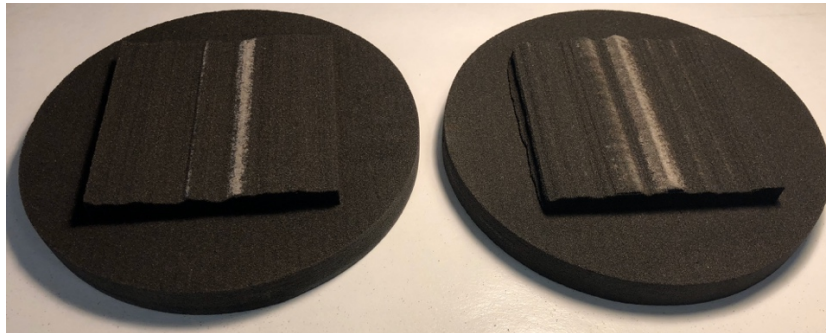
Figure A.4. Failure patterns after shear in NCJ-10-1: a. CNL conditions b. CNS conditions.
