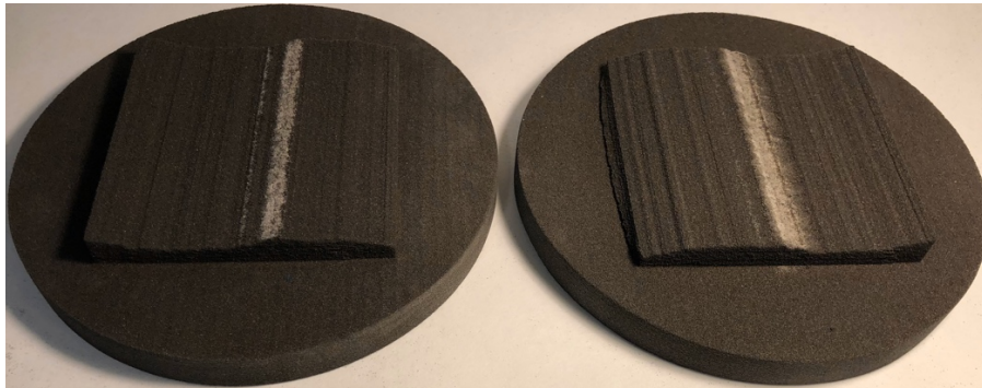
Figure A.8. Failure patterns after shear in NCJ-10-5: a. CNL conditions b. CNS conditions.
