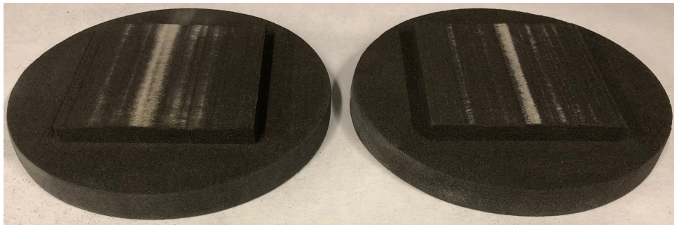
Figure A.3. Failure patterns after shear in NCJ-4-3: a. CNL conditions b. CNS conditions.
