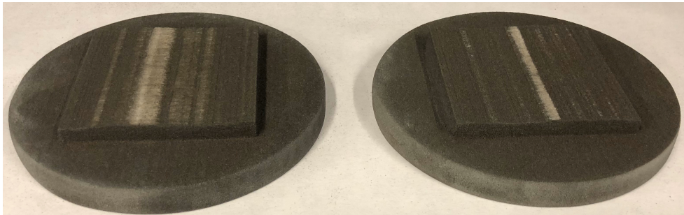
Figure A.2. Failure patterns after shear in NCJ-4-2: a. CNL conditions b. CNS conditions.
