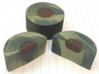
Figure 3.10. Infiltration of the printed disks with epoxy resin. The green part is where the dyed epoxy resin has infiltrated the specimen. The gray part is not yet infiltrated.
