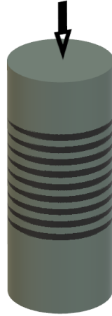
Figure 3.3. Schematic illustration of a cylindrical printed sample showing the orientation of the layers.
