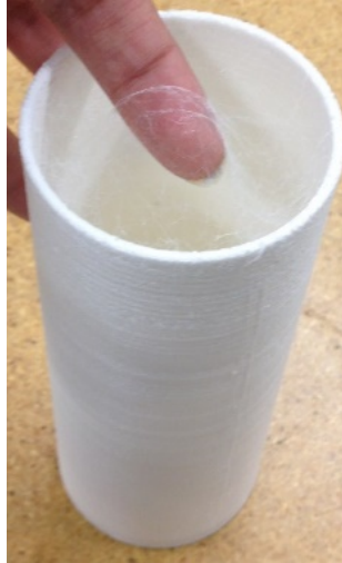
Figure 3.33. Stringy print encountered when printing with the Flexystruder printhead.
