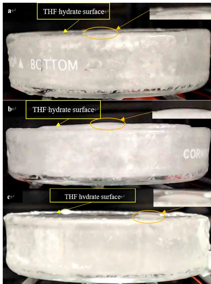
Figure 3-5 Typical droplet of testing liquids on a THF hydrate surface.
