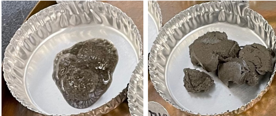
Figure 4-14: Flocculated MFT without predilution (HPAM4 = 1500 ppm, PVBTMAC = 3500 ppm). Left: Before filtration. Right: After filtration.
