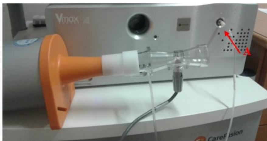
Figure 5. Vmax sample line is now connected to the calibration port (A) as shown by the arrow indicating the connection point.
