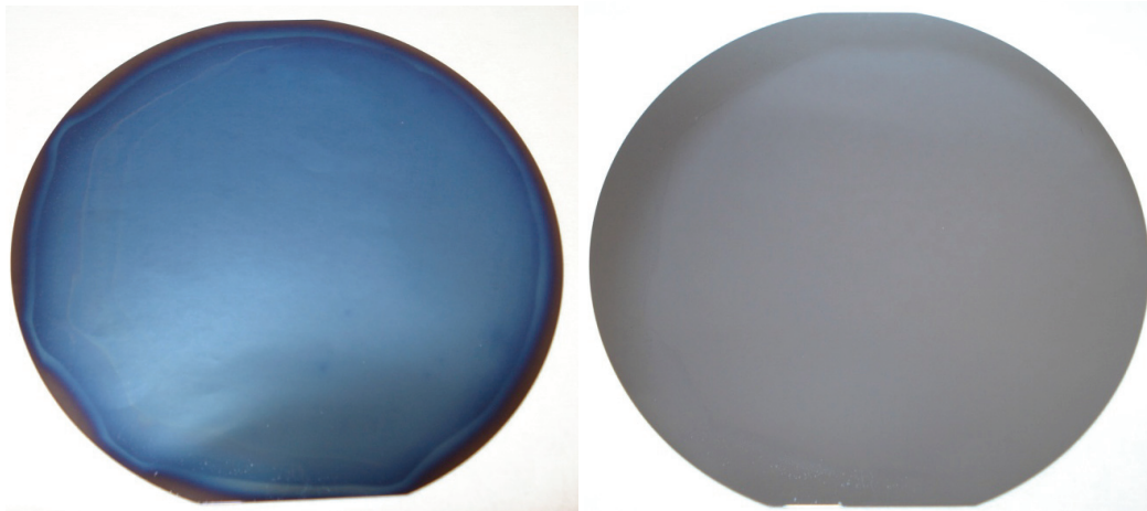
Figure 3.17. A substrate is shown after the diffusion doping and drive-in procedure. The left image shows the substrate before the BOE process, the right image is after the BOE.
