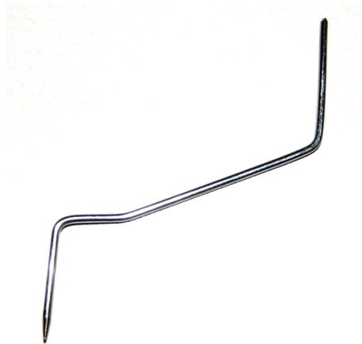
Figure 4.13. Force application probe constructed of 1.5875mm diameter stainless steel rod.
